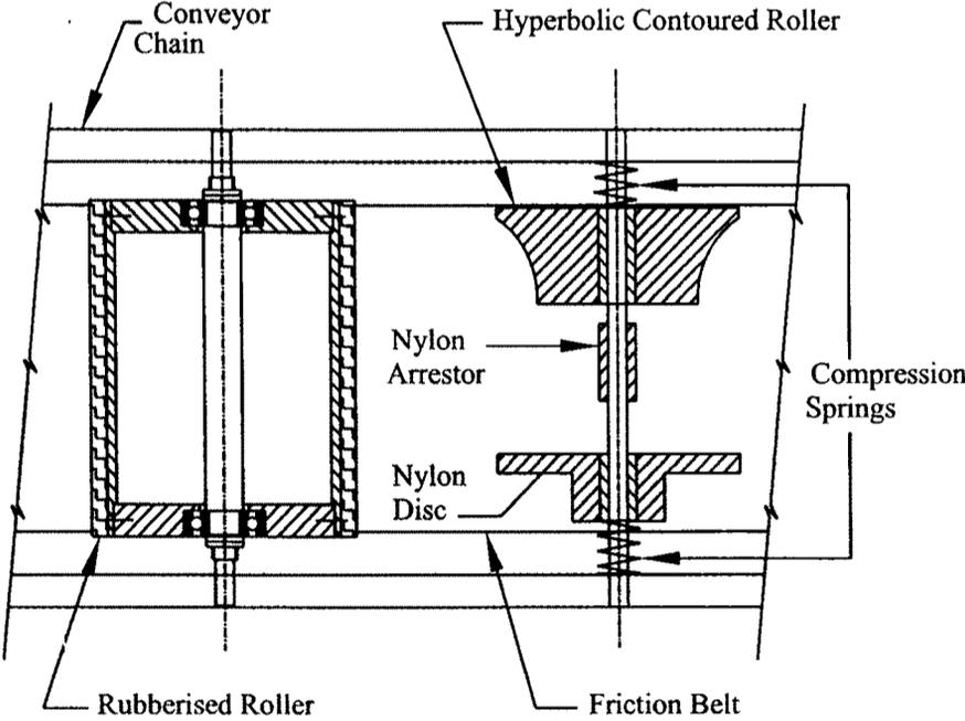
Figure 2.9 Apple Orienting Rollers Assembly
