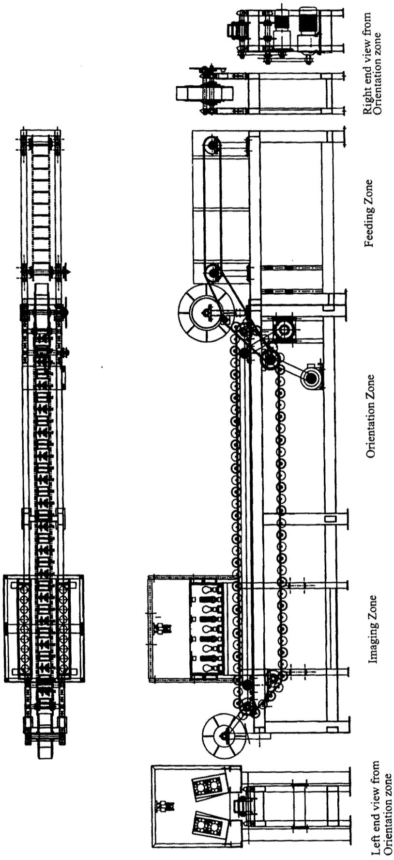
Figure 2.6 Mechanical Assembly of Fruit Feeding, Orienting and Conveying Sections
