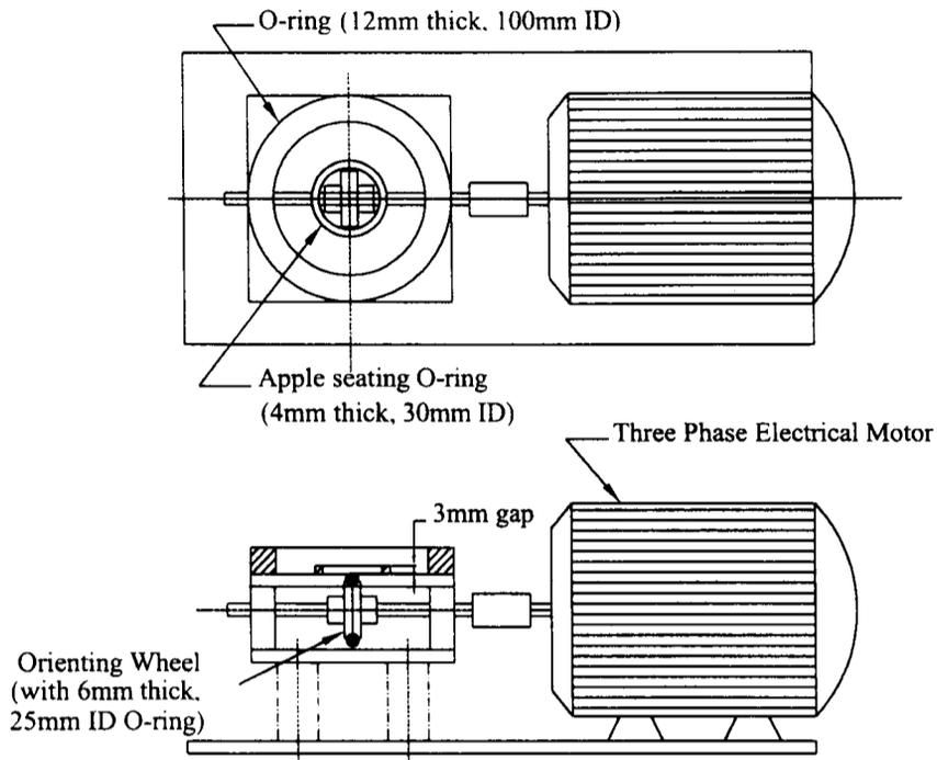
Figure 2.1 Vertical Orientation Unit
