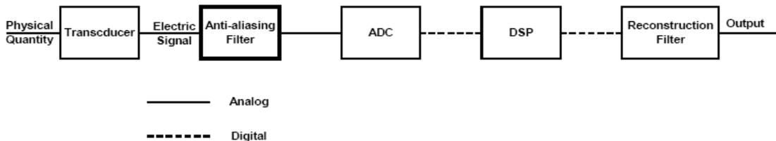
**Figure 1.1 A Typical DSP System**
