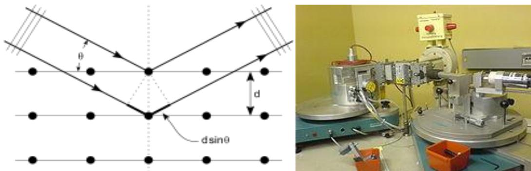
Fig. 2.4.1. Bragg's equation diagram and X-Ray Spectrometer
