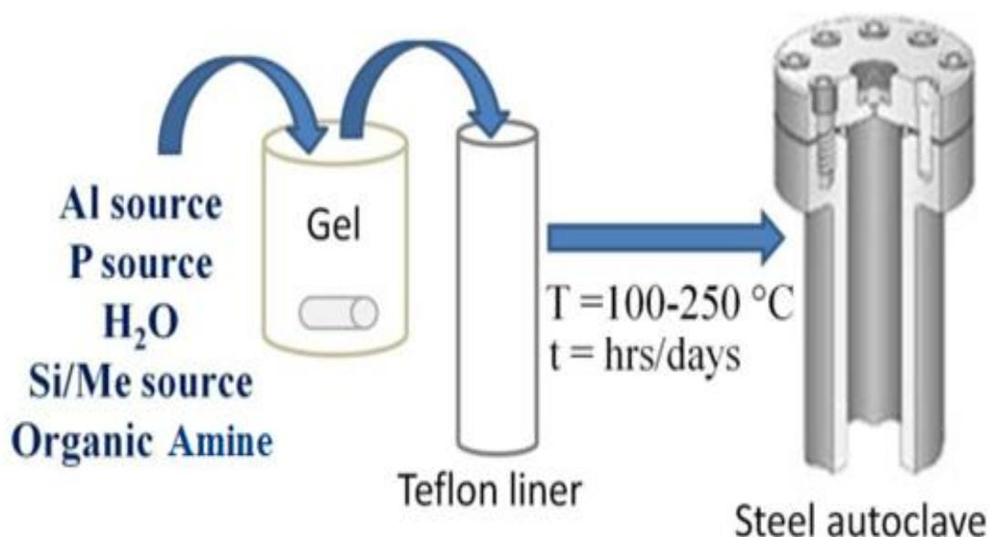
Fig. 2.2.4. Graphical representation of synthesis steps
