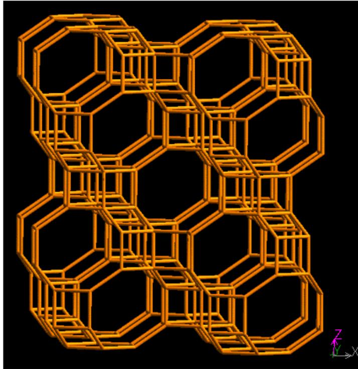
Fig. 2.1.2. 3D framework structure and channel system of SAPO-5 aluminophosphate
