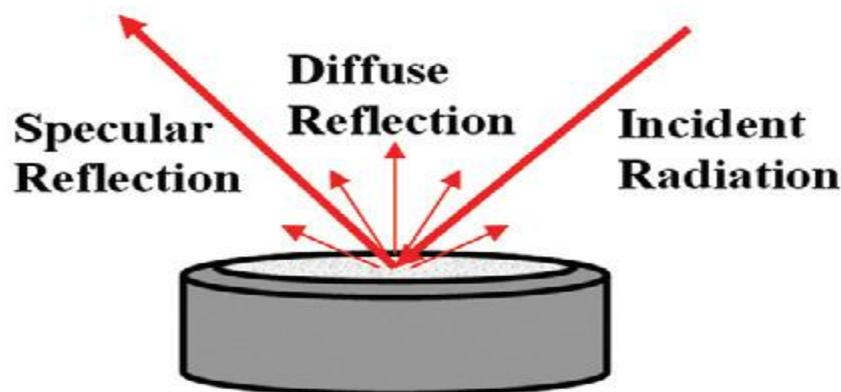
Fig. 2.4.4. Principle of diffuse reflectance
