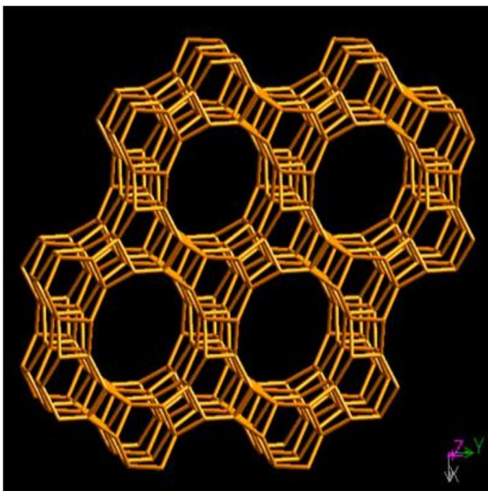
Fig. 2.1.1. 3D framework structure and channel system of AIPO-5 aluminophosphate
