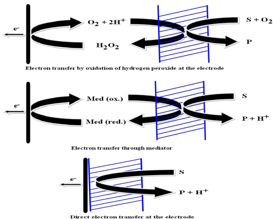
**Fig. 7.** Mechanism of electron transfer in amperometric biosensing system
