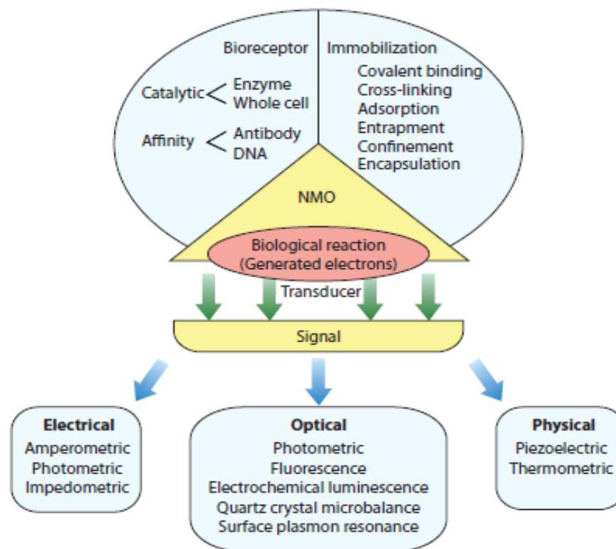
**Fig. 6.** Various types of transducers for biosensing
