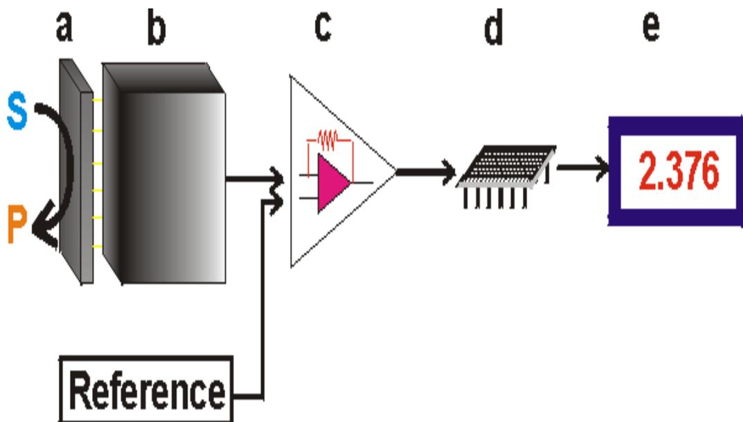
**Fig. 5.** Schematic diagram showing the main components of a biosensor. The biocatalyst (a) converts the substrate to product. This reaction is determined by the transducer (b) which converts it to a signal. The output from the transducer is amplified (c), processed (d) and displayed (e). (Reproduced with permission from Mart Chaplin, <http://www.isbu.ac.uk/biology/enztech/biosensors>)
