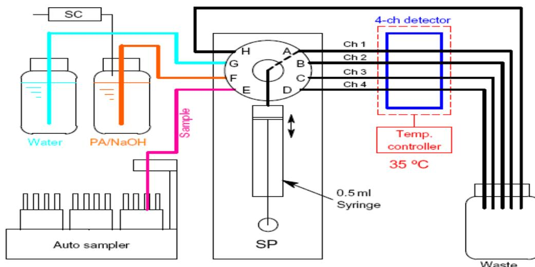
**Fig. 2.** Zone fluidics based creatinine analyzer (Source: Ohira *et al.*, 2009)
