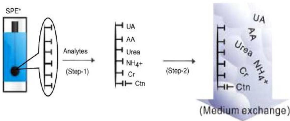
**Fig. 9.** Conceptual representation for the selective recognition of creatinine (Ctn) in presence of uric acid (UA), ascorbic acid (AA), urea, ammonium chloride (NH<sub>4</sub><sup>+</sup>) and creatine (Cr) at the SPE. Step-1: preconcentration of SPE at 1.8V vs. Ag/AgCl. Step-2: medium exchange of the SPE where the preconcentrated electrode is submerged in water. (Source: Chen *et al.*, 2006)
