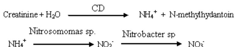
The reacting bacteria consume oxygen, so that the oxygen decrease may be detected by an oxygen electrode.
