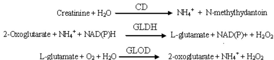
Ammonia produced by the enzymatic hydrolysis of creatinine was converted to glutamate, and the oxygen consumption due to the oxidation of glutamate by GLOD was detected with an oxygen electrode. **Table 2** provides a comparison of analytical properties of DO metric creatinine biosensors
