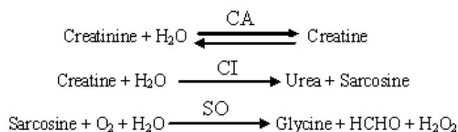
The reaction of creatinine in reaction 1 leads to oxygen consumption in reaction 3.
