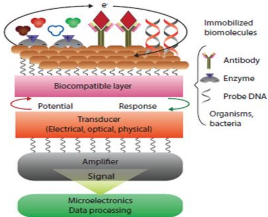
**Fig. 4.** Elements and selected components of a typical biosensor Schematic structure and operating principle of a biosensor
