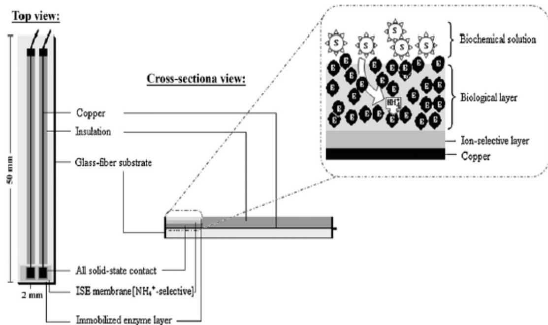
**Fig. 8.** Schematic diagram of the conductometric creatinine biosensor (Source: Isiladak *et al.*, 2012)
