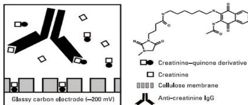
**Fig. 10.** Principle of size exclusion redox-labeled immunoassay (Source: Benkert *et al.*, 2000b)
