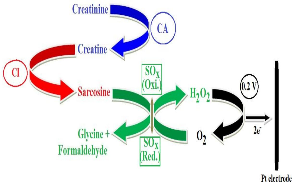
**Fig. 25.** Flow of electrons in present creatinine biosensor based on of Enzymes/c-MWCNT/PANI/Pt electrode
