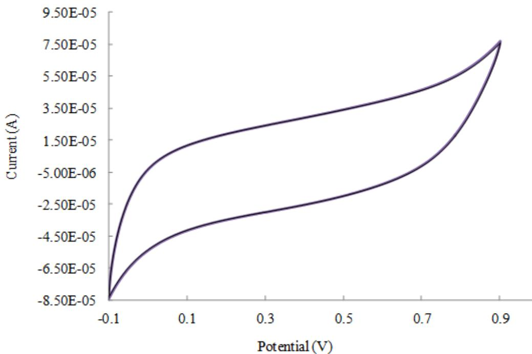
**Fig. 24.** Cyclic voltammogram of Enzymes/c-MWCNT/PANI/Pt electrode in 0.05 M PB (pH 7.5) at 100  $\mu\text{M}$  creatinine solution
