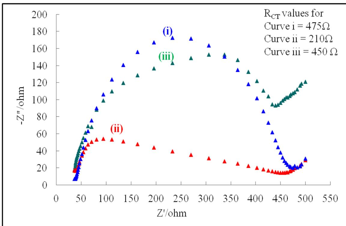
**Fig. 23.** Nyquist plot of electrochemical impedance spectra for PANI/Pt electrode (curve i), c-MWCNT/PANI/Pt electrode (curve ii) and Enzymes/c-MWCNT/PANI/Pt electrode (curve iii) in 0.05 M PB (pH 7.5) containing 5 mM  $K_3Fe(CN)_6/K_4Fe(CN)_6$  (1:1) as a redox probe
