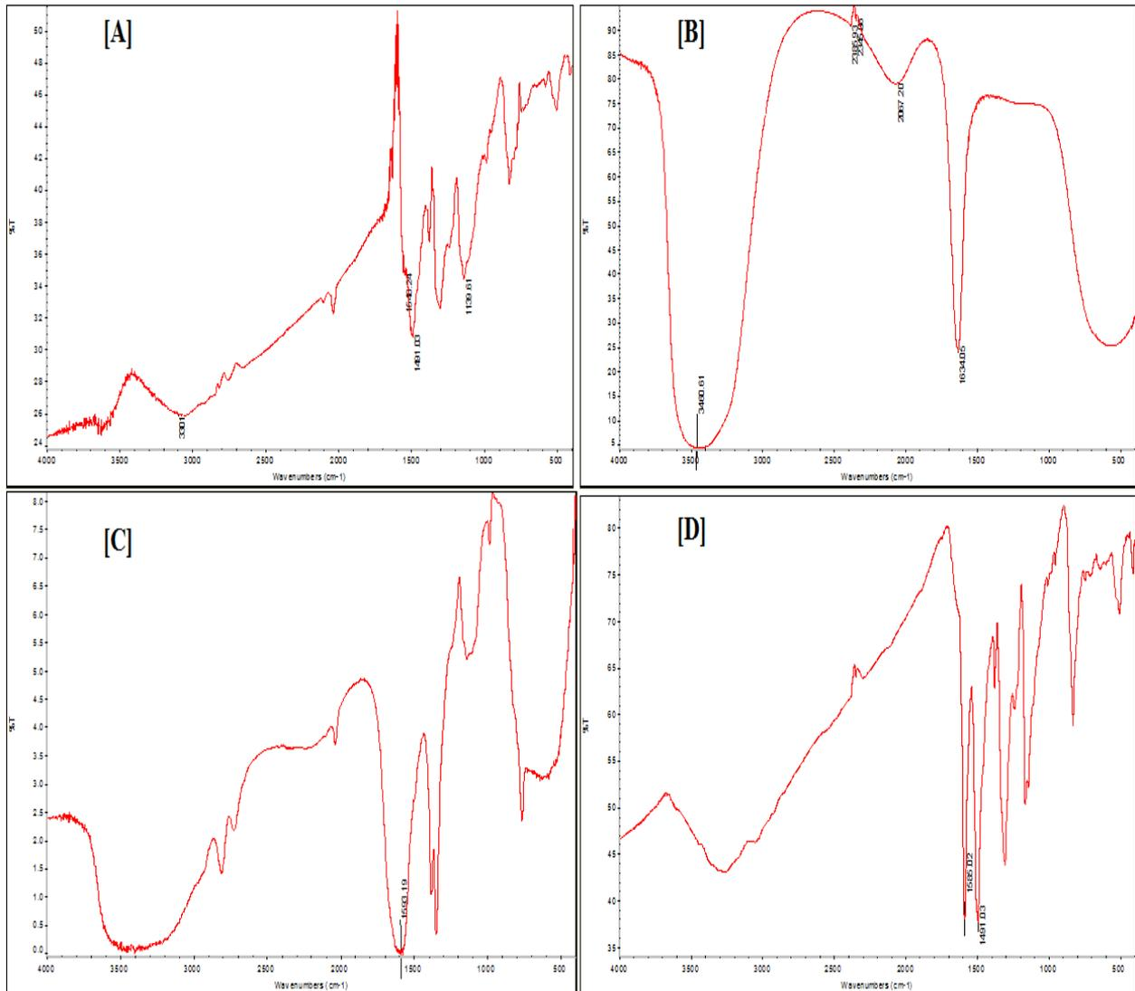
**Fig. 22.** FTIR spectra for pure PANI film [A] c-MWCNTs [B] c-MWCNT/PANI composite [C] Enzymes/c-MWCNT/PANI composite
