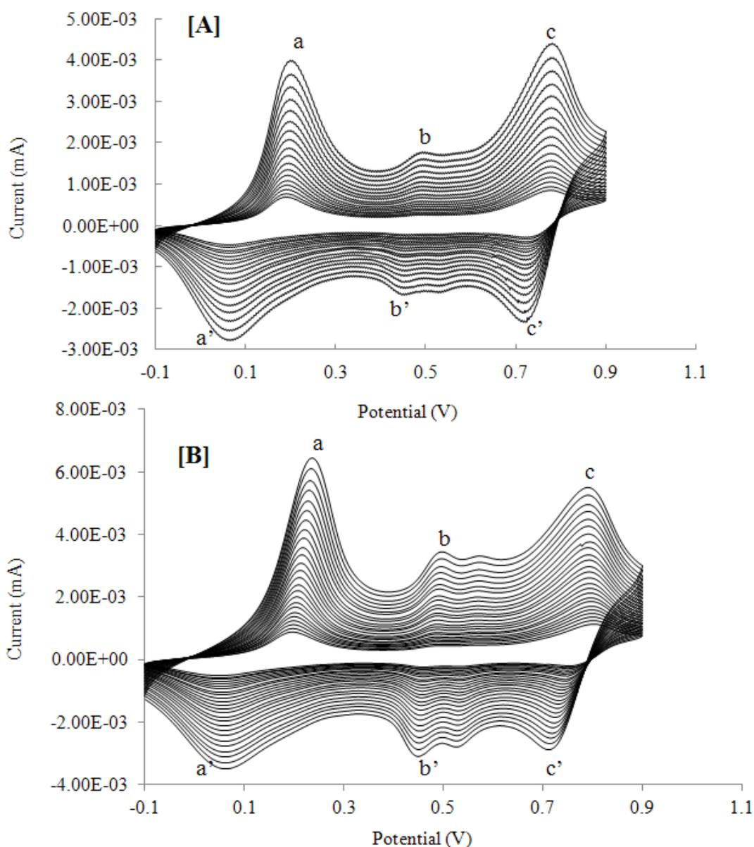
**Fig. 18.** Cyclic voltammograms for electrochemical deposition of PANI film [A] and c-MWCNT/PANI composite film [B] onto surface Pt electrode. Supporting electrolyte: 1N HCl solution; scan rate: 50 mV/s.
