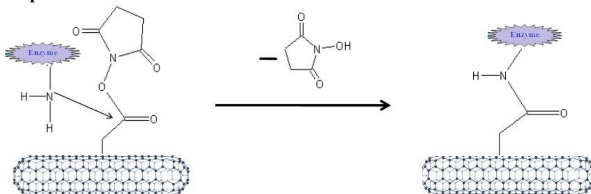
**Fig. 19.** Different steps involved in the immobilization of enzymes on to c-MWCNT/PANI composite film
