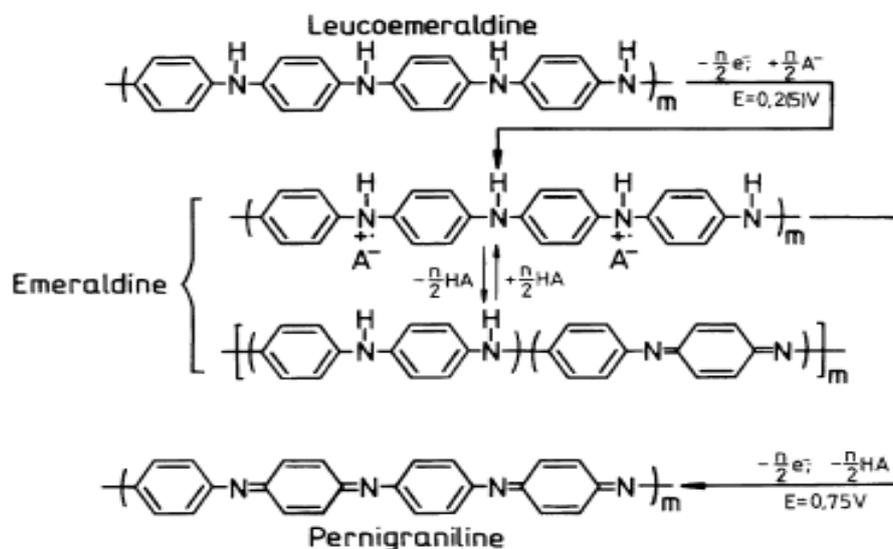
**Fig. 17.** Generalized scheme of the oxidative and non-oxidative (protonic acid) doping of PANI:  $n$ , number of aniline units,  $m = 4n$  (Source: Gospodinova and Terlemezyan, 1998)
