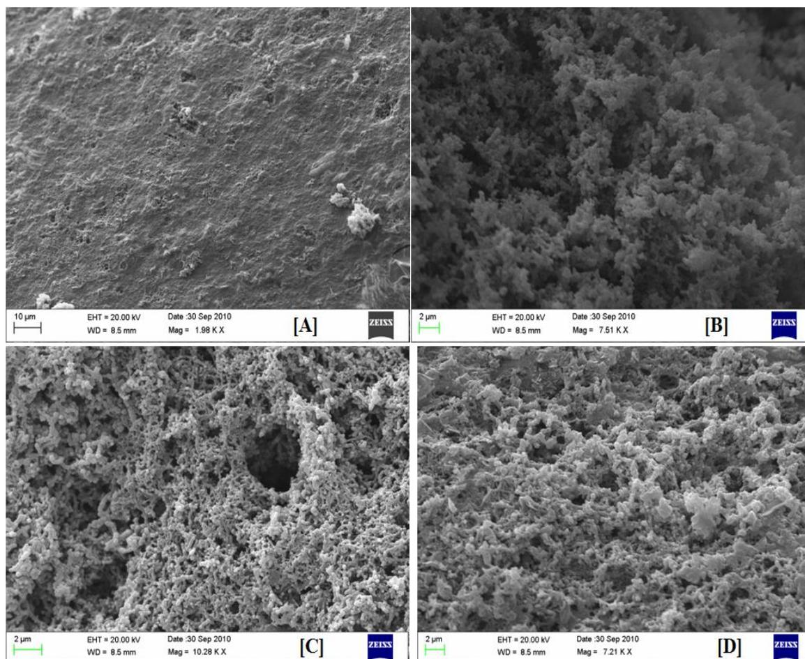
**Fig. 21.** Scanning electron microscopy of bare Pt electrode [A] PANI film [B] c-MWCNT/PANI composite film [C] immobilized enzymes onto c-MWCNT/PANI composite film deposited on Pt electrode
