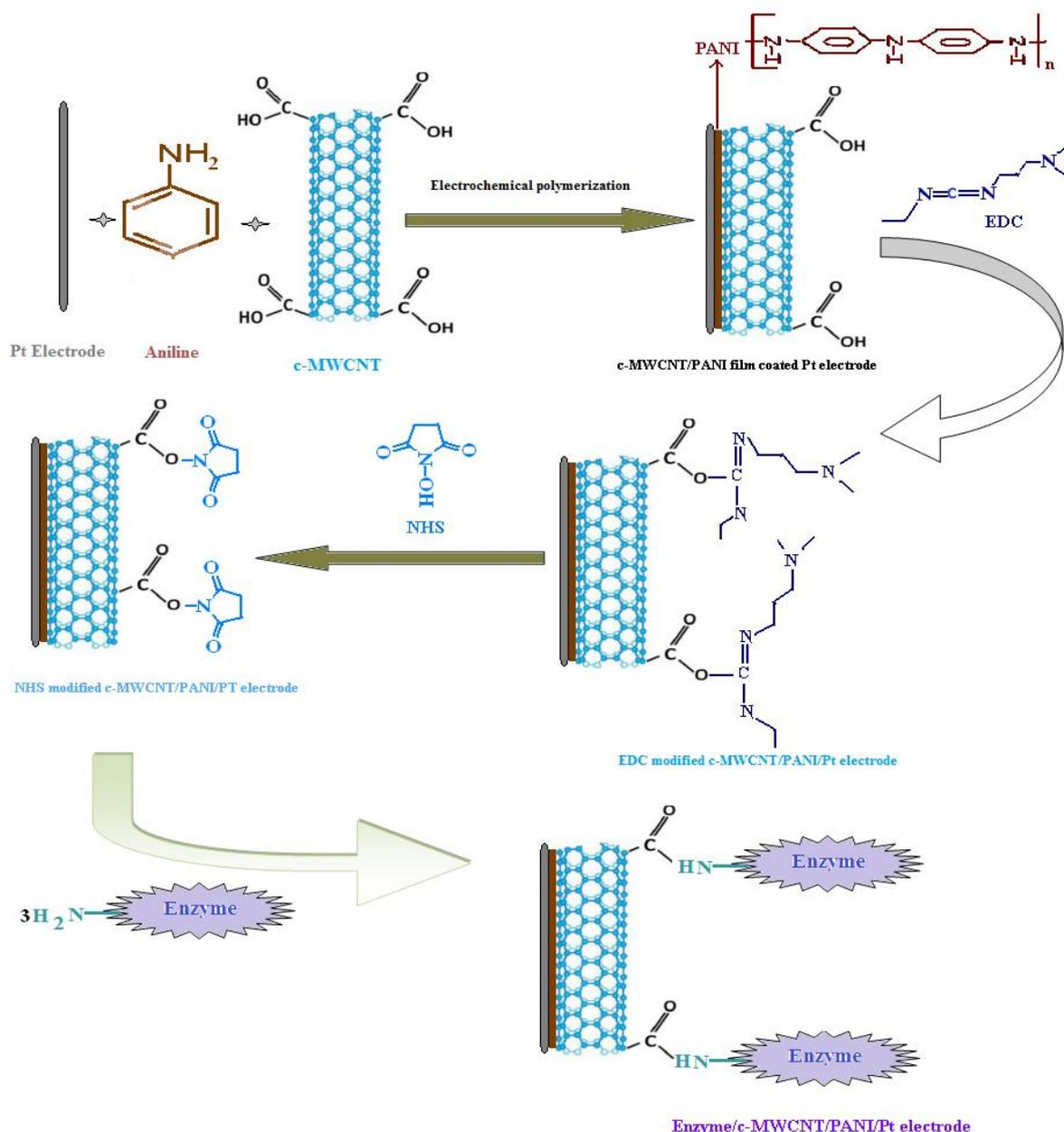
**Fig. 18.** Schematic representation of chemical reaction involved in the fabrication of Enzymes/c-MWCNT/PANI/Pt hybrid electrode
