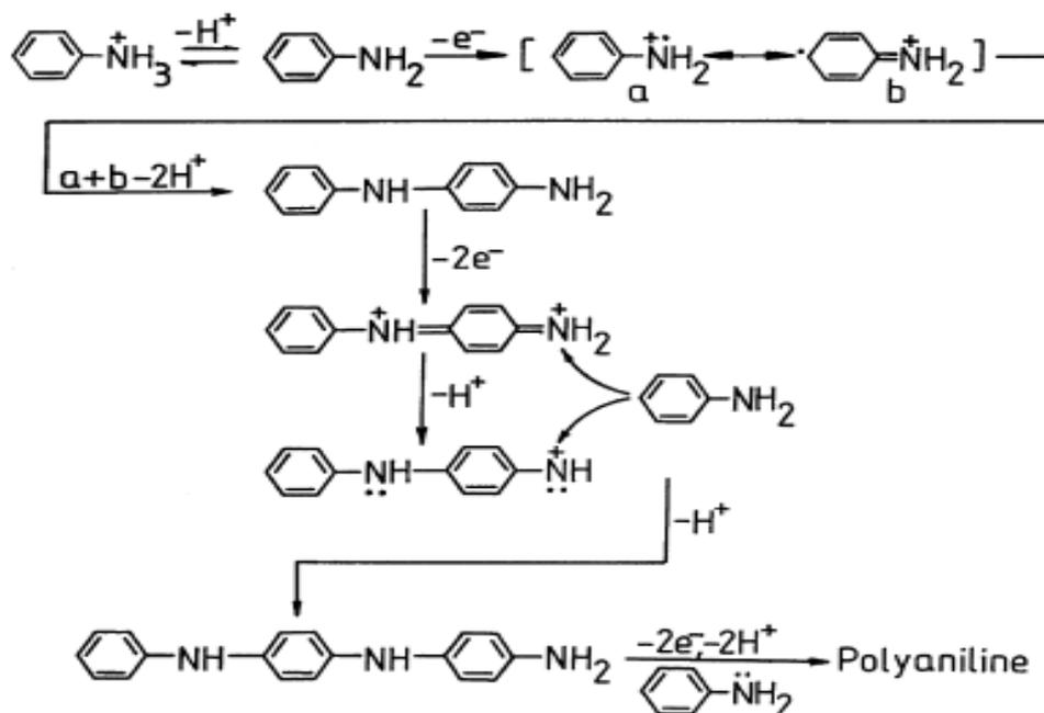
**Fig. 16.** Mechanism of the polymerization of aniline (Source: Wei *et al.*, 1989; 1990a,b)
