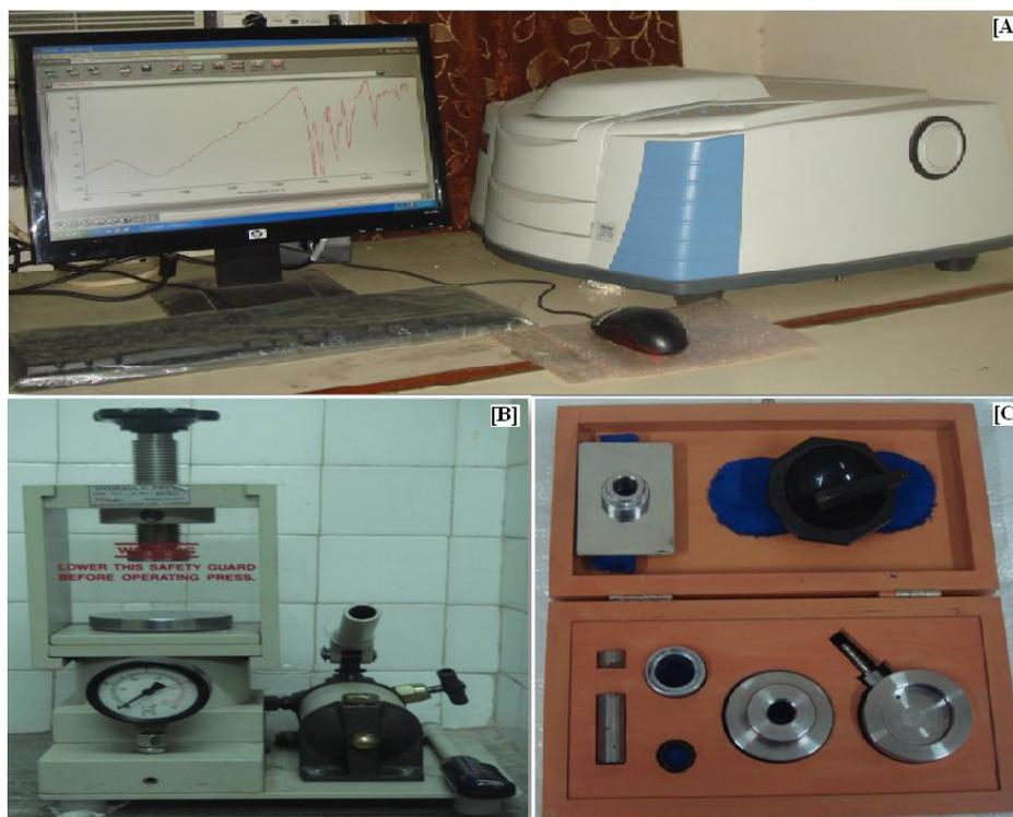
**Fig. 13.** FTIR spectrophotometer [A] Hydraulic press [B] Dye set for pellet preparation along with pellet holding socket [C]
