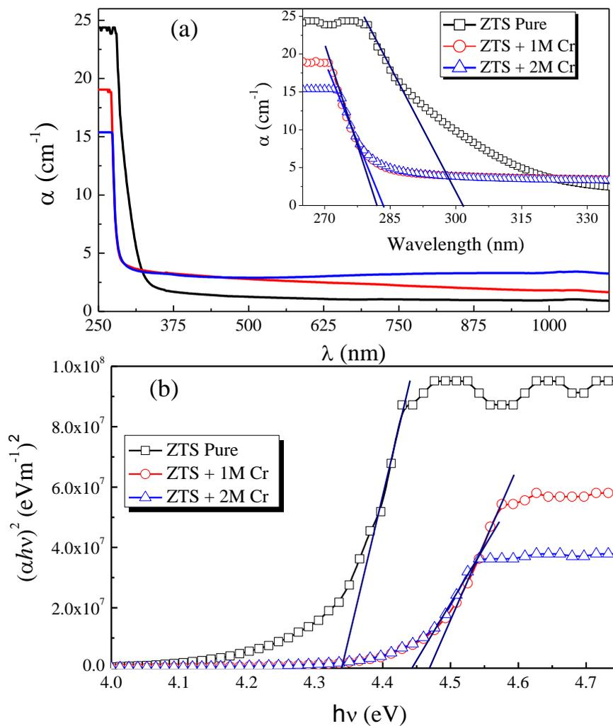
**Fig. 8.7:** (a) the absorption spectra, the inset indicates blue shift of absorption edge. (b) shows the increase in band gap of doped single crystals
