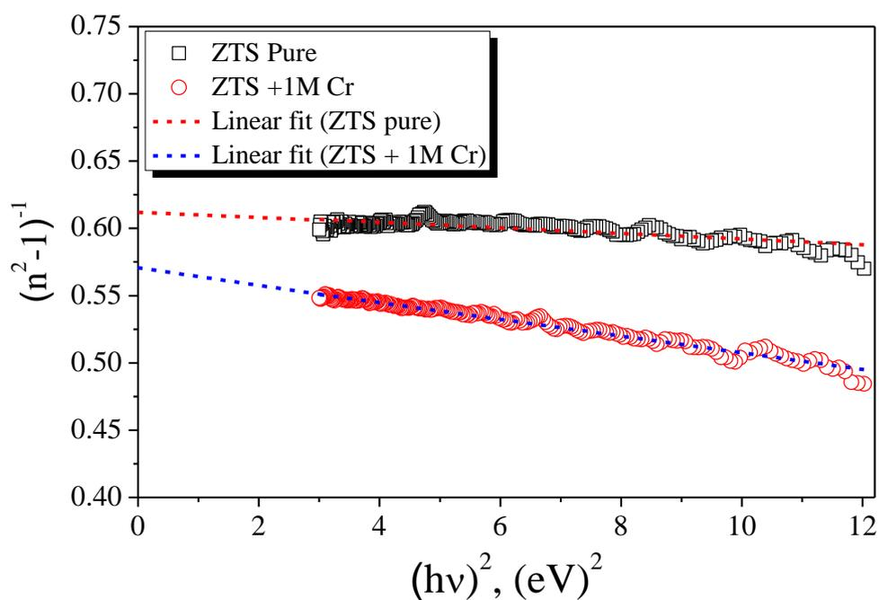
**Fig. 8.10:** The  $(n^2 - 1)^{-1}$  vs.  $hv^2$  plots for pure and 1 mol% doped ZTS single crystals. The dashed straight lines are the linear fit of the data points
