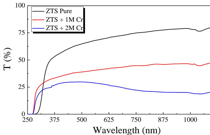
**Fig. 8.6:** The optical transparency spectra for pure, 1 mol%, and 2 mol% Cr-doped ZTS crystals
