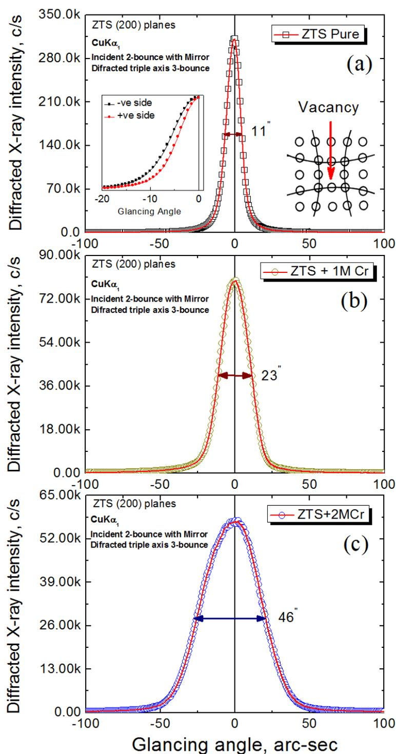
**Fig. 8.3:** The high resolution X-ray Diffraction curves recorded for (200) diffraction planes of (a) pure, (b) 1 mol% and (c) 2 mol%  $Cr^{3+}$  doped ZTS single crystals
