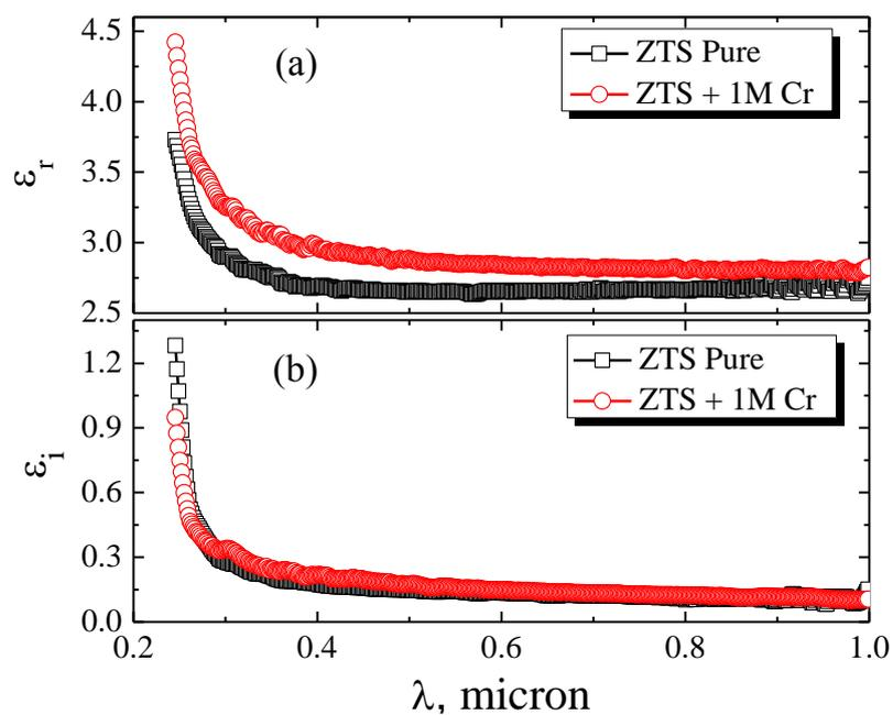
**Fig. 8.9:** (a) Real and (b) imaginary optical dielectric constants of pure and 1 mol% Cr-doped ZTS single crystals
