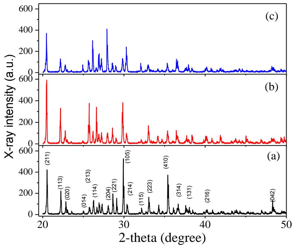
**Fig. 8.2:** The PXRD spectra of (a) pure and (b) 1 mol% and (c) 2 mol%  $Cr^{3+}$  doped ZTS crystals
