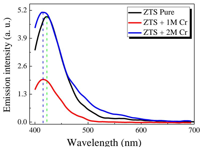
**Fig. 8.5:** The photoluminescence emission spectra for pure, 1 mol% and 2 mol% Cr-doped ZTS single crystals
