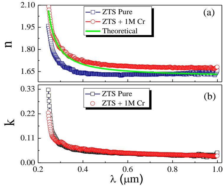
**Fig. 8.8:** (a) The linear refractive index and (b) the extinction coefficient of pure and 1 mol% Cr-doped ZTS single crystals
