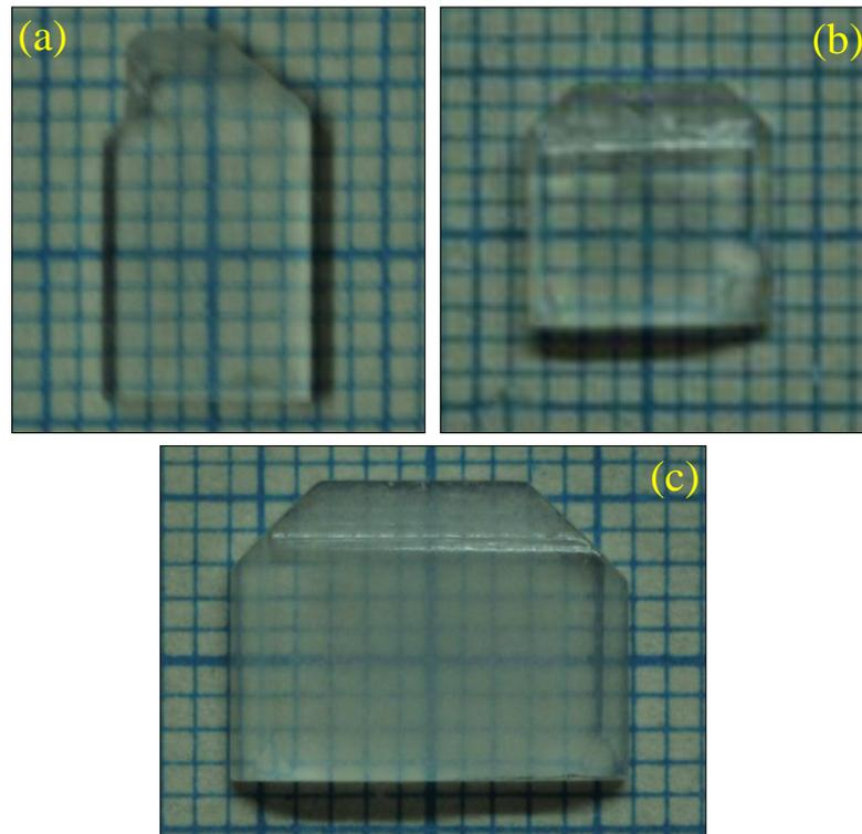
**Fig. 8.1:** The photographs of SEST grown (a) pure, (b) 1 mol% and (c) 2 mol% Cr doped ZTS single crystals
