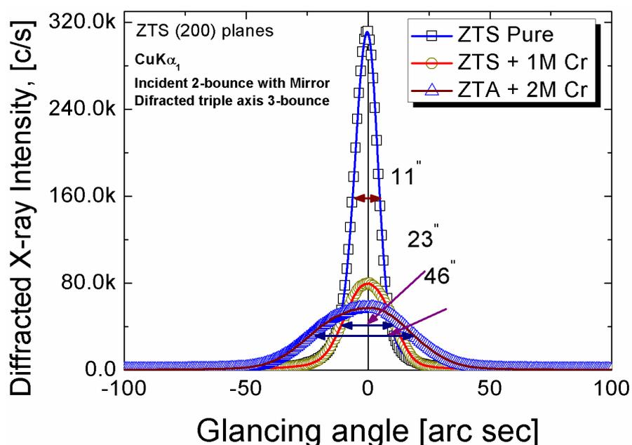
**Fig. 8.4:** The high resolution X-ray Diffraction curves of the pure and doped ZTS single crystals (Fig. 7.3) plotted on a common scale of glancing angle
