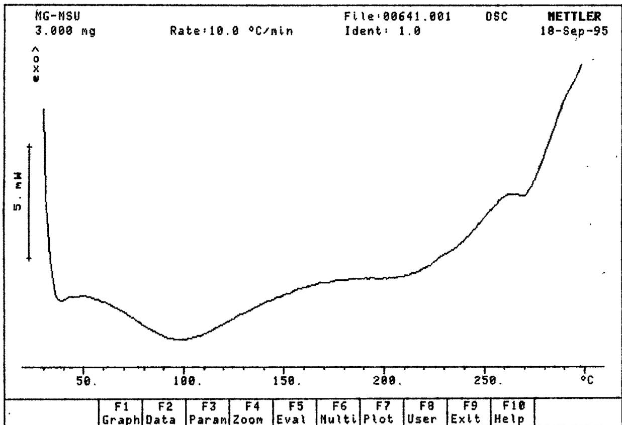
The products were also characterised by thermal analysis (Differential Scanning Calorimetry). A shift on the higher side of the endothermic peak of MGGs compared to the GG was observed (Fig 4.6).
