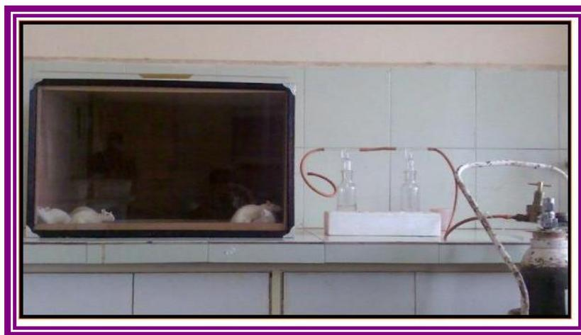
**Figure 12:  $\text{CCl}_4$  Vapour Induction Chamber**
