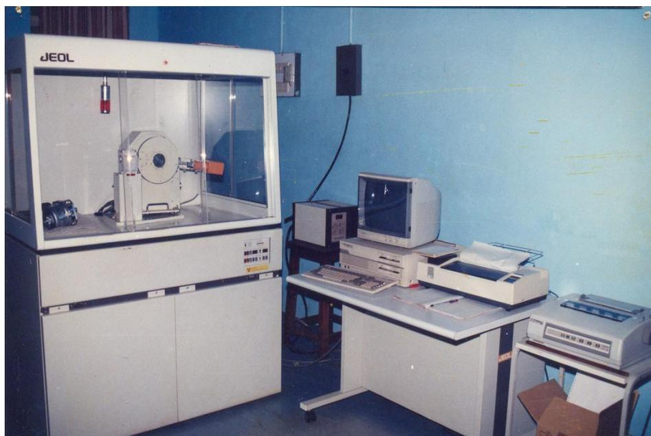
**Fig.3.3 Photograph of X-Ray Diffractometer**
