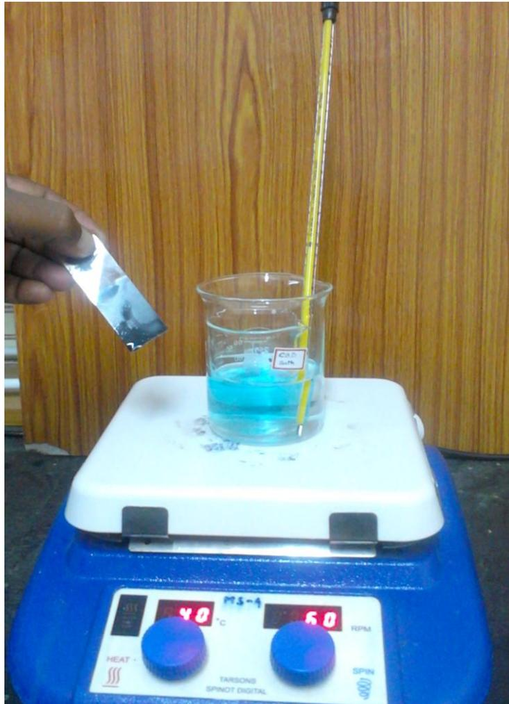
**Fig.3.1** Experimental set up for the preparation of metal oxide thin films
