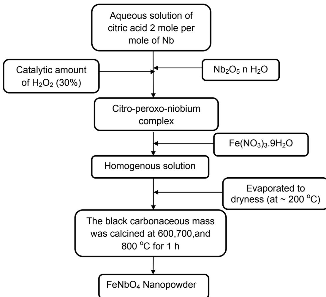
**Fig. 3.6. Flow chart for preparation of FeNbO<sub>4</sub> nanopowder by niobium-citrate complex process**
