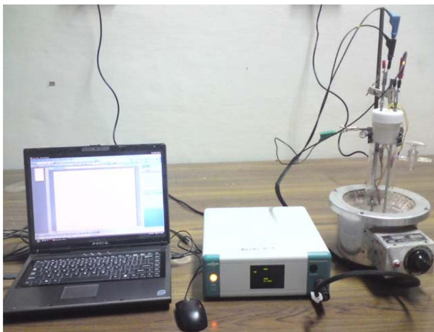
**Fig. 3.18. Photograph of Potentiostat /Galvanostat (Model: Micro auto lab type III) for electrical conductivity measurement**
