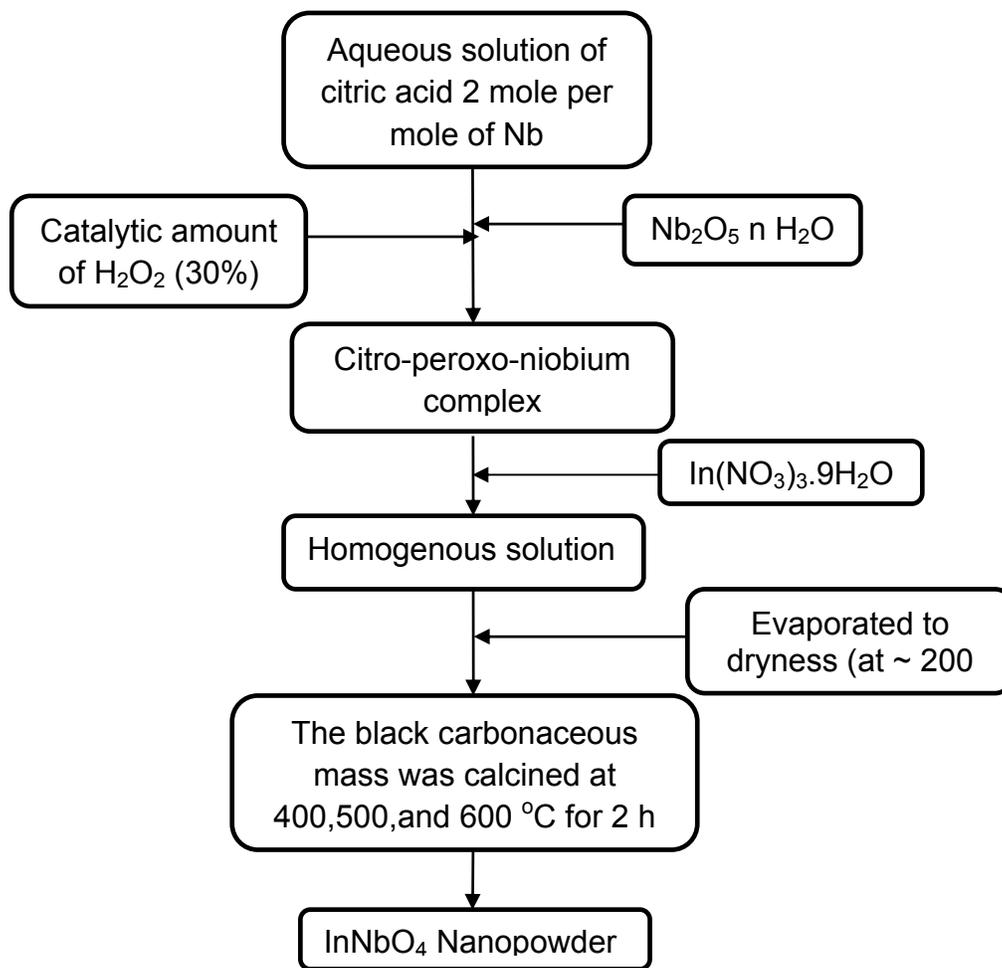
**Fig. 3.2. Flow chart for preparation of InNbO<sub>4</sub> nanopowder by niobium-citrate complex process**
