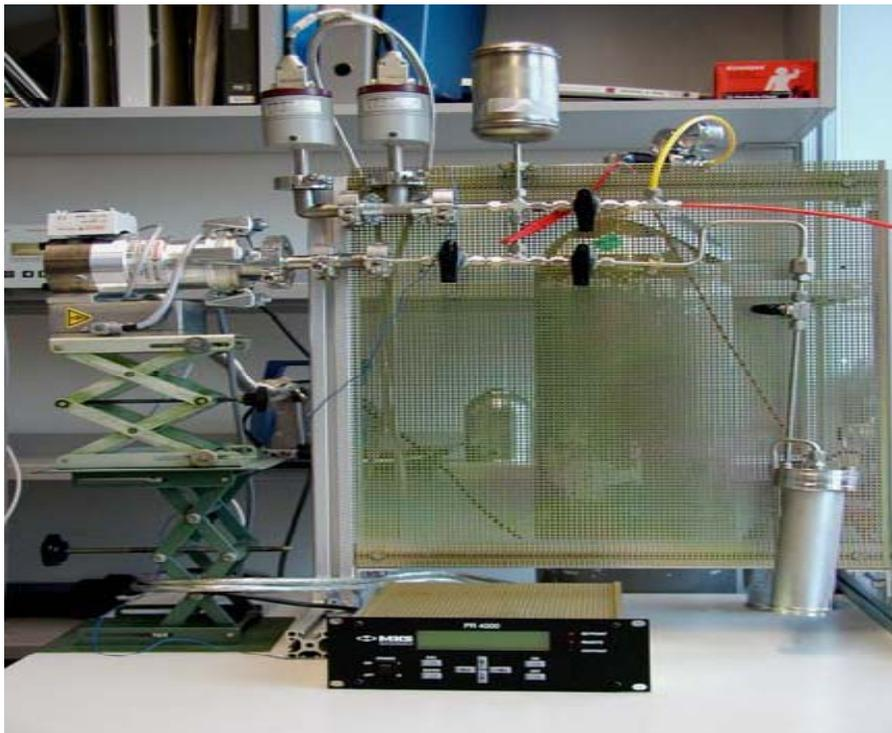
**Fig.3.13. BET instrument to determine the surface area**
