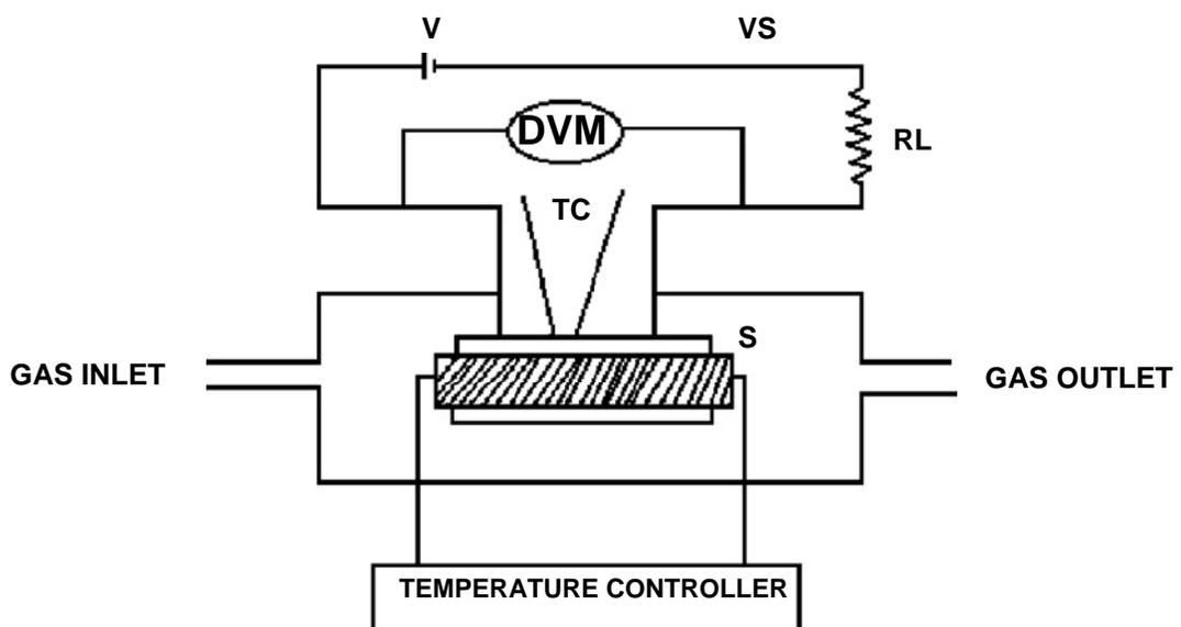
**Fig. 3.20. Electric circuit for gas sensor**
