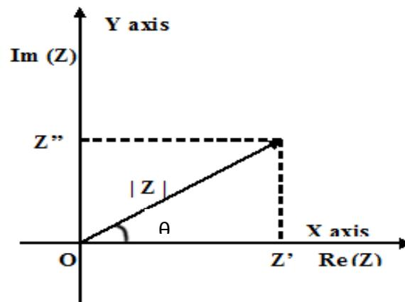
**Fig 3.15. The impedance  $Z$  plotted as a planar vector using rectangular and polar coordinates**
