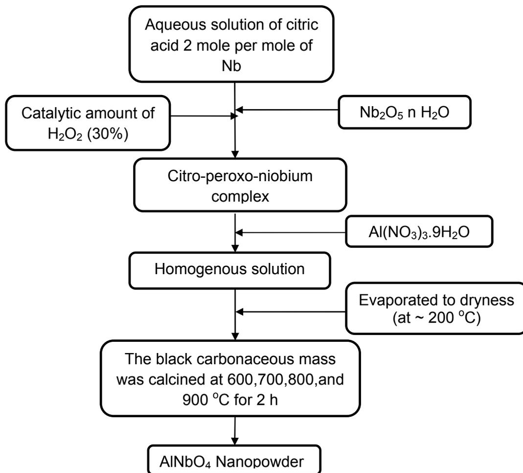
**Fig. 3.4. Flow chart for preparation of AlNbO<sub>4</sub> nanopowder by niobium-citrate complex process**
