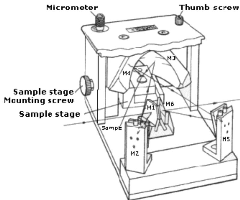
**Fig.3.14. diffuse reflectance accessory optical diagram**
