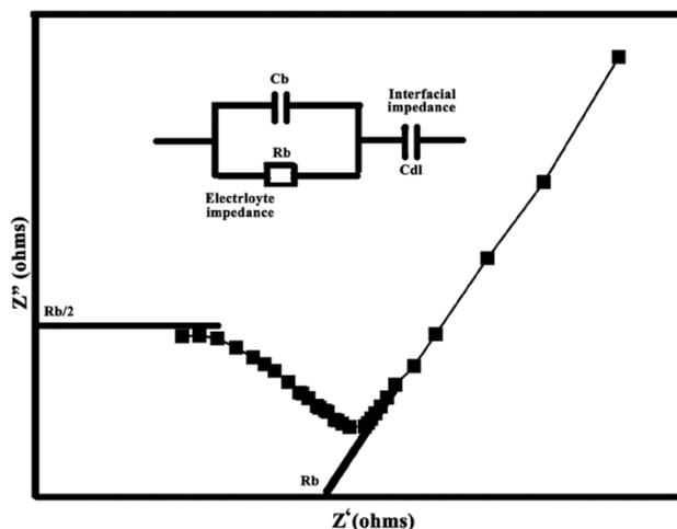
**Fig.3.16. Schematic representation of complex impedance plot**
