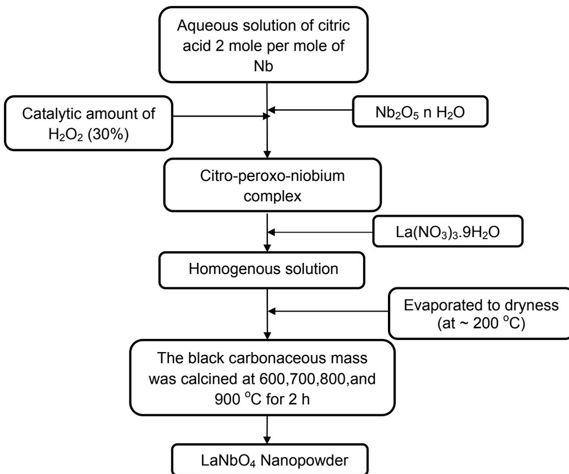
**Fig. 3.5. Flow chart for preparation of LaNbO<sub>4</sub> nanopowder by niobium-citrate complex process**
