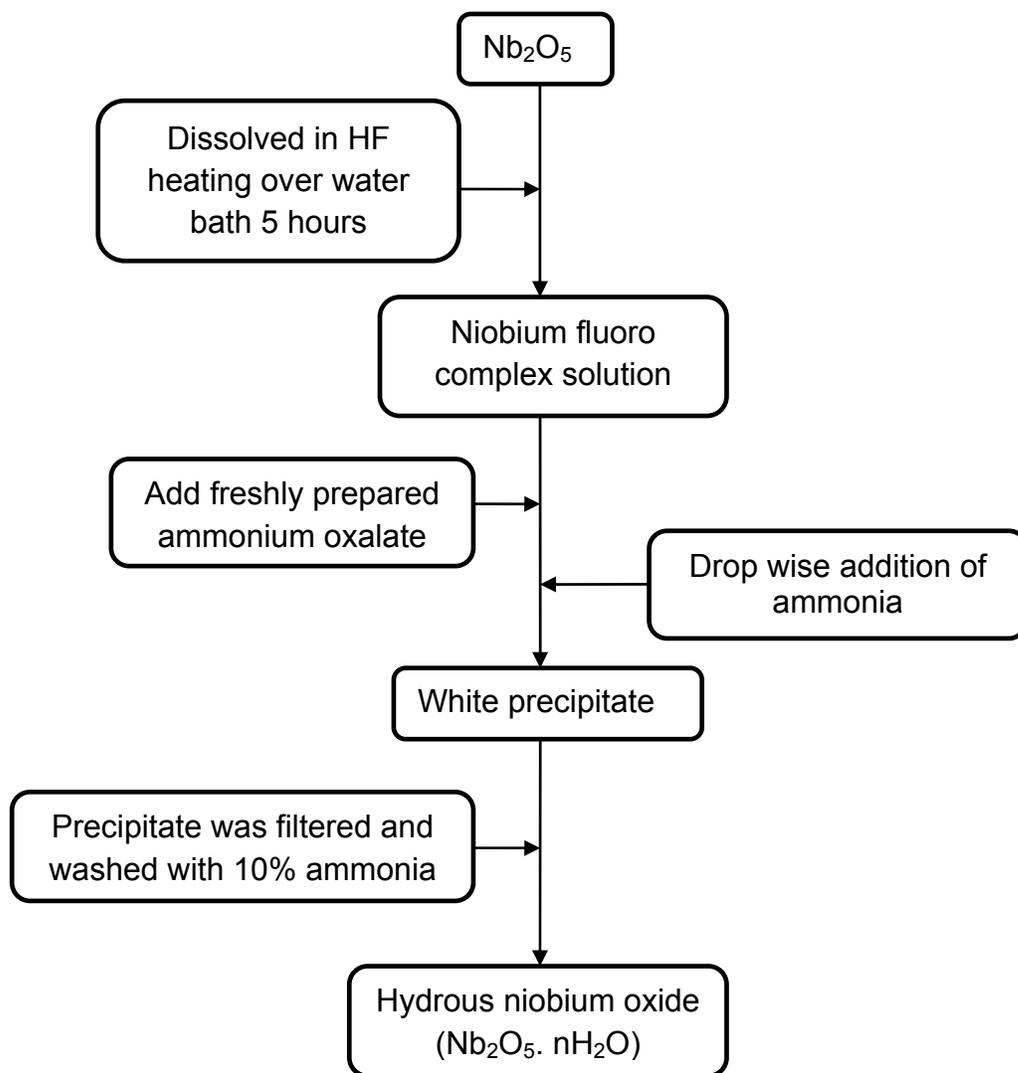
Fig. 3.1. Flow chart for preparation of  $\text{Nb}_2\text{O}_5 \cdot n\text{H}_2\text{O}$
