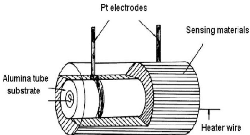
**Fig. 3.19. Sensor element used for gas sensitivity studies**
