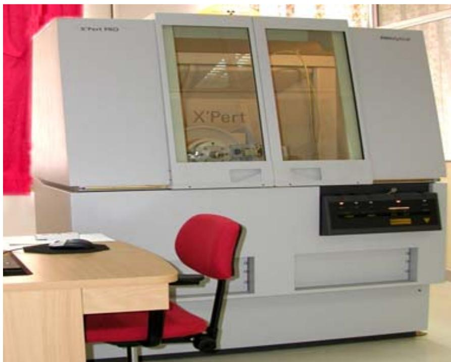
**Fig.3.10. Photograph of X-ray diffractometer**
