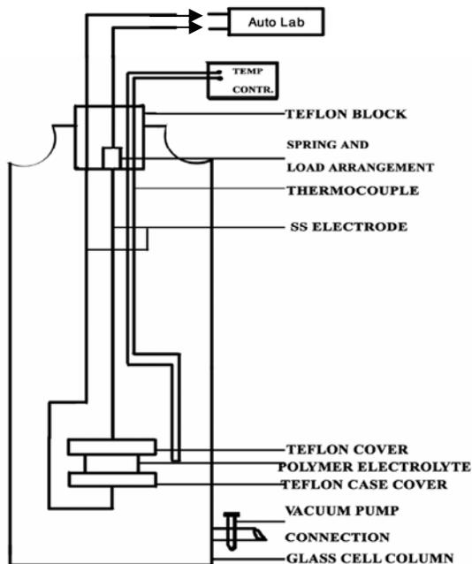
**Fig. 3.17. Schematic representation of conductivity cell diagram**
