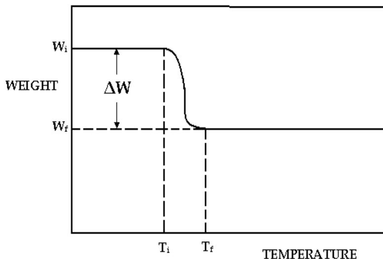
**Fig.3.7. Schematic thermogram for a single step decomposition reaction**
