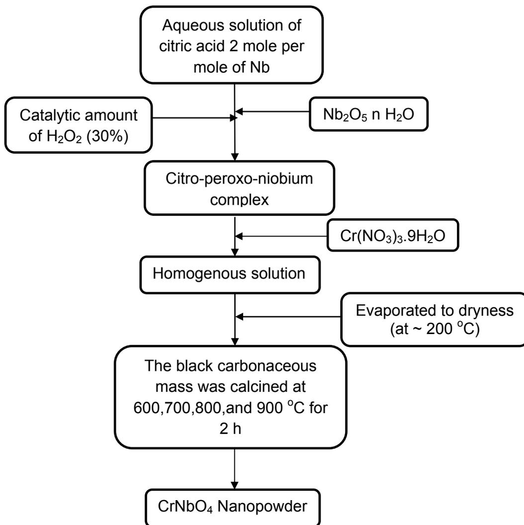
**Fig. 3.3. Flow chart for preparation of CrNbO<sub>4</sub> Nanopowder by niobium-citrate complex process**
