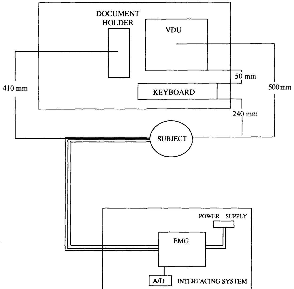
Figure 3.1. Schematic Diagram of Experimental Set-Up.
