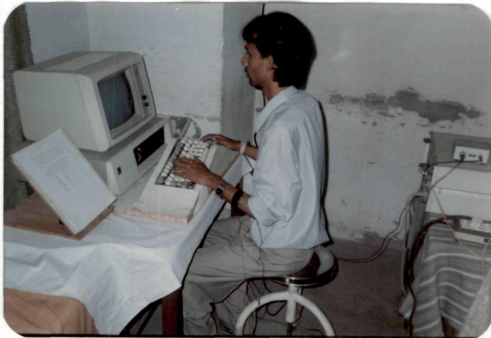
**Figure 3.2.** Photographic View of the experimental set-up showing the subjects seat, the VDU, the document holder, EMG System alongwith the interfacing arrangement.
