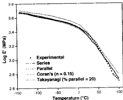
**Figure 4.15:** Experimental and theoretical curves of storage modulus of  $H_{20}$  blends in the whole temperature range
