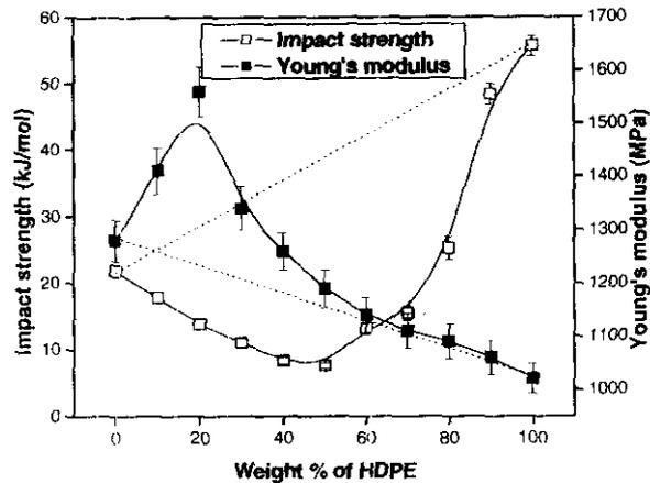
**Figure 4.3:** Effect of blend ratio on the impact strength and Young's modulus of uncompatibilised PP/HDPE blends
