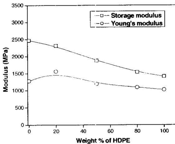
**Figure 4.12:** Comparison of the moduli values obtained from dynamic mechanical and static mechanical tests.
