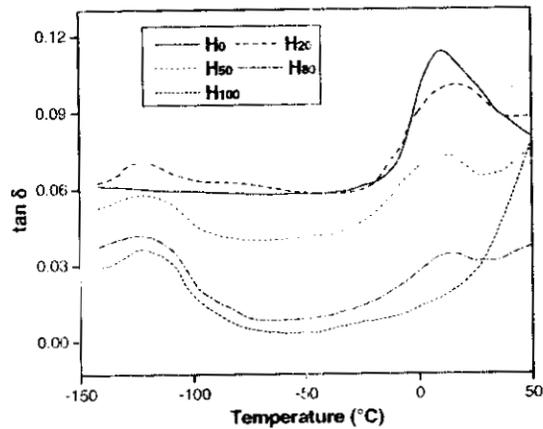
**Figure 4.14:** Effect of blend ratio on the variation of  $\tan \delta$  as a function of temperature
