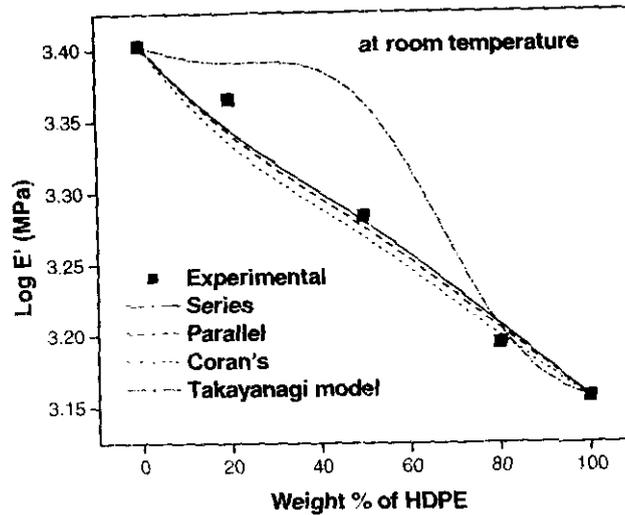
**Figure 4.20:** Comparison of the experimental and theoretical data of storage modulus of PP/HDPE blends at room temperature
