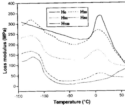
**Figure 4.13:** Effect of blend ratio on the variation of loss modulus as a function of temperature
