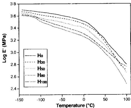
**Figure 4.11:** The variation of storage modulus of PP, HDPE and their blends as a function of temperature.
