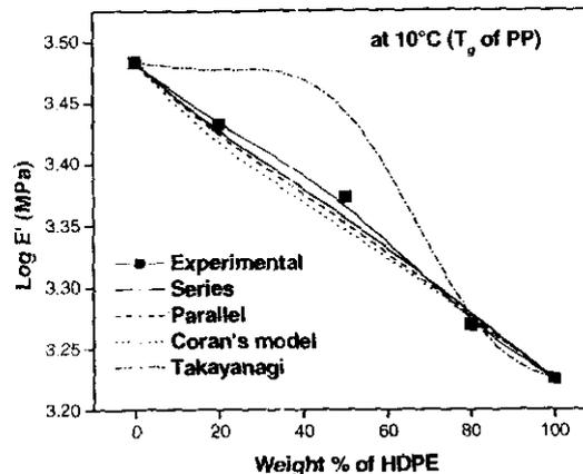
**Figure 4.19:** Comparison of the experimental and theoretical data of storage modulus of PP/HDPE blends at the  $T_g$  of PP
