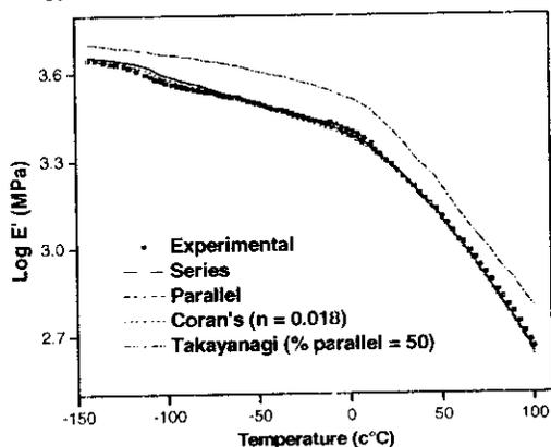
**Figure 4.17:** Experimental and theoretical curves of storage modulus of  $H_{50}$  blends in the whole temperature range
