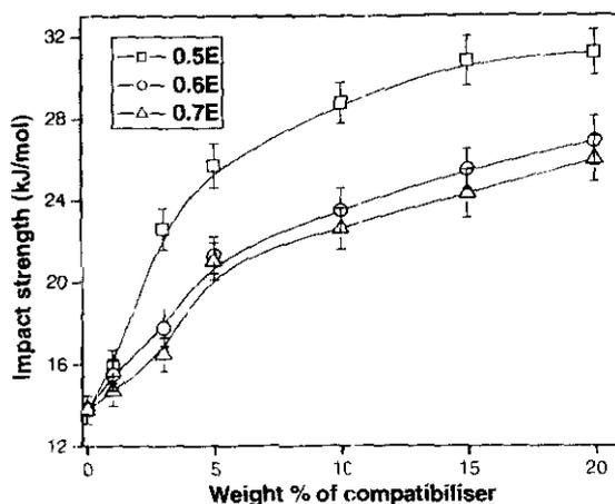
Figure 4.7: Effect of compatibilisation on the impact strength of  $H_{20}$  blends
