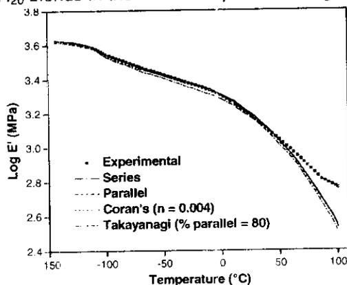
**Figure 4.16:** Experimental and theoretical curves of storage modulus of  $H_{80}$  blends in the whole temperature range
