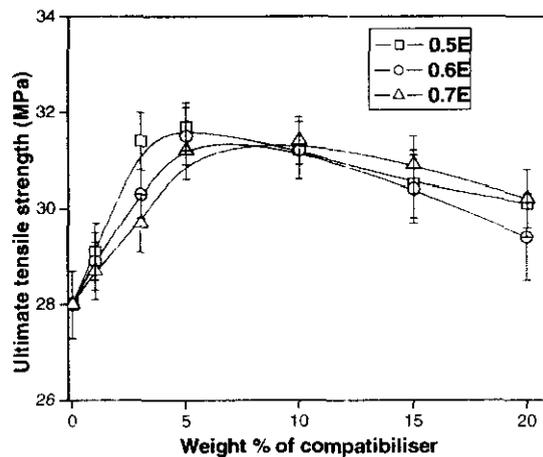
**Figure 4.4:** Effect of compatibilisation on the tensile strength of  $H_{20}$  blends
