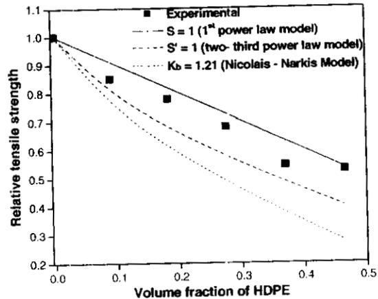
**Figure 4.8:** Plot of relative tensile strength versus volume fraction of dispersed HDPE phase using different models
