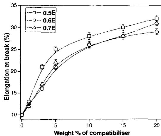
**Figure 4.5:** Effect of compatibilisation on the elongation at break of  $H_{20}$  blends
