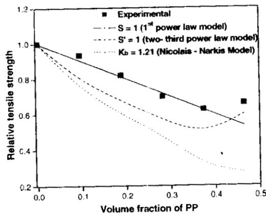
**Figure 4.9:** Plot of relative tensile strength versus volume fraction of dispersed PP phase using different models
