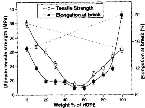
**Figure 4.2:** Effect of blend ratio on the ultimate tensile strength and elongation at break of uncompatibilised PP/HDPE blends
