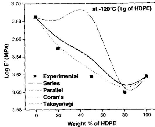
**Figure 4.18:** Comparison of the experimental and theoretical data of storage modulus of PP/HDPE blends at the  $T_g$  of HDPE
