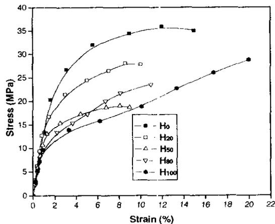
Figure 4.1: Stress-strain behaviour of uncompatibilised PP/HDPE blends
