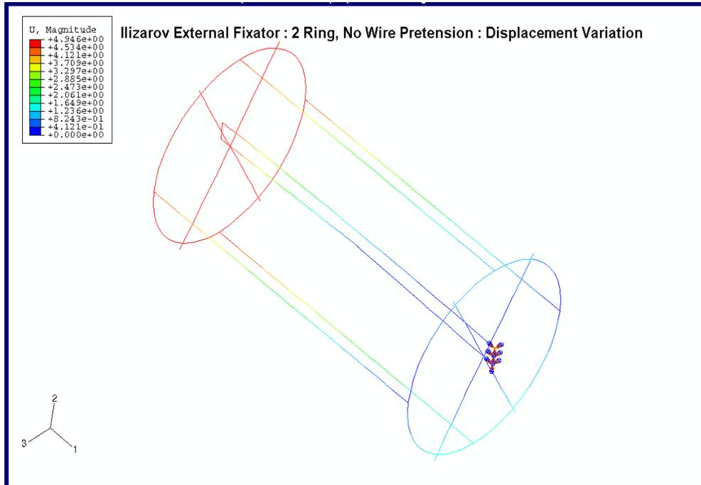
Figure 8.5 – Axial displacement variation in Group 1 construct.
