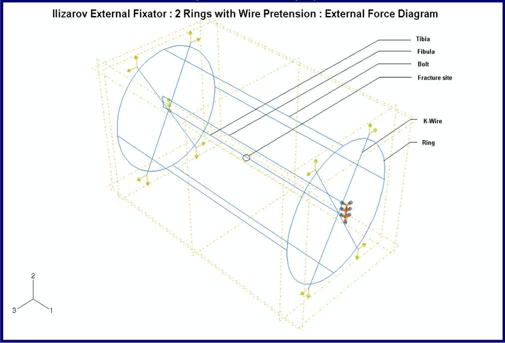
Figure 8.6 - External forces in Group 2 construct.
