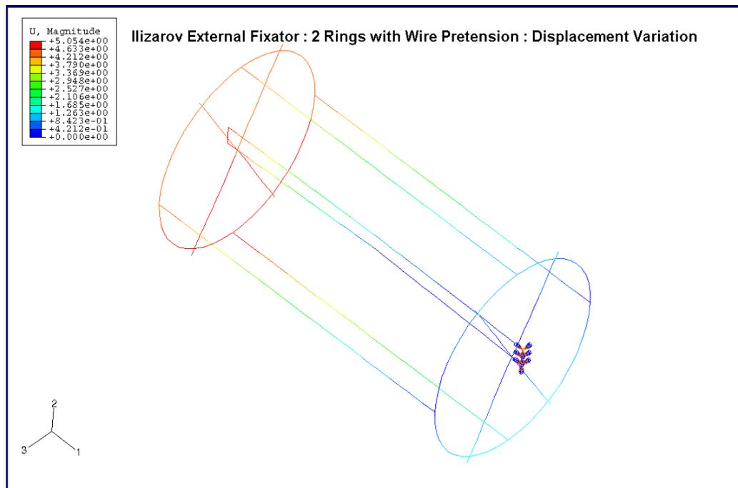
Figure 8.8 – Axial displacement variations in Group 2 construct.
