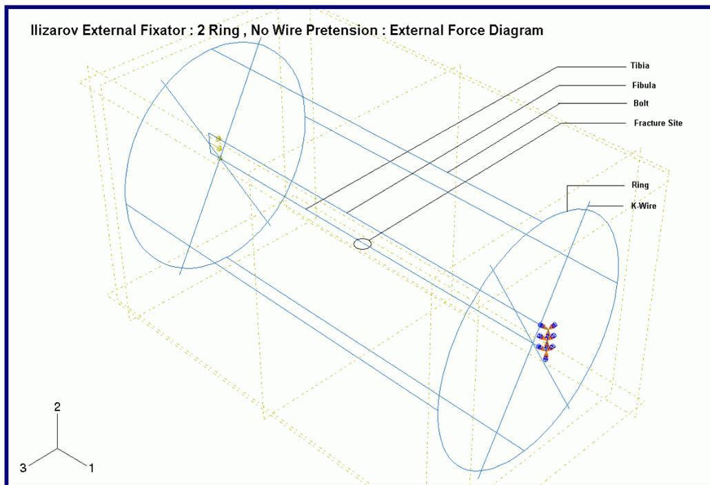
Figure 8.3 - External forces in Group 1 construct.
