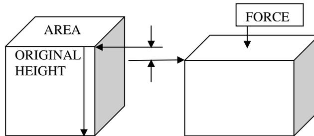
Figure 4.4 - Stress and strain.
