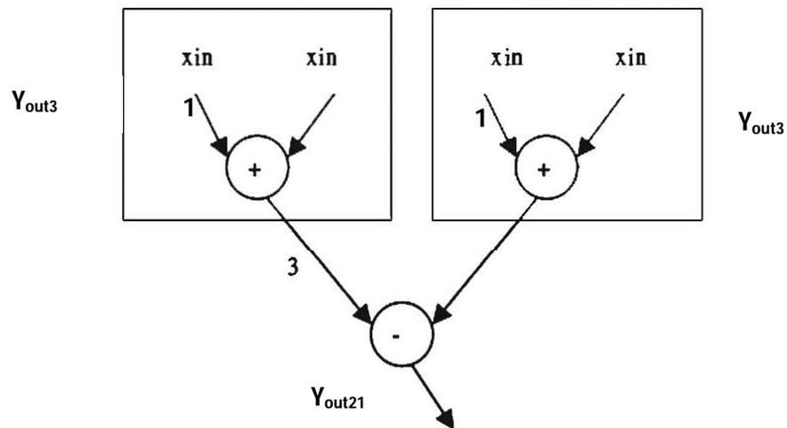
**Figure 3.6 (c) Adder Graph for coefficient 21**
