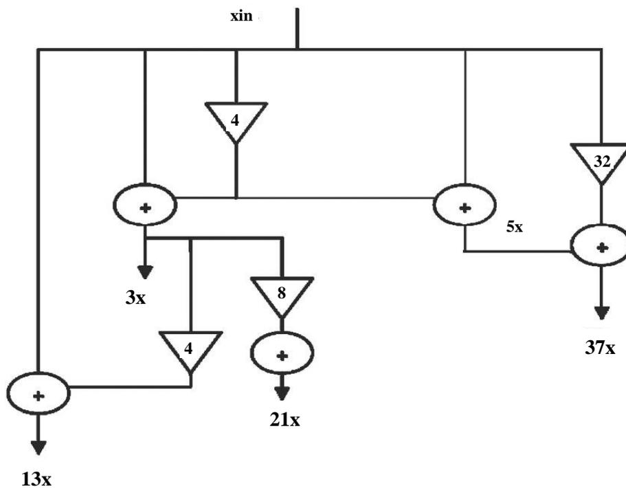
**Figure 3.7 Multiplier blocks for coefficients {3,13,21,37} synthesized by the proposed adder graph method**
