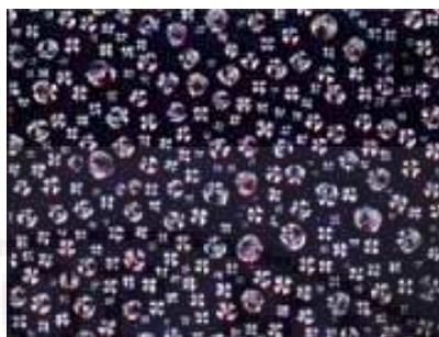
Figure 6.1: An illustrative picture of PDLC
