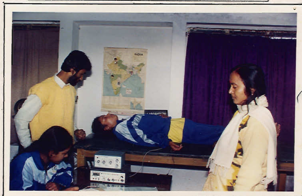
Fig. 6. Recording of Galvanic skin response from the finger tips of a subject.
