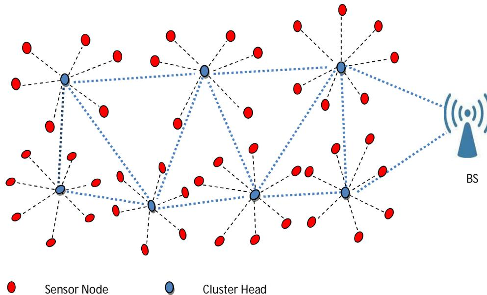
**Figure 4.1 Cluster Based Hierarchical Routing**
