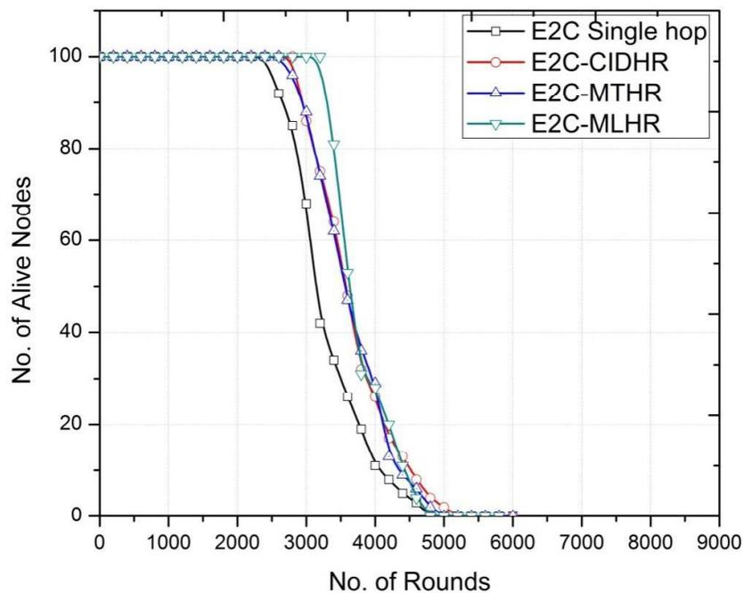
**Figure 4.6 Comparison of the network lifetime for 100m x 100m network with 100 nodes**
