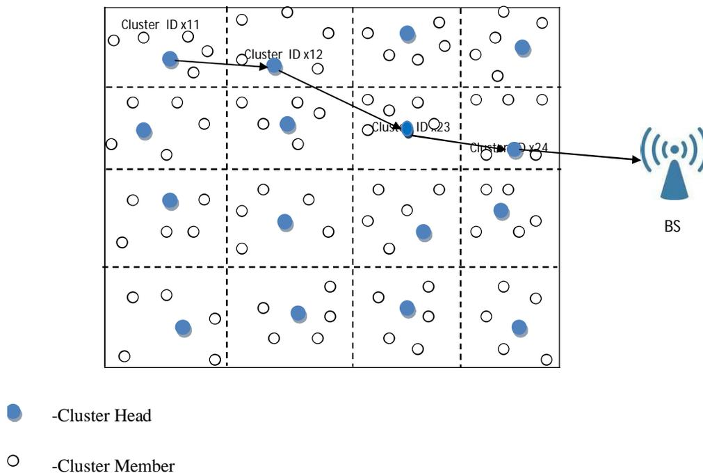
**Figure 4.2 Cluster ID based Hierarchical Routing**
