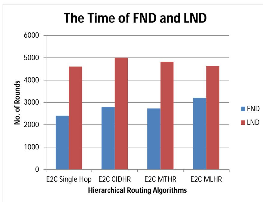
**Figure 4.5 Number of rounds when First and Last Node Dies for 100m x 100m network with 100 nodes**
