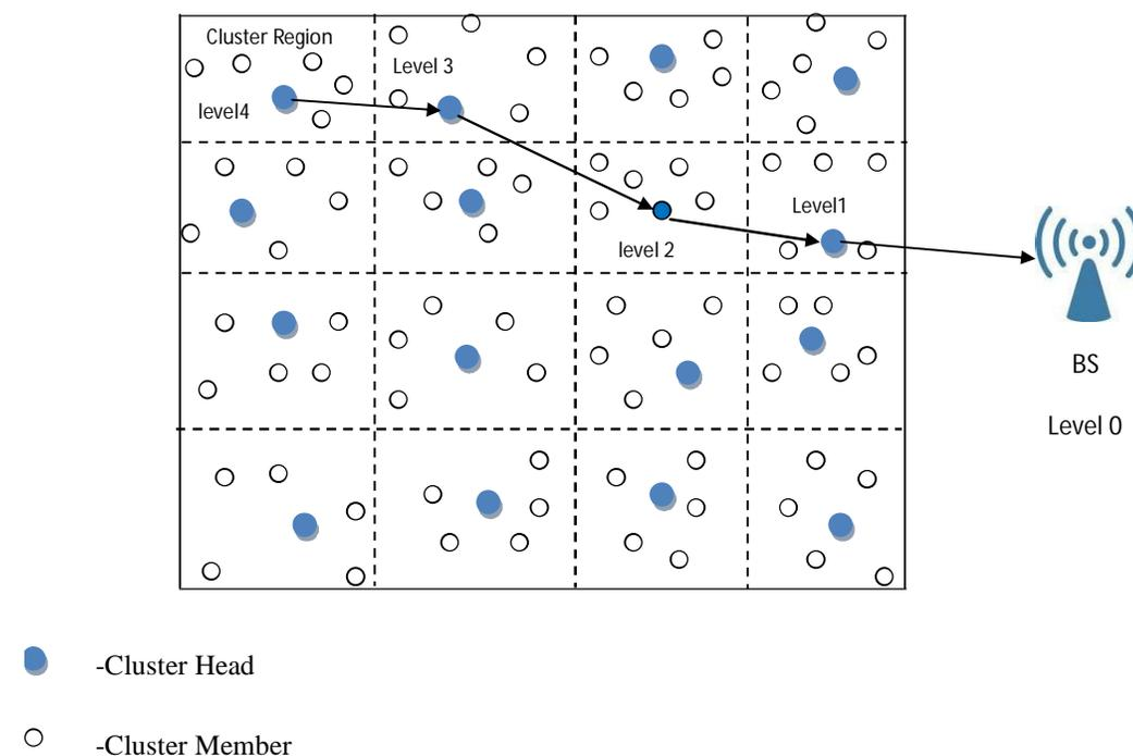
**Figure 4.4 Multi Level Hierarchical Routing**
