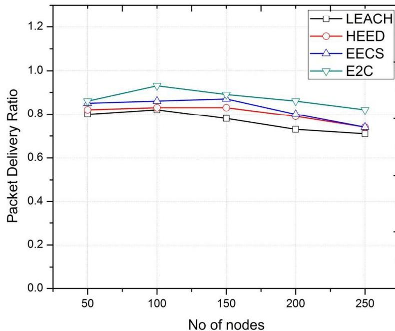
**Figure 3.9 Effect of Number of Nodes on Packet Delivery Ratio**
