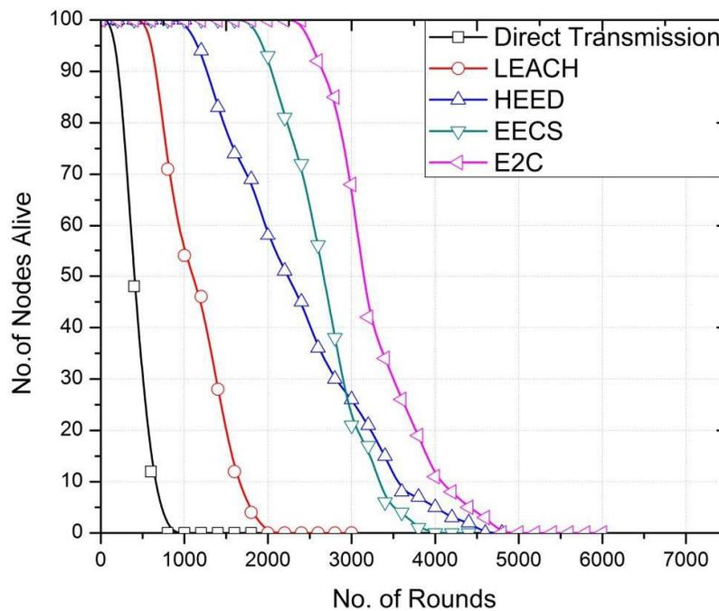
**Figure 3.7 Comparison of the network lifetime for 100m x 100m network with 100 nodes**
