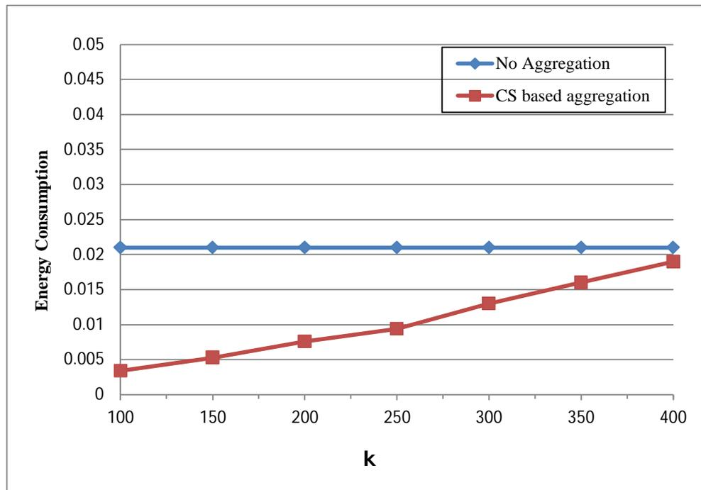
**Figure 5.5 Comparing CS based aggregation against non-aggregation in 1000 node networks**
