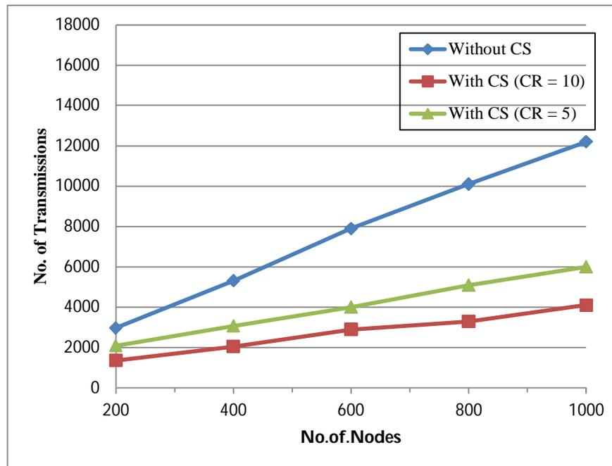
**Figure 5.4** A comparison of the total number of transmissions between the CS-based approach and the traditional transmission approach in the network
