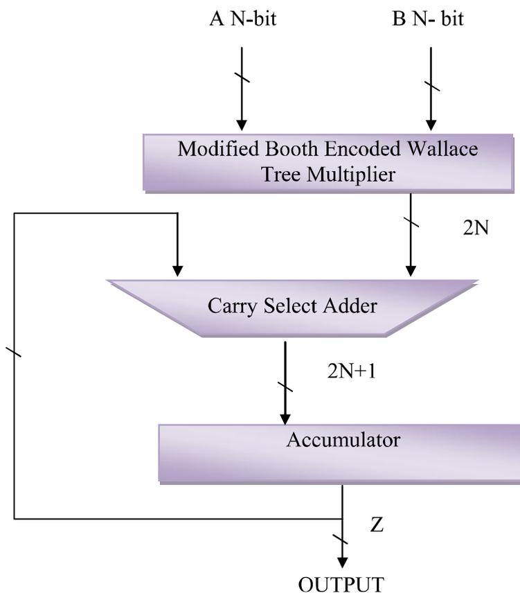
**Figure 5.1 MAC unit with proposed adder and multiplier**
