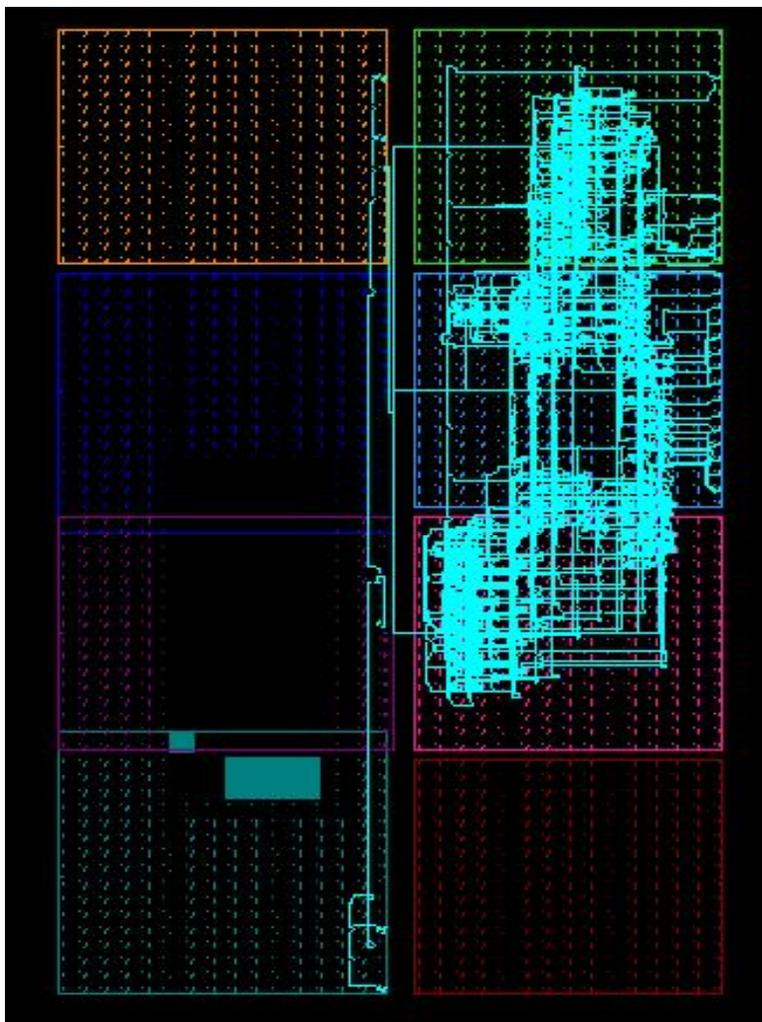
**Figure 5.10 FPGA Floor Plan of FIR filter with proposed MAC unit**
