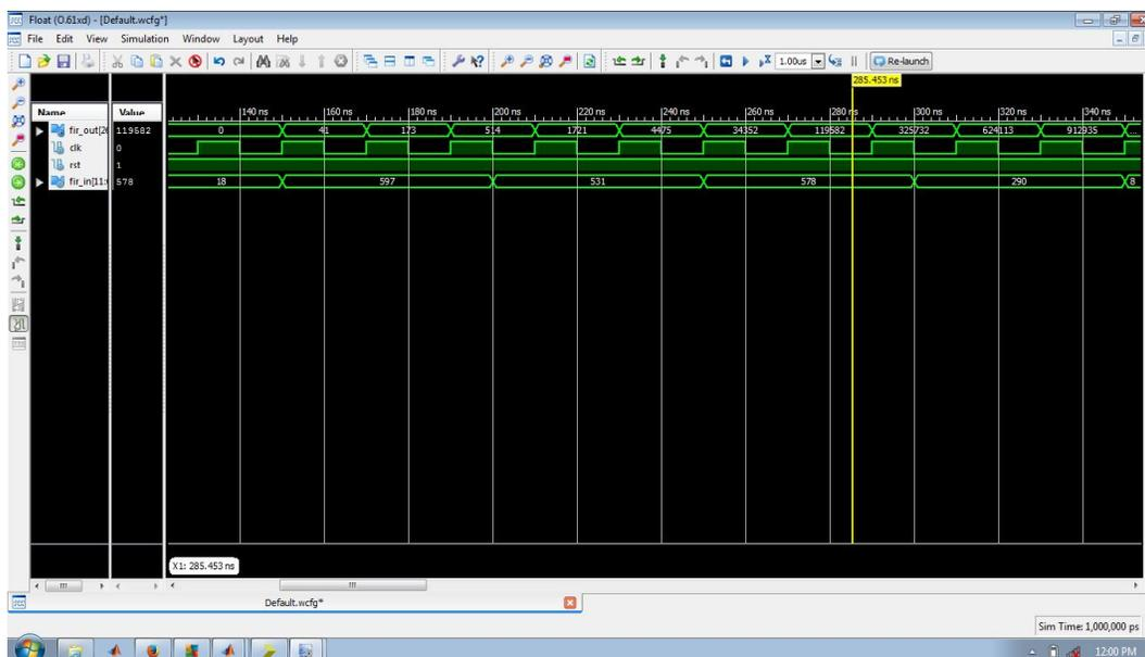
**Figure 5.8 Simulation output of FIR filter with proposed MAC unit**
