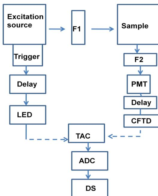
**Figure 2.10** Block diagram representing the concept of time correlated single photon counting. Here Excitation source is a pulsed light source, F1 and F2 are the filters/monochromators, PMT is a fast photomultiplier tube, 'Delay' are the delay lines to adjust the start and stop pulse times. LED is the leading edge timing discriminator, CFTD is the constant fraction timing discriminator, TAC is time to amplitude convertor, DS is the data storage device (computer). Recreated from ref. [106].
