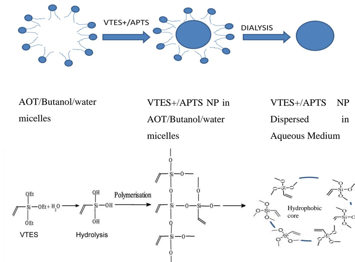
**Figure 2.1** The schematic diagram of combined microemulsion/sol-gel process for producing SiNPs. Recreated from ref. [51, 97]
