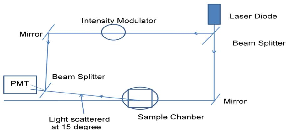
**Figure 2.7** Optical heterodyne used for zeta potential measurement.
