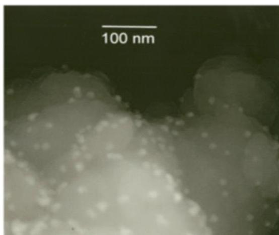
**Fig. 2.1** TEM image of polypyrrole silver synthesized by interfacial polymerization technique
