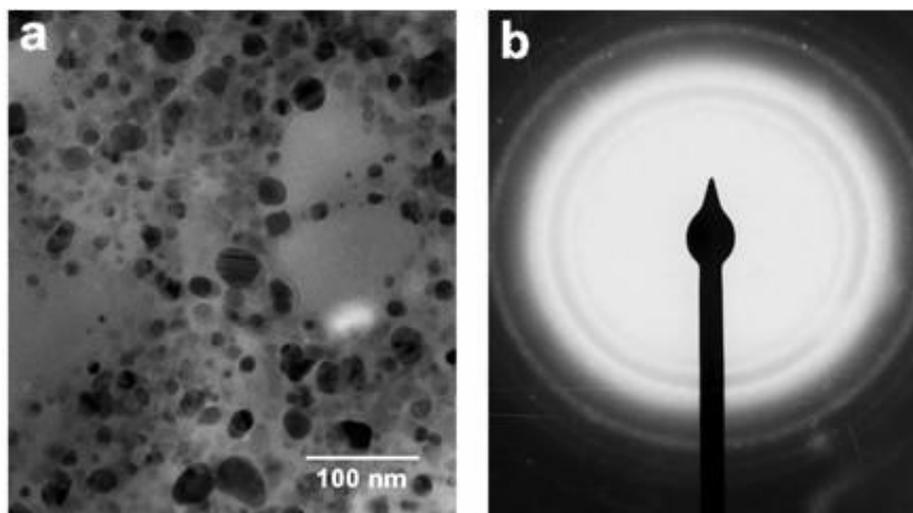
**Fig. 2.4** **a** TEM images of AgNP. **b** ED pattern images of AgNP synthesized using fungus, *Cladosporium cladosporioides*
