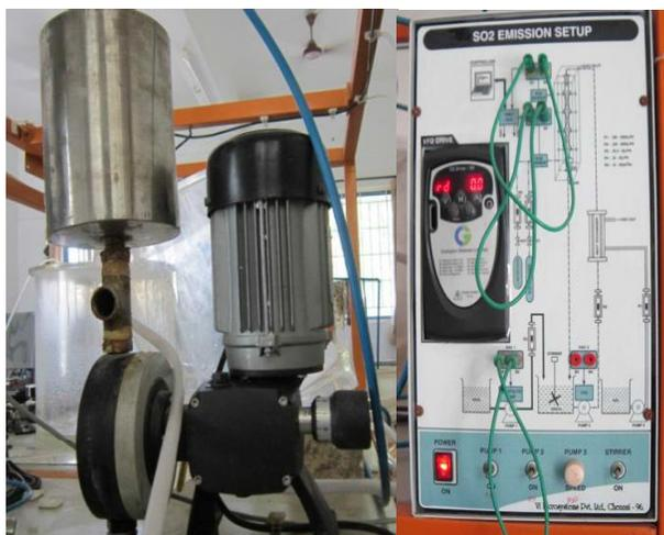
**Figure 4.5 Variable frequency drive with induction motor**
