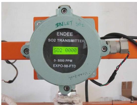
**Figure 4.4 SO<sub>2</sub> gas sensor with transmitter**
