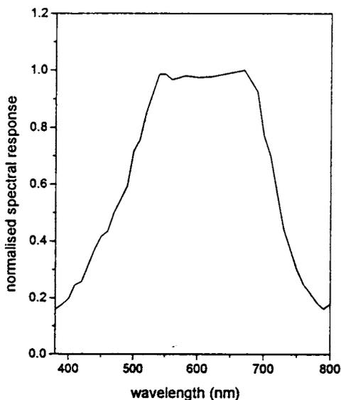
Fig. 8.13 Normalised spectral response of Cell-C
