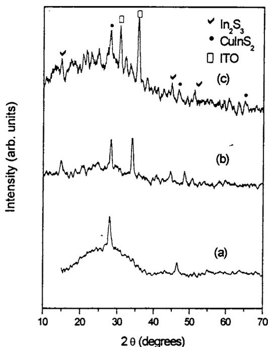
Fig. 8.6 XRD spectra of (a) CuInS<sub>2</sub> (b) In<sub>2</sub>S<sub>3</sub> (c) ITO/CuInS<sub>2</sub>/In<sub>2</sub>S<sub>3</sub>
