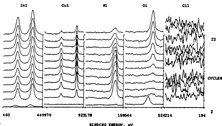
Fig. 8.2 XPS depth profile of Cell-B
