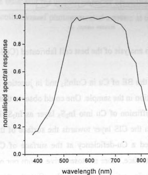
Fig. 8.8 Spectral response of Cell-B
