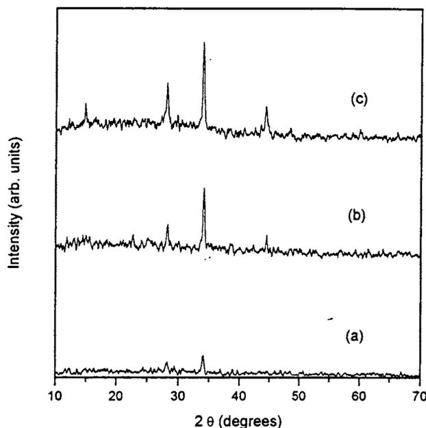
Fig. 8.10 XRD spectrum of In<sub>2</sub>S<sub>3</sub> buffer layer (a) as prepared (b) coated with 5 mg Ag (c) coated with 10 mg Ag (without any annealing)
