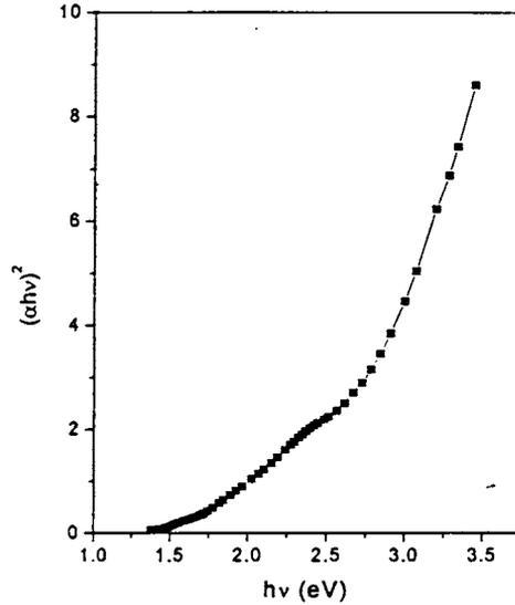
Fig. 8.12 Absorption edges for CuInS<sub>2</sub> and In<sub>2</sub>S<sub>3</sub> (Cell-C)
