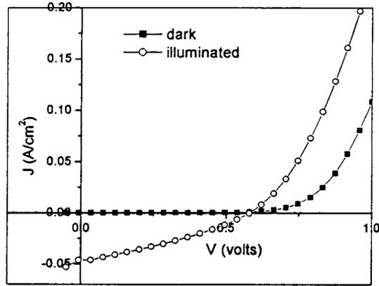
Fig. 8.11 Dark and illuminated J-V characteristics of the best cell fabricated (Cell-C)
