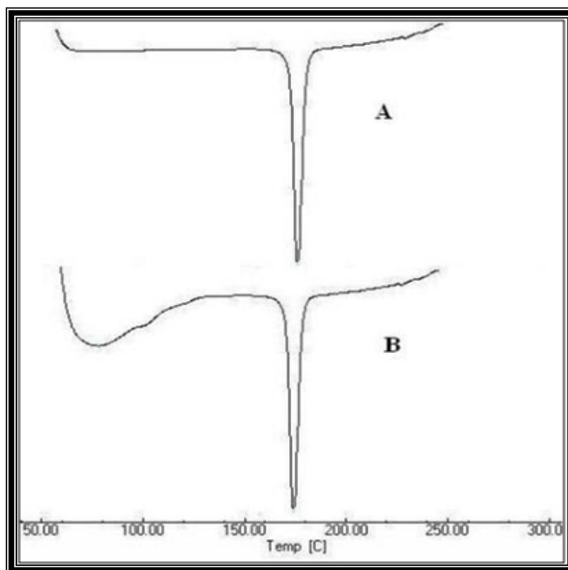
**Figure 5.6 DSC tharmogram of pure Nifedipine (A) and optimized nanosuspension (B)**
