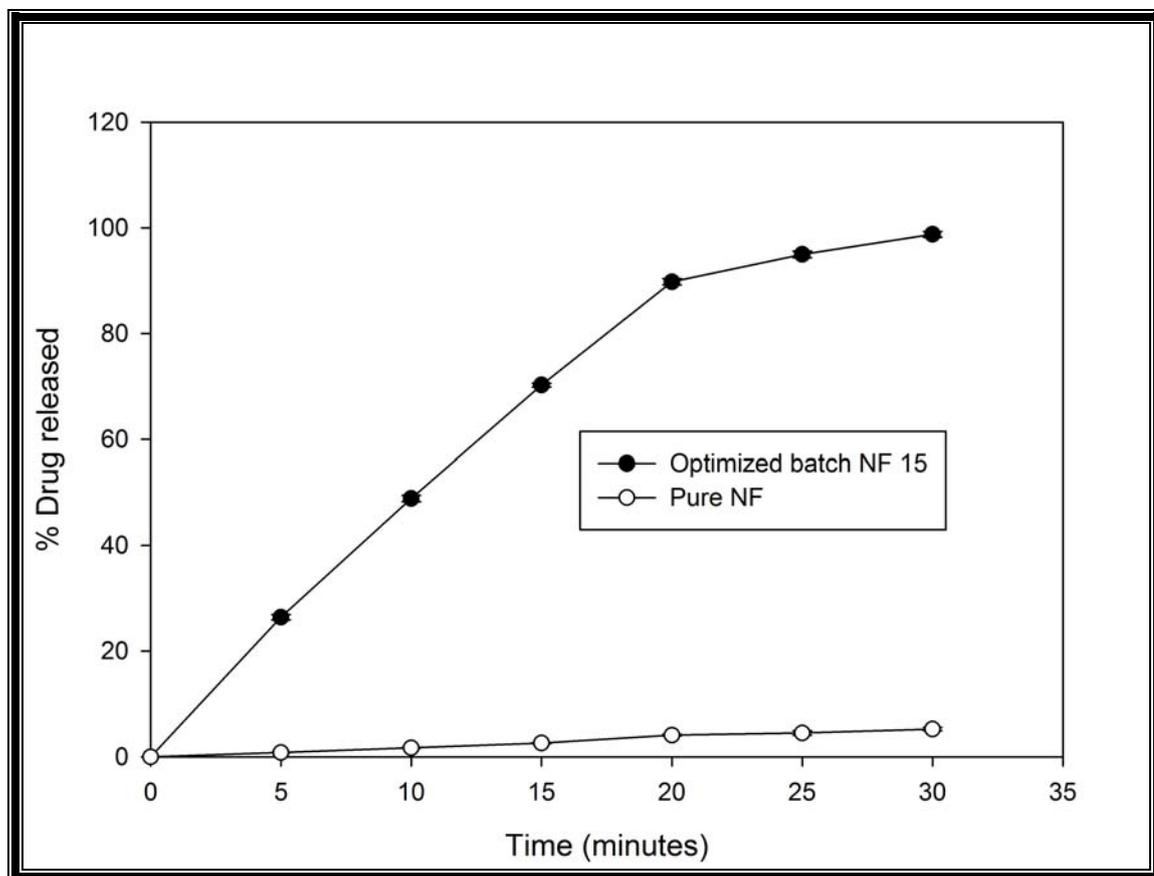
**Figure 5.7 Release profile of pure drug, and optimized nanosuspension formulation in deionized water (0.05% polysorbate 20)**
