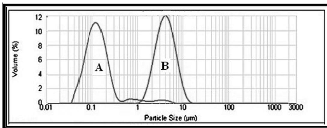
**Figure 5.4. Particle size graph of batch optimized nanosuspension NF 15 (A) and pure drug (B)**
