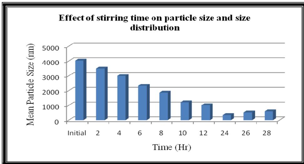
**Figure 5.2 Effect of stirring time on particle size and size distribution (Batch NF 3)**
