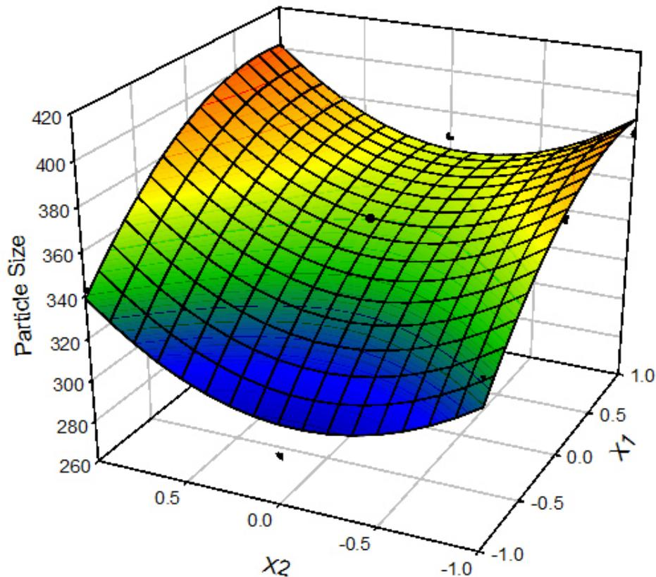
**Figure 5.3 Response surface plot of effect drug to stabilizer ratio ( $X_1$ ) and % V/V of milling media ( $X_2$ ) on particle size distribution**
