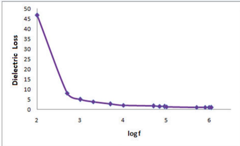
Figure 6.6: Variation of Dielectric loss as a function of Frequency for 6MNA
