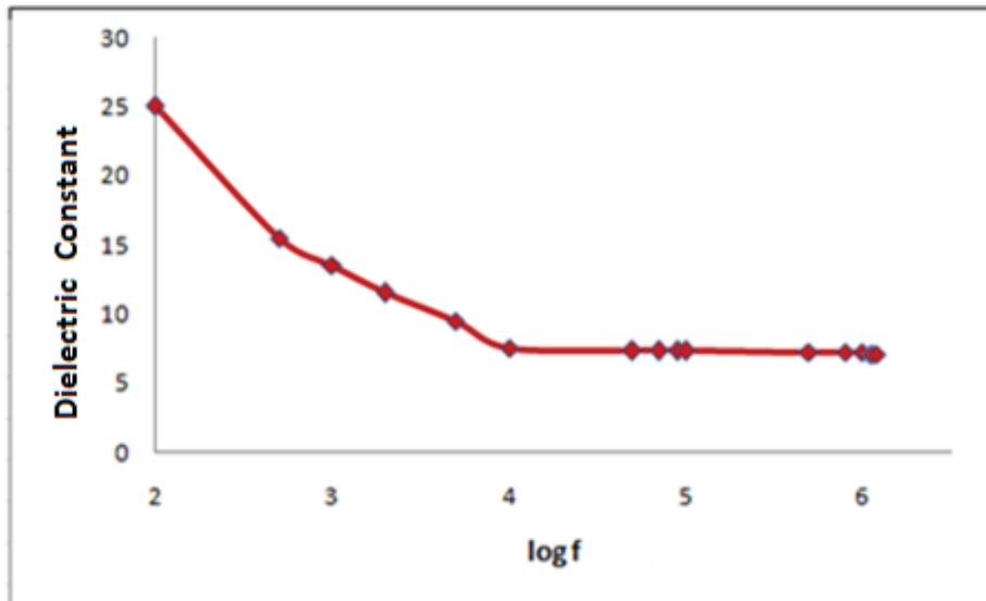
Figure 6.3: Variation of Dielectric Constant as a function of Frequency for ACD
