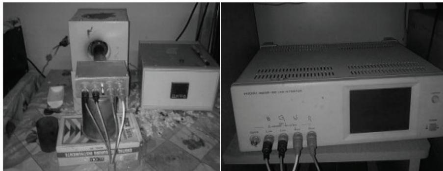
Figure 6.1: HIOKI 3532-50 LCR-HITESTER for dielectric measurement
