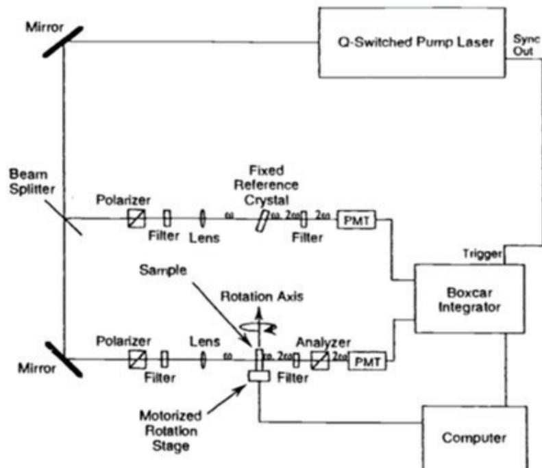
**Figure 6.11: Schematic experimental setup for SHG efficiency measurement**
