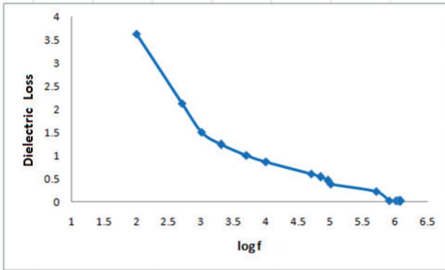
Figure 6.8: Variation of Dielectric Loss as a function of Frequency for AMA
