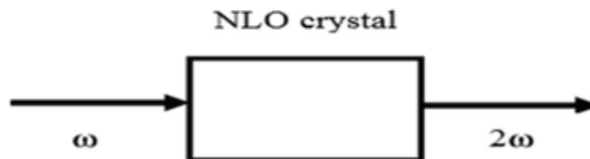
**Figure 6.10 : Schematic diagram of SHG**
