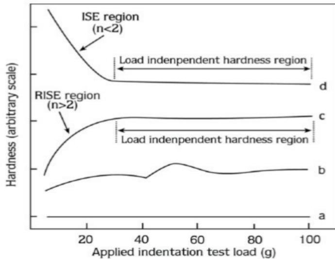
**Figure 5.6: Schematic representation of hardness applied indentation test load variation.**
