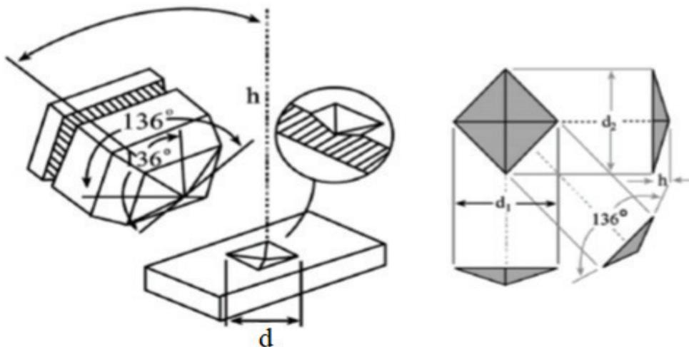
**Figure 5.7: Vickers indentation and indentation diagonal length**
