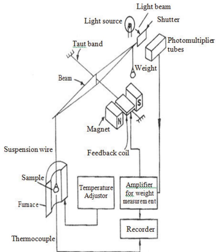
Figure 5.1: Schematic Experimental Setup of TGA Equipment
