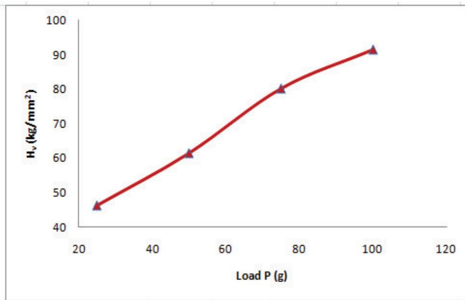
Figure 5.9 Variation of Vicker's microhardness number  $H_v$  with load P for ACD
