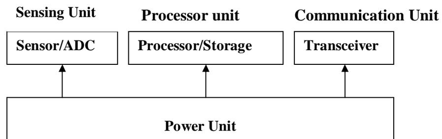
**Figure 1.1 Essential Components of a Sensor Node**
