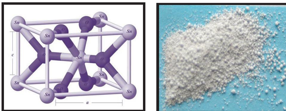
**Figure 1.3.** Schematic diagram of rutile type tetragonal structure and powder form of SnO<sub>2</sub> nanoparticle.
