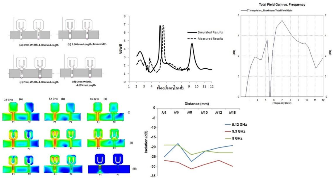
Figure 3.6: Geometry and results of MIMO antenna for band notch characteristics
