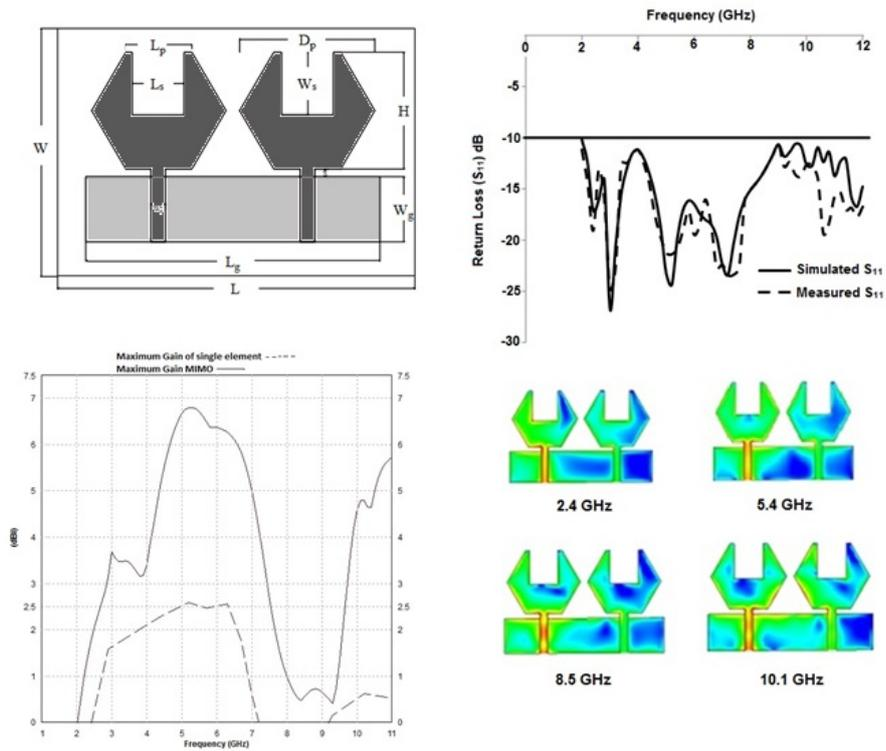
Figure 3.5: Geometry and results of two elements spanner shape MIMO antenna for UWB applications
