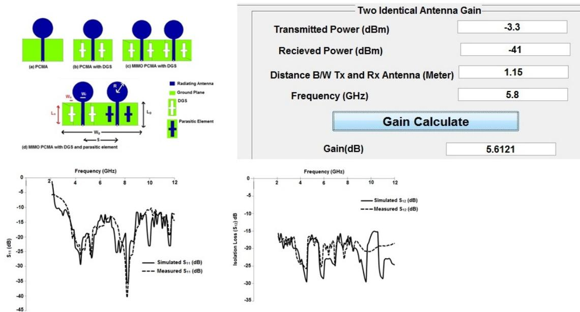
Figure 3.4: Configuration and results of MIMO antenna with 2- elements with DGS and parasitic structure for UWB applications
