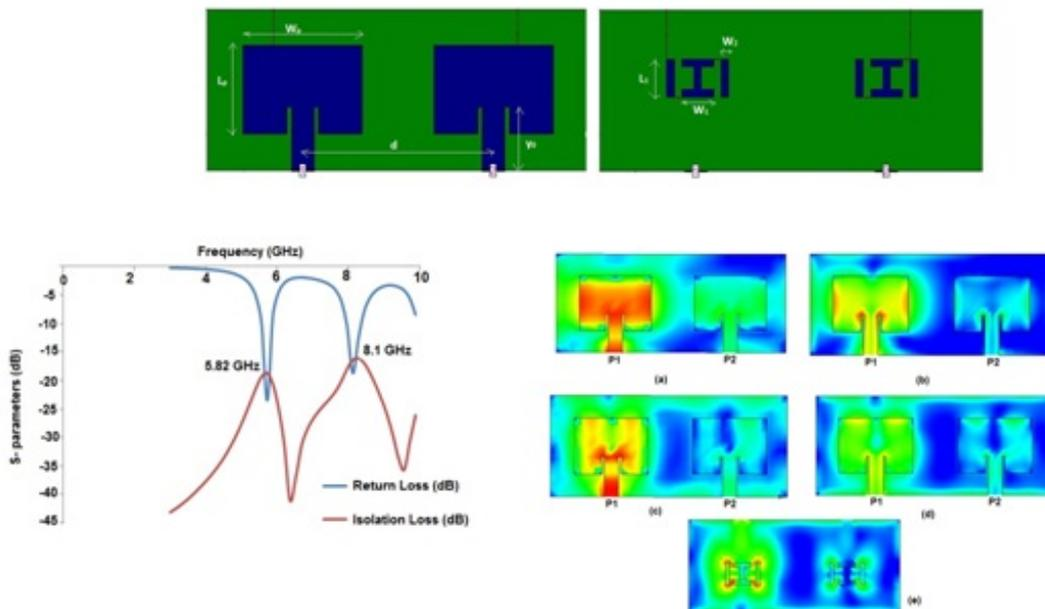
Figure 3.1: Configuration and results of DGS -two elements MIMO antenna
