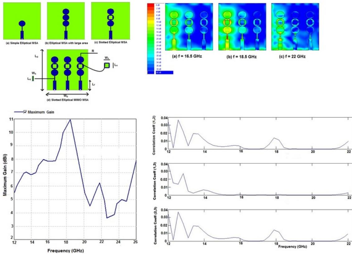
Figure 3.3: Geometry and results of three element slotted MIMO antenna
