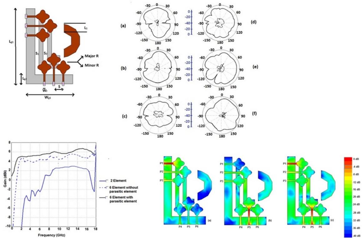
Figure 3.8: Geometry and results of six elements MIMO antenna for polarization characteristics
