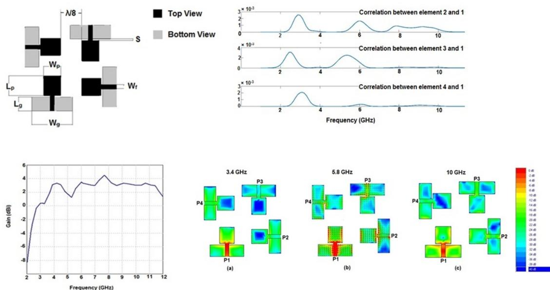
Figure 3.7: Geometry and results of four elements MIMO antenna for polarization characteristics
