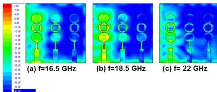
Figure 6.8: Simulated surface current distribution of for 3-element slotted diversity antenna
