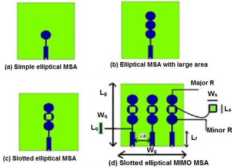
Figure 6.1: Structure of 3-element MIMO antenna
