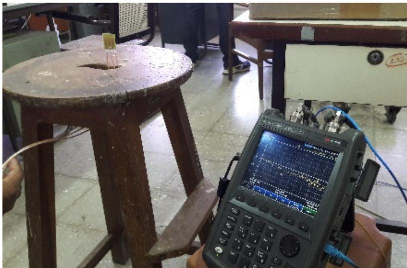
Figure 6.3: Testing using vector network analyzer ( $S_{11}$  and  $S_{12}/S_{13}$ )
