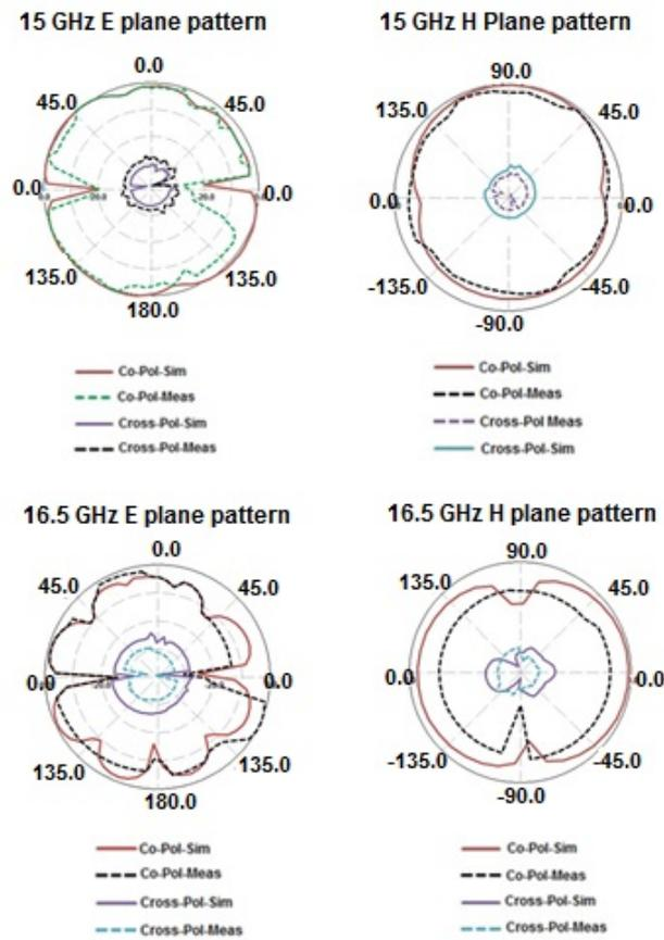
Figure 6.6: Comparison of radiation characteristics for 3-element slotted diversity antenna
