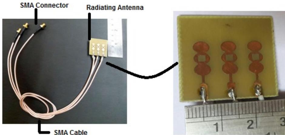
Figure 6.2: Fabricated prototype of 3-element slotted diversity antenna
