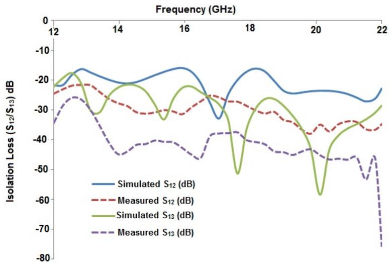
Figure 6.5: Comparative study of simulated and hardware results of  $S_{12} / S_{13}$  for 3-element slotted diversity antenna
