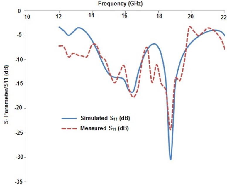
Figure 6.4: Comparative study of simulated and hardware results of  $S_{11}$  for 3-element slotted diversity antenna
