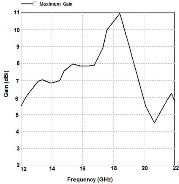
Figure 6.7: Simulated maximum gain of for 3-element slotted diversity antenna
