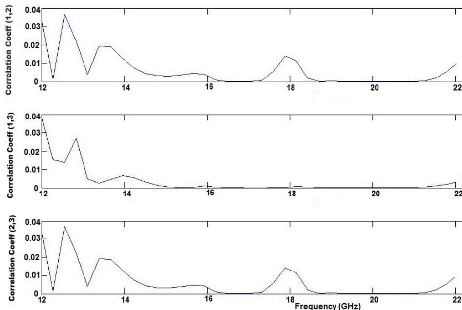
Figure 6.9: Simulated ECC (Envelope Correlation Coefficient) of for 3-element slotted diversity antenna
