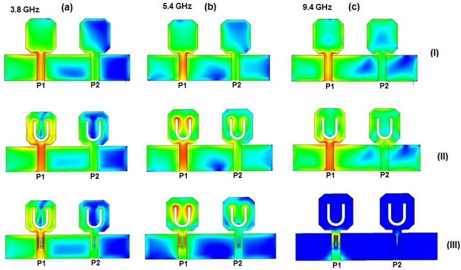
Figure 5.13: surface current distribution characteristics of dual notched MIMO antenna
