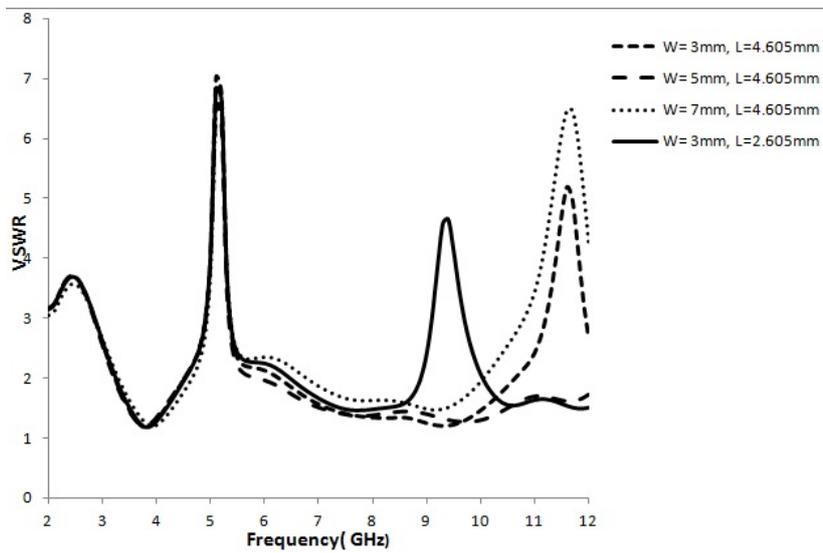
Figure 5.5: Comparative study of VSWR by changing lengths and width of slot on feed line
