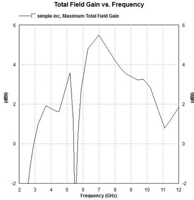
Figure 5.11: Gain variation of dual notched MIMO antenna
