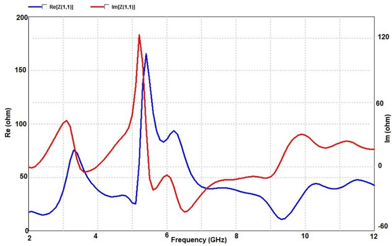
Figure 5.9: Impedance variation plots for dual notched MIMO antenna
