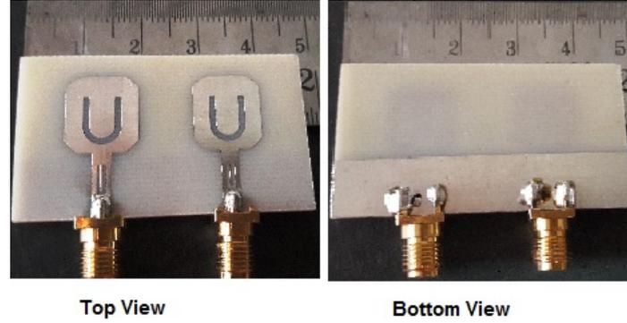
Figure 5.6: Fabricated MIMO antenna with dual notched characteristics
