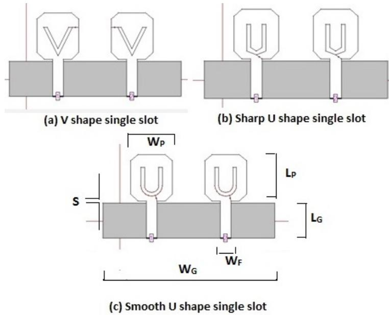
Figure 5.2: Basic structure of single notch antenna
