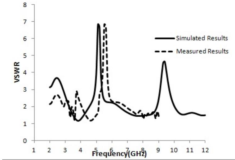
Figure 5.7: Comparative study of simulated and measured VSWR for dual notched MIMO antenna
