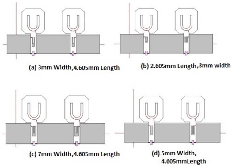
Figure 5.4: Different antenna configurations for creation of dual notch characteristics
