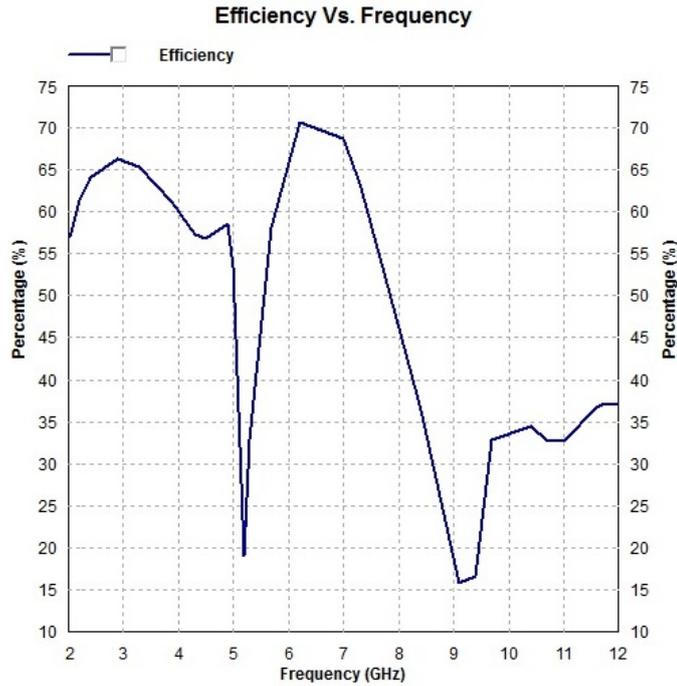
Figure 5.12: Radiation efficiency of dual notched MIMO antenna
