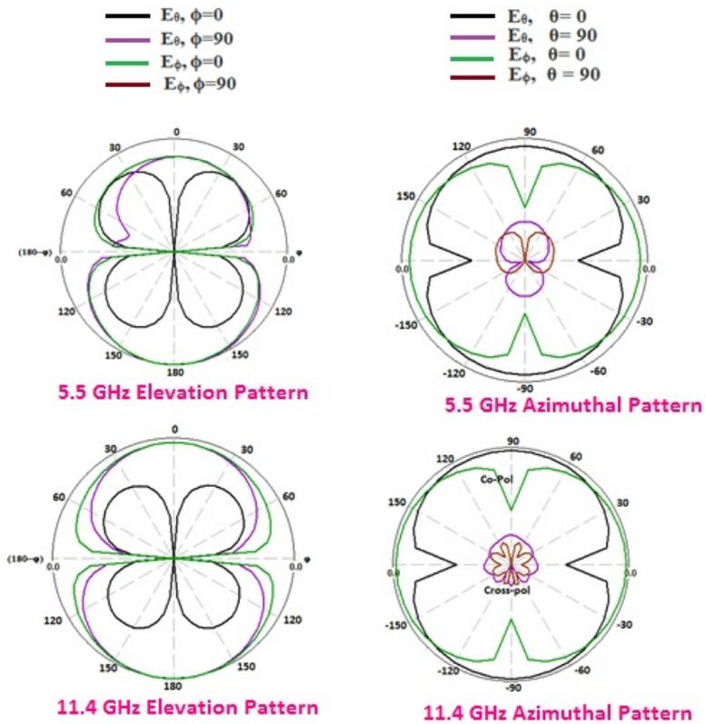
Figure 5.10: Radiation characteristics for dual notched MIMO antenna(E-plane and H-plane)
