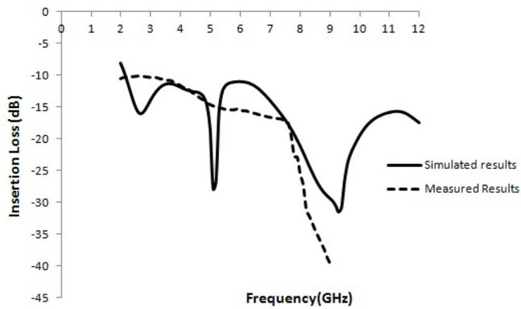
Figure 5.8: Isolation characteristics for dual notched MIMO antenna
