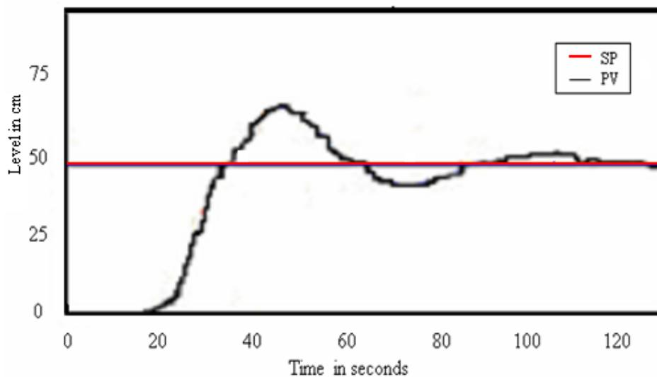
**Figure 3.8** Real time response for a change in process parameter from  $b = 2.2$  to  $b = 4.4$  given by opening the outlet valve completely from the middle(normal) position.
