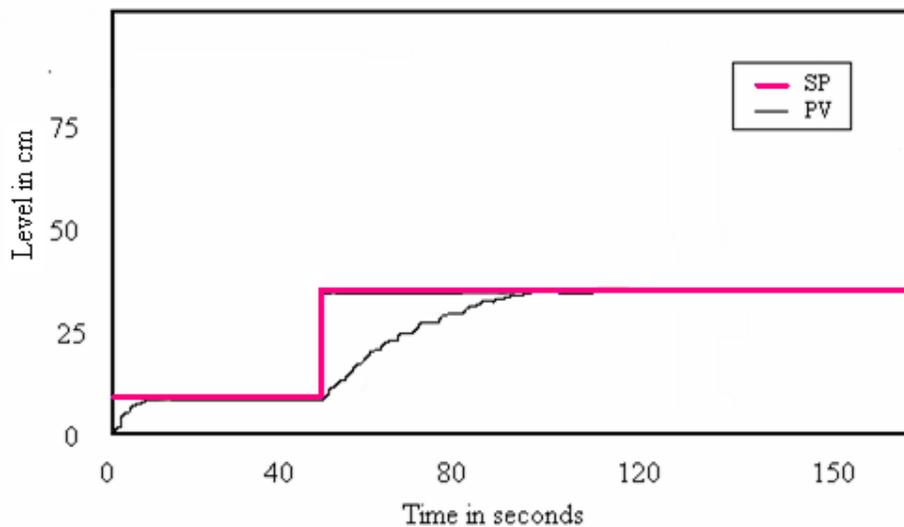
**Figure 3.2** Real time response for a step increase in the set point from 10 cm to 38 cm at  $t = 50$  seconds
