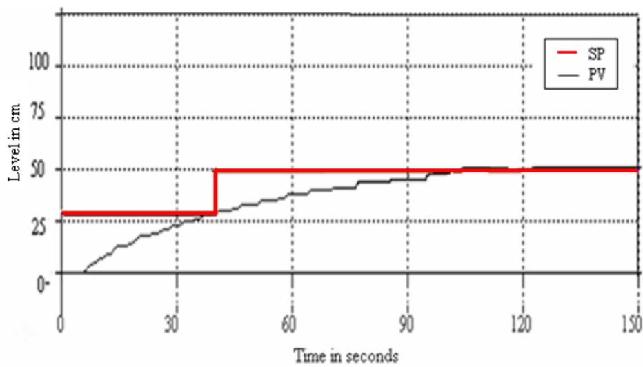
**Figure 3.5 Real time response for a step increase in set point from 28 cm to 50 cm at  $t = 40$  seconds**
