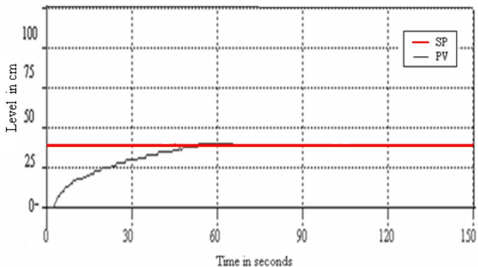
**Figure 3.4** Real time response for a step increase in set point from 0 to 38 cm
