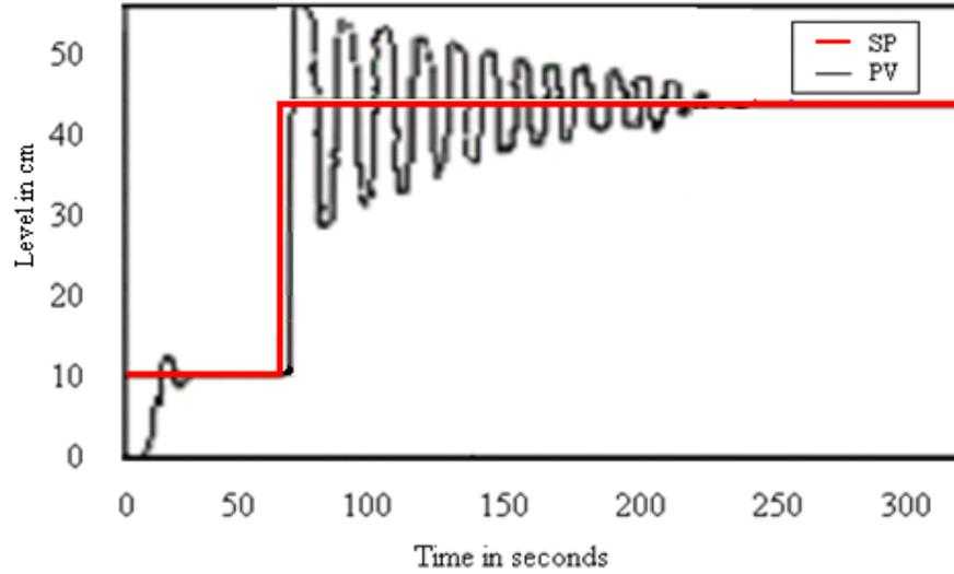
**Figure 3.7** Simulated response for a change in process parameter from  $b = 2.2$  to  $b = 4.4$  given by opening the outlet valve completely from the middle(normal) position
