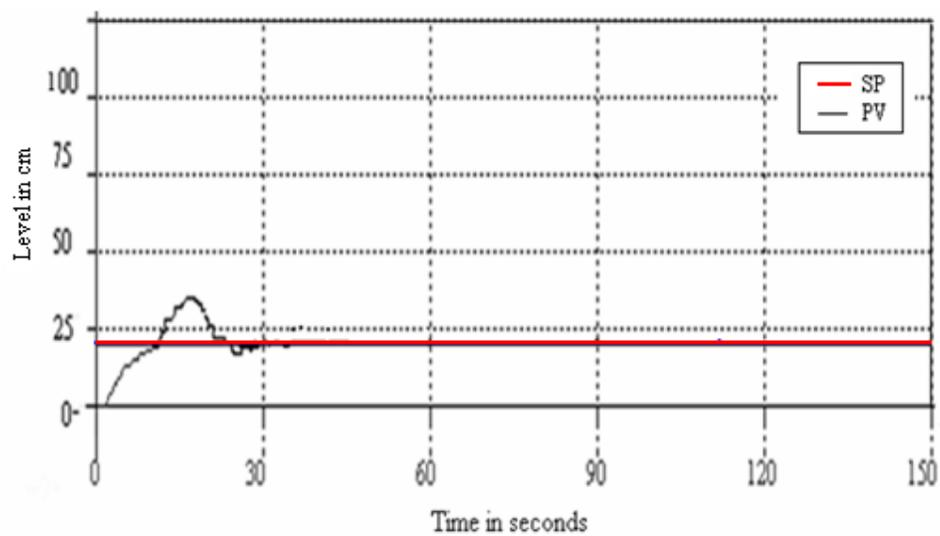
**Figure 3.6 Real time response for a step increase in load given by sudden opening of the inlet valve by 10%**
