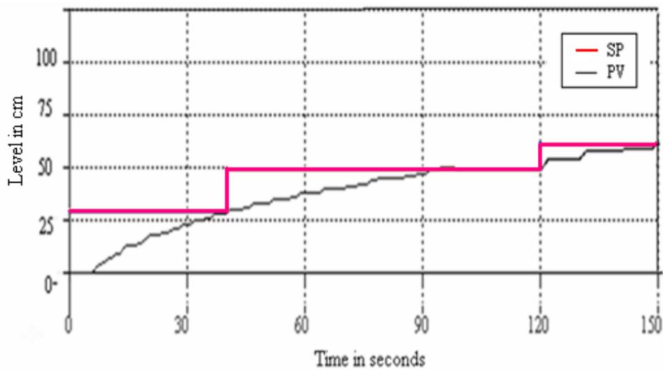
**Figure 3.3** Real time response for a step increase in set point from 28 cm to 50 cm at  $t = 40$  seconds and from 50 cm to 68 cm at  $t = 120$  seconds
