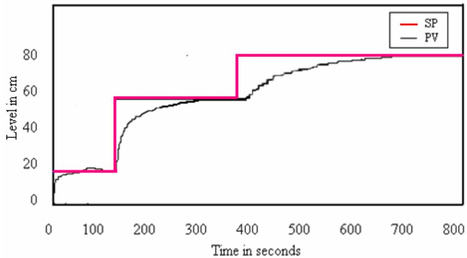
**Figure 3.1** Simulated response for a step increase in set point from 20 cm to 60 cm at  $t = 150$  seconds and from 60 cm to 80 cm at  $t = 400$  seconds
