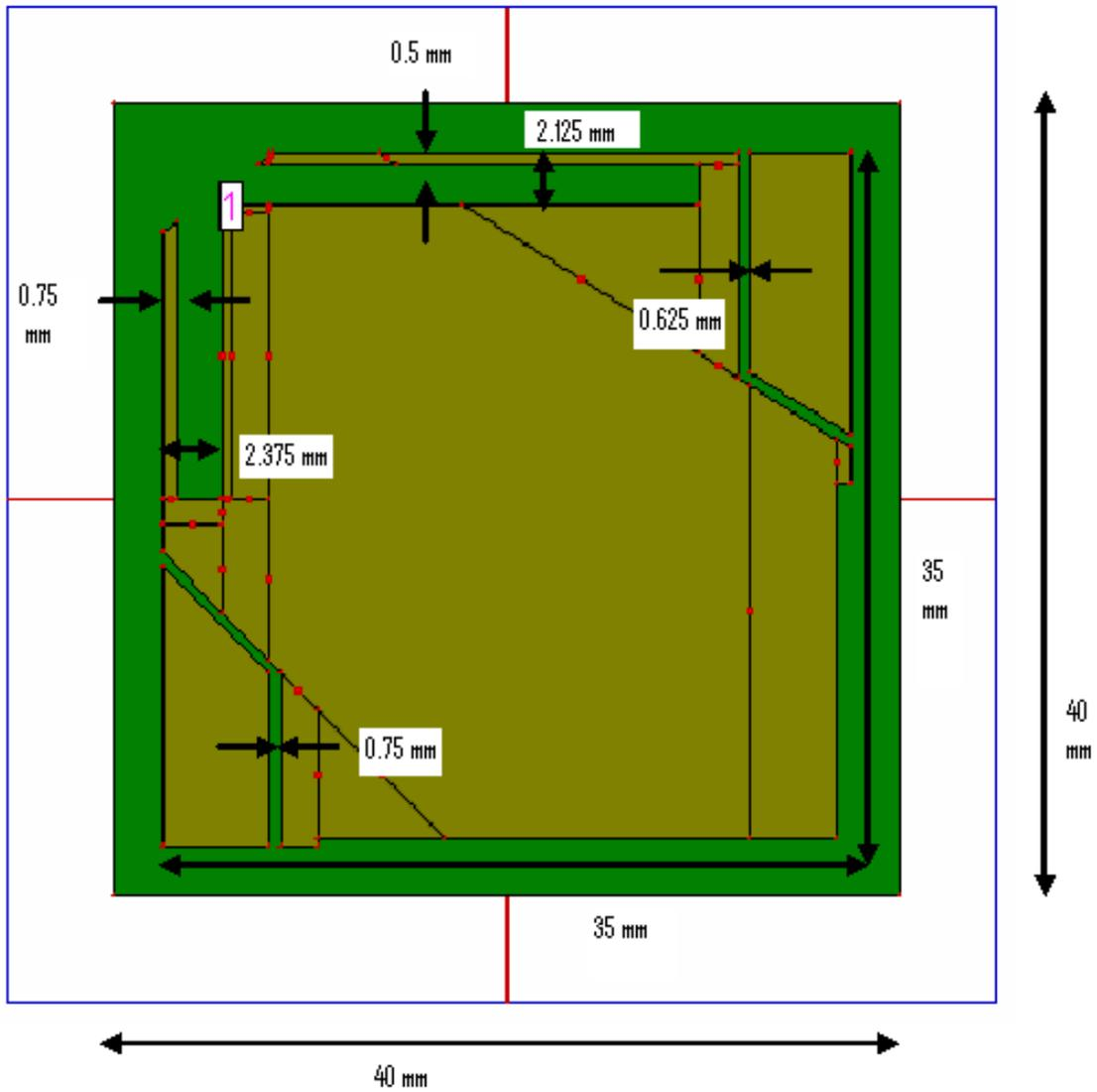
Figure 6.6 Front view of modified square microstrip patch antenna with slits at the edges and having finite ground
