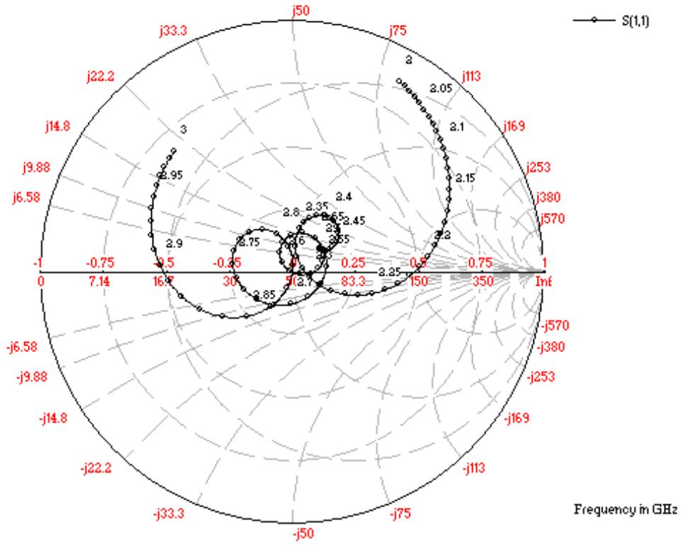
Figure 6.5 Impedance loci for antenna design-1
