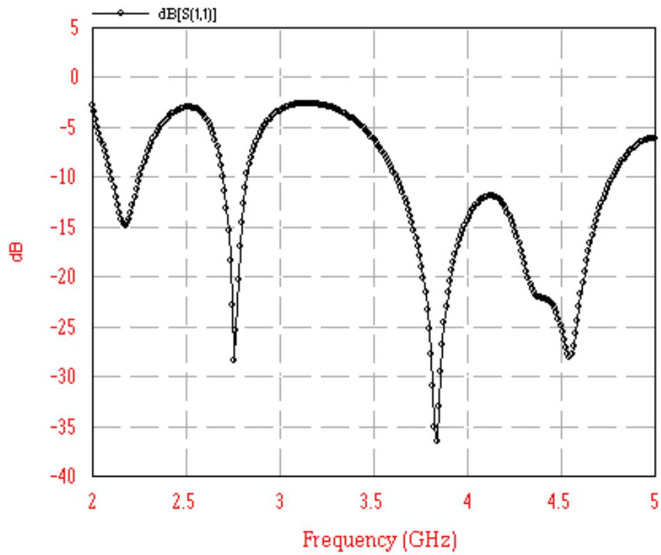
Figure 6.7 Graph between return loss and frequency for antenna design-2
