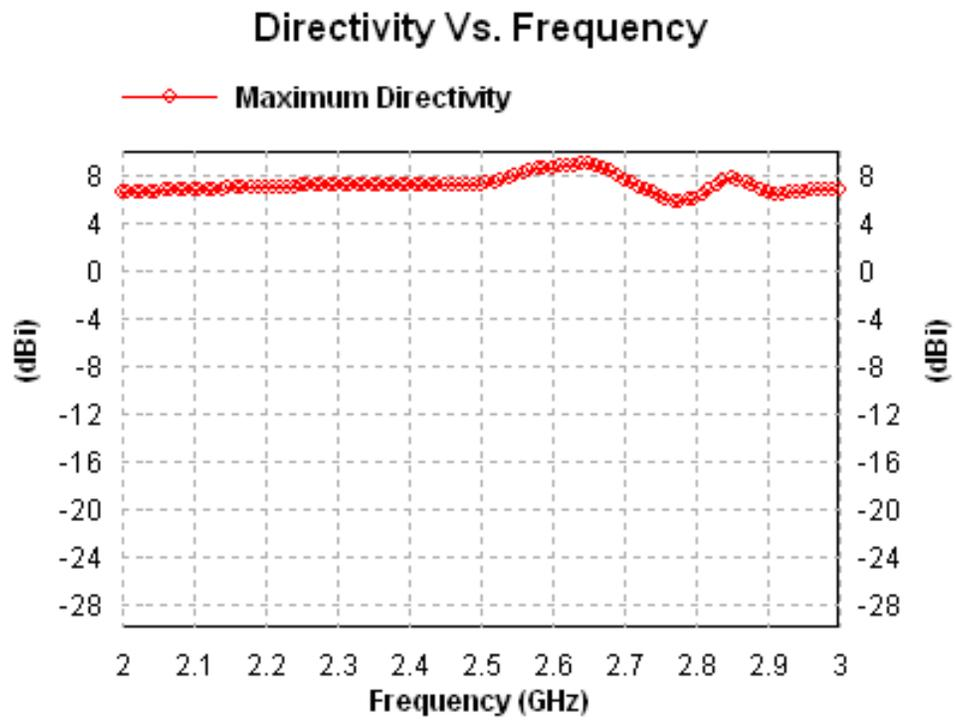
Figure 6.3 Graph between directivity and frequency for antenna design-1
