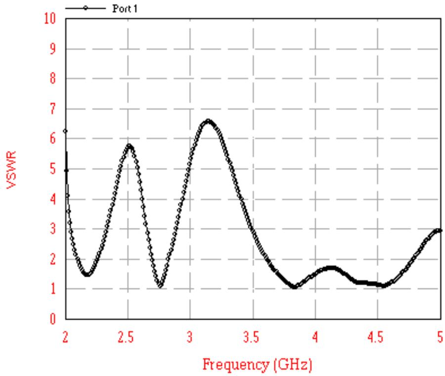
Figure 6.8 Graph between VSWR and frequency for antenna design-2
