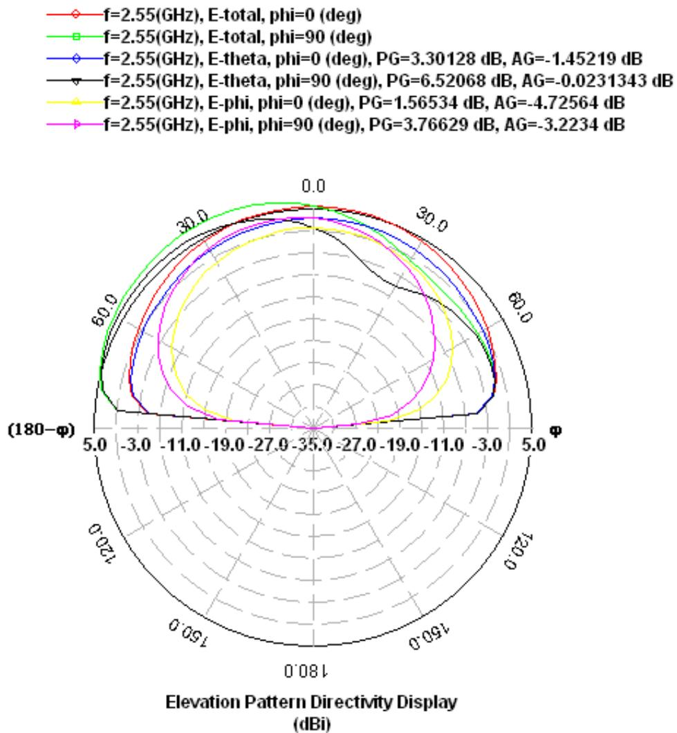
Figure 6.4 Radiation pattern for antenna design-1
