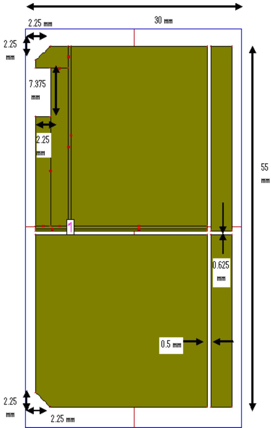
Figure 6.1: Increased substrate height rectangular microstrip antenna design-1
