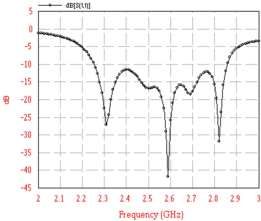
Figure 6.2 Graph between return loss and frequency for antenna design-1
