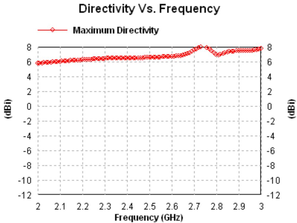
Figure 2.31 Graph between directivity and frequency for antenna design-5
