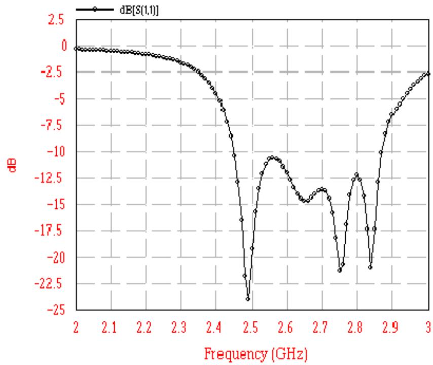
Figure 2.9 Graph between return loss and frequency for antenna design-2
