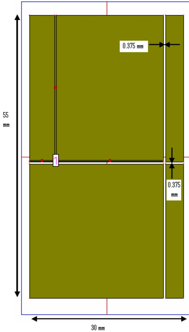
Figure 2.22 Gap-coupled rectangular microstrip antenna design- 4
