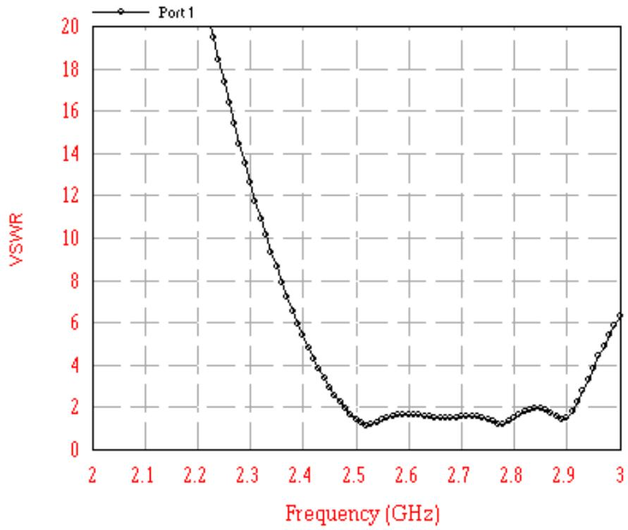
Figure 2.17 Graph between VSWR and frequency for antenna design-3
