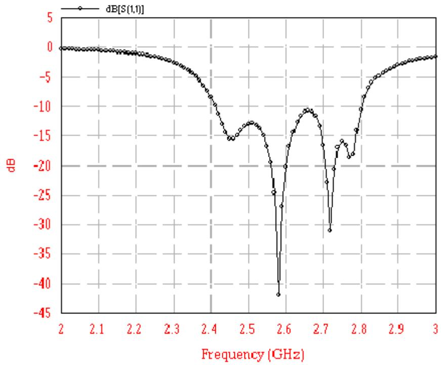
Figure 2.2 Graph between return loss and frequency for antenna design-1
