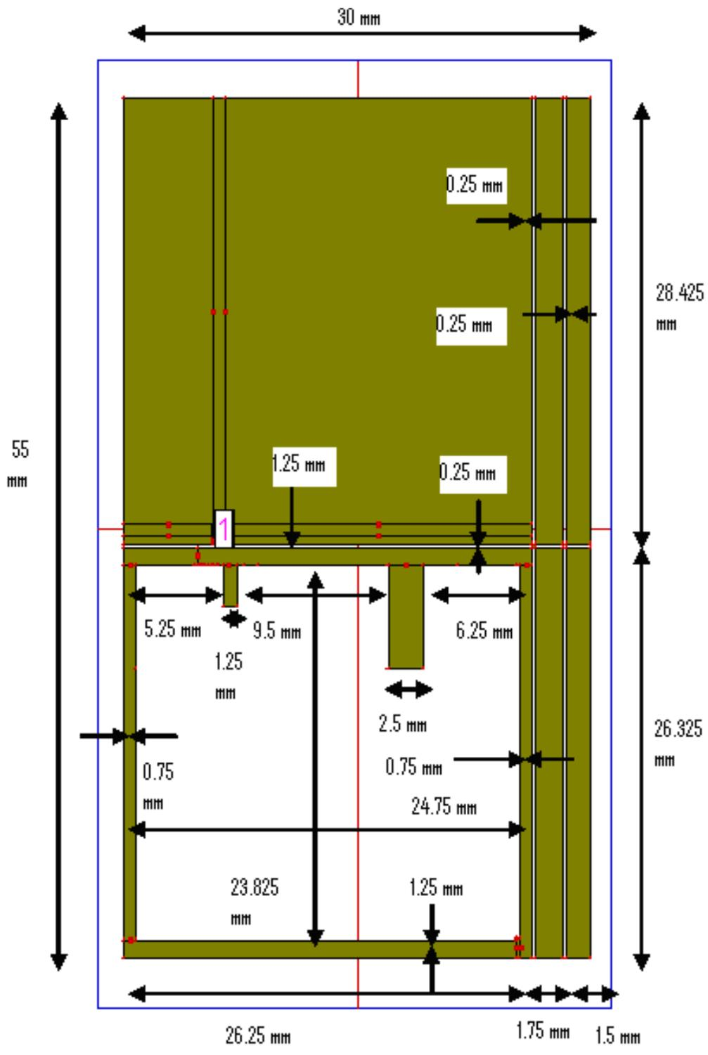
Figure 2.29 Gap-coupled compact rectangular microstrip antenna design-5
