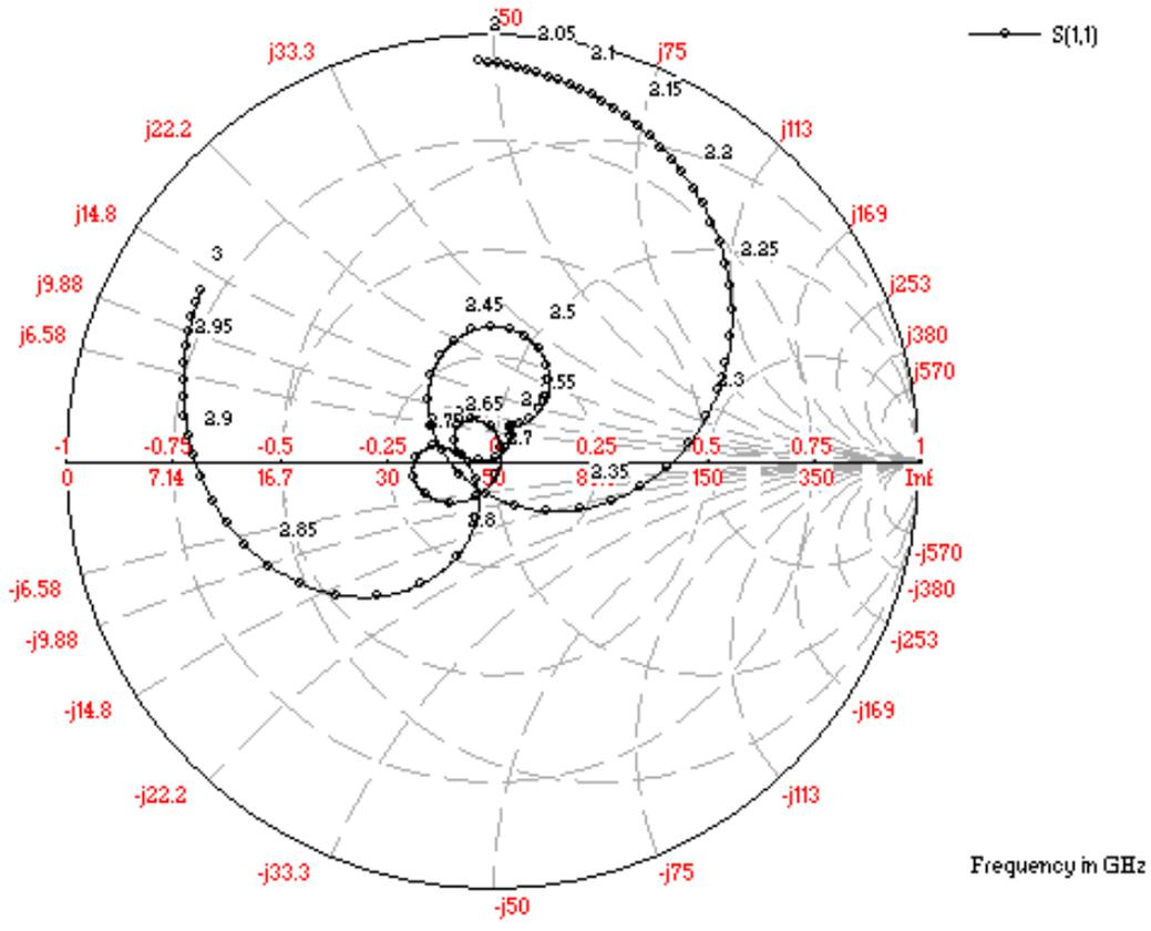
Figure 2.28 Impedance loci for antenna design-4
