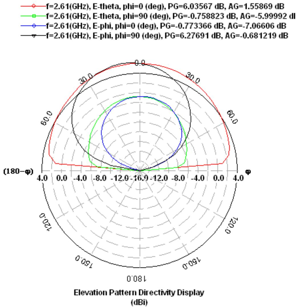
Figure 2.5 Radiation pattern for antenna design-1
