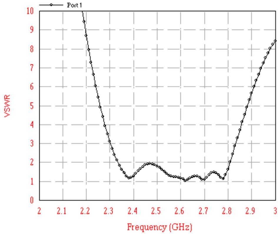
Figure 2.24 Graph between VSWR and frequency for antenna design-4
