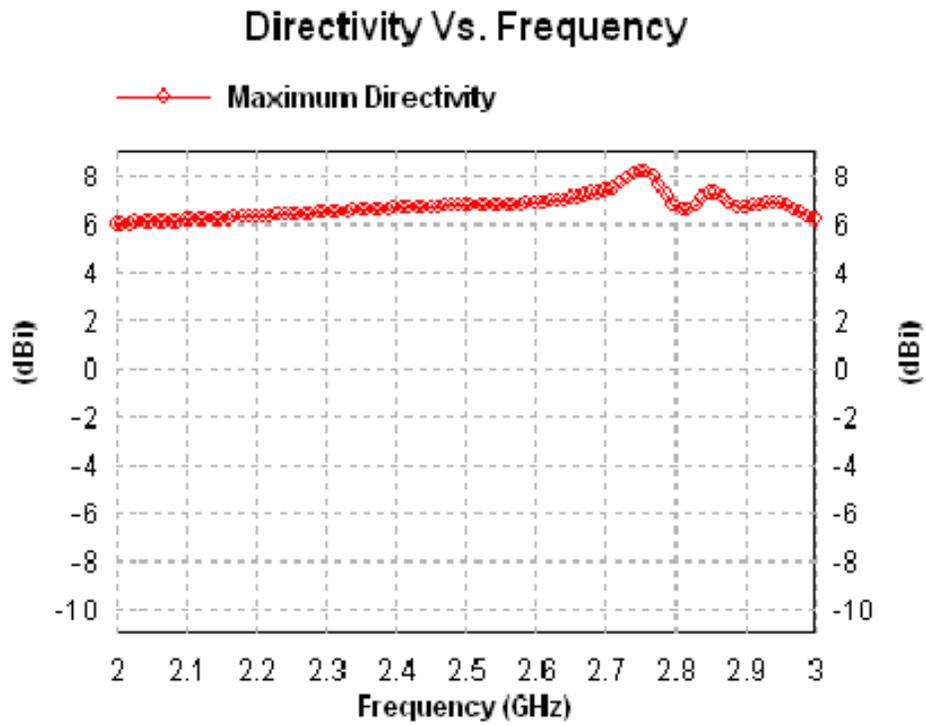
Figure 2.11 Graph between directivity and frequency for antenna design-2
