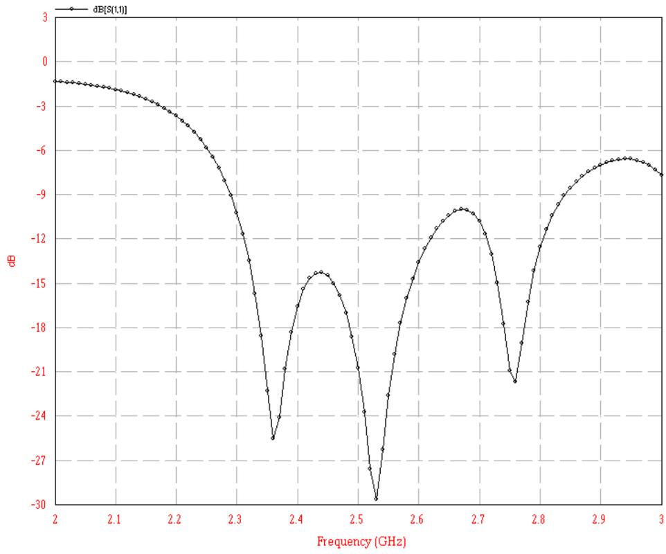
Figure 2.30 Graph between return loss and frequency for antenna design-5
