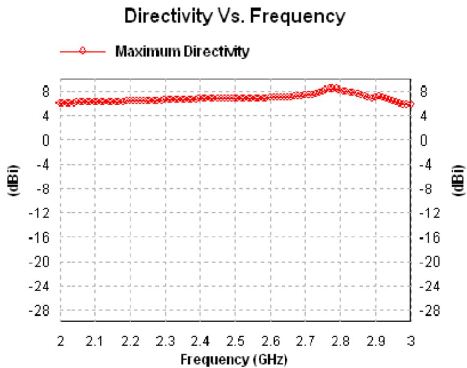
Figure 2.18 Graph between directivity and frequency for antenna design-3
