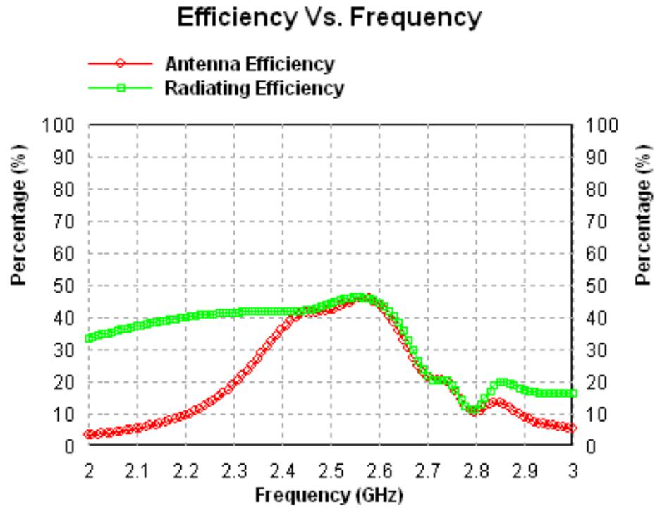
Figure 2.6 Graph between efficiency and frequency for antenna design-1
