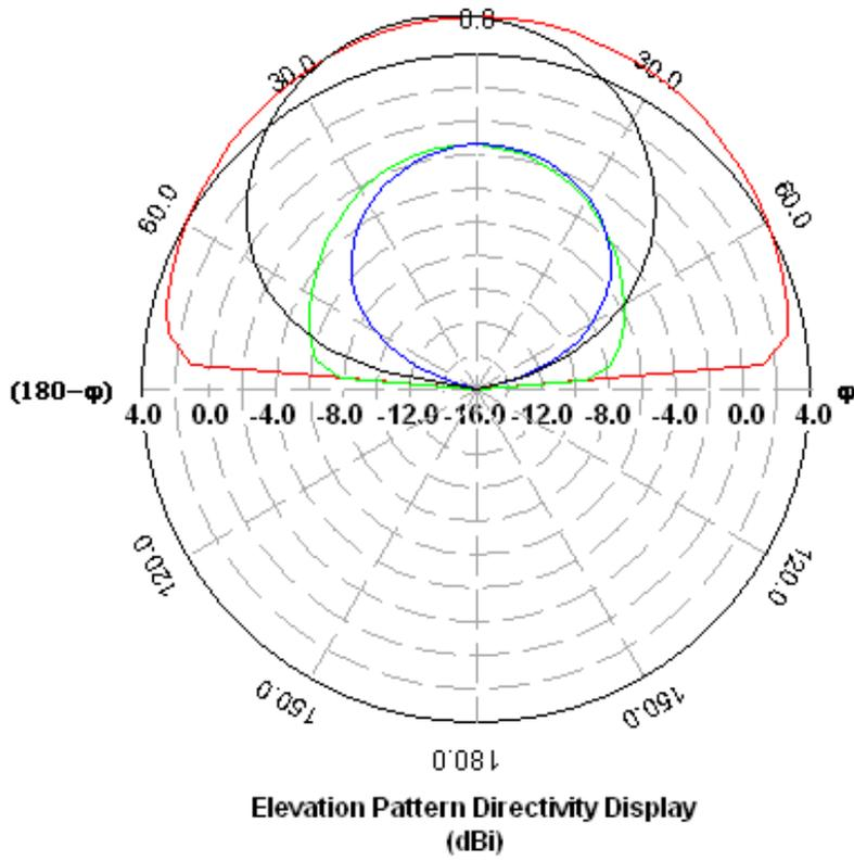
Figure 2.12 Radiation pattern for antenna design-2
