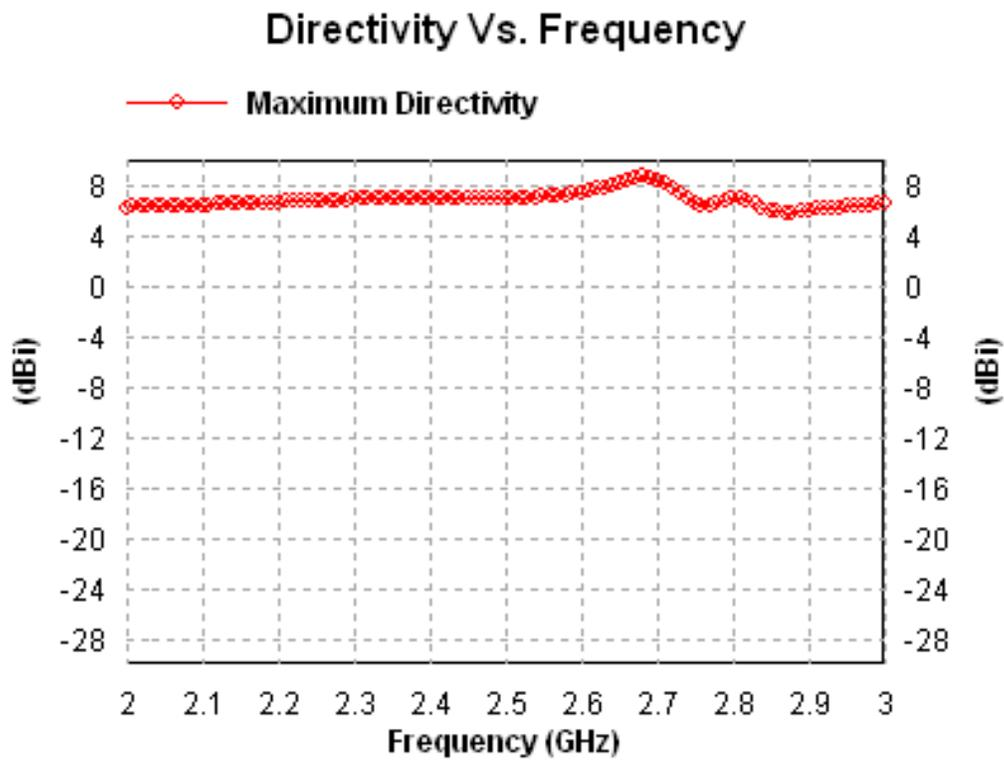
Figure 2.25 Graph between directivity and frequency for antenna design-4
