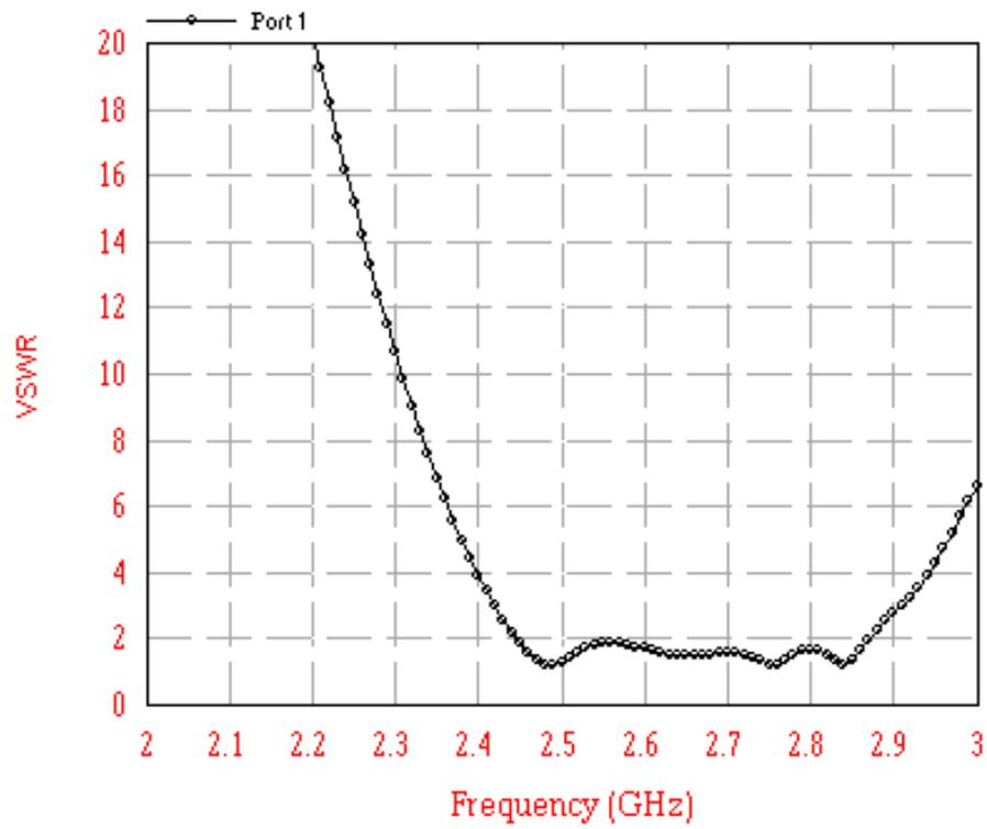
Figure 2.10 Graph between VSWR and frequency for antenna design-2
