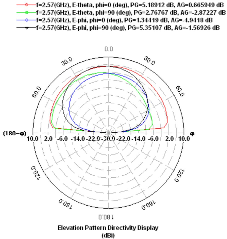
Figure 2.26 Radiation pattern for antenna design-4
