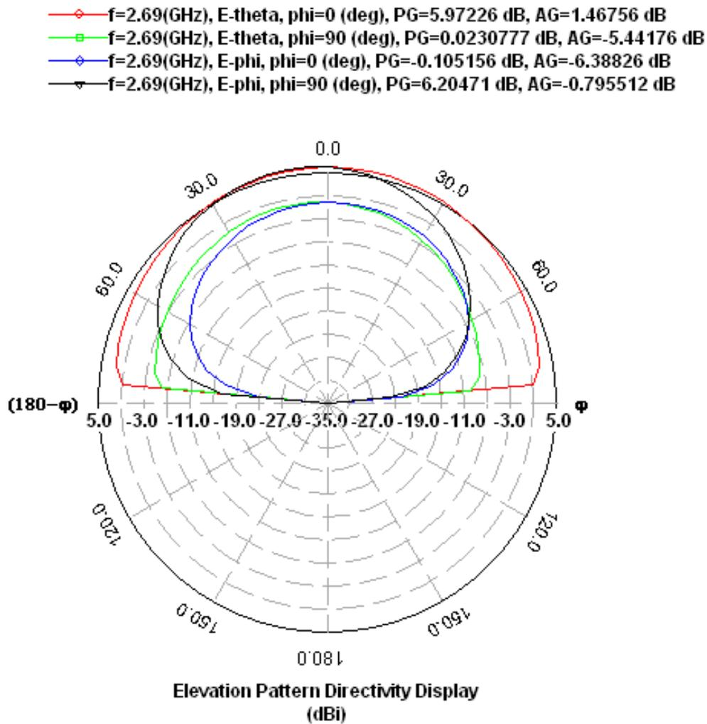
Figure 2.19 Radiation pattern for antenna design-3
