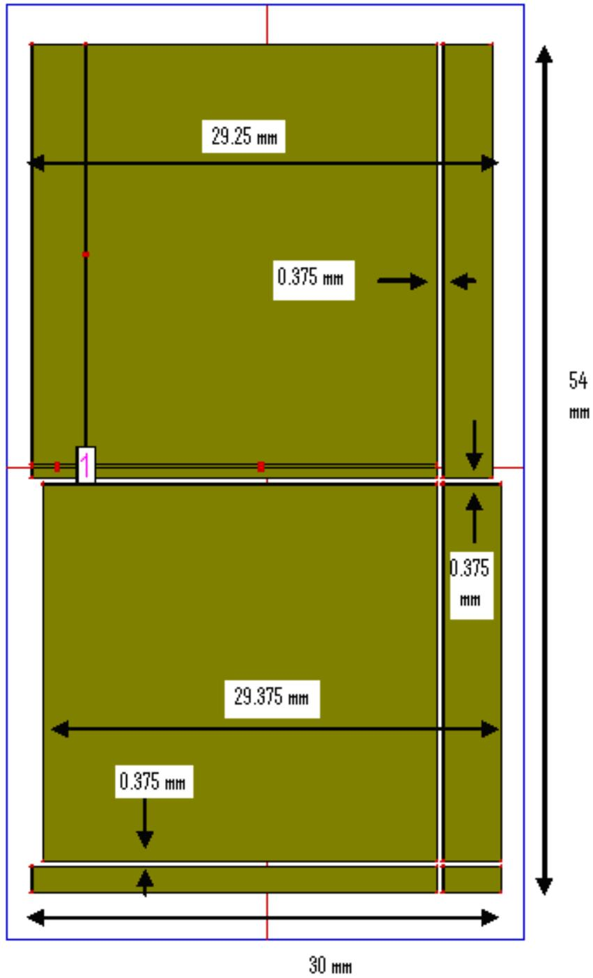
Figure 2.15 Gap-coupled rectangular microstrip antenna design-3
