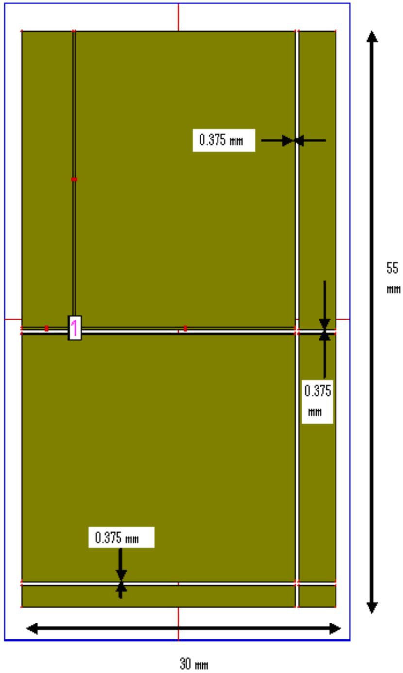
Figure 2.1 Gap-coupled rectangular microstrip antenna design-1
