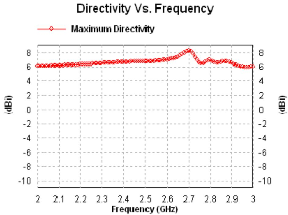
Figure 2.4 Graph between directivity and frequency for antenna design-1
