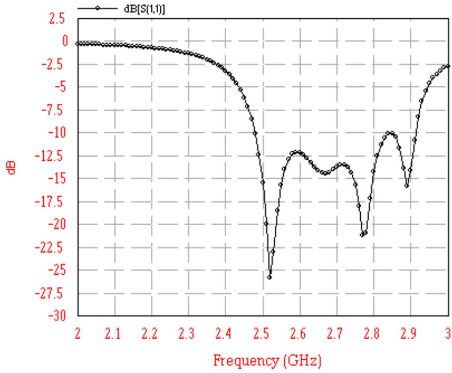
Figure 2.16 Graph between return loss and frequency for antenna design-3
