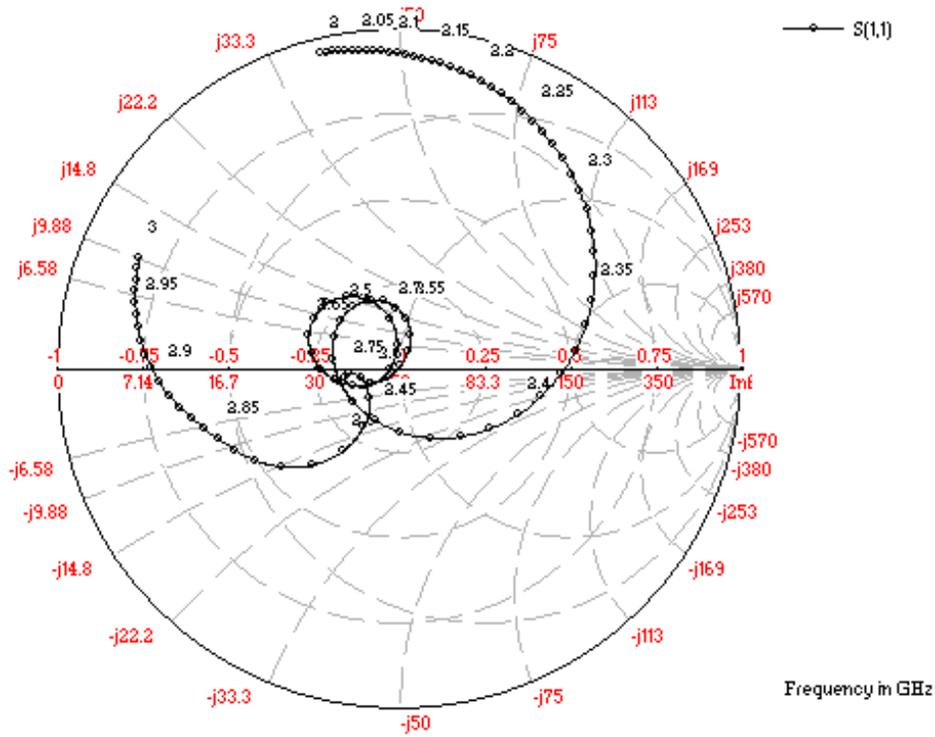
Figure 2.7 Impedance loci for antenna design-1
