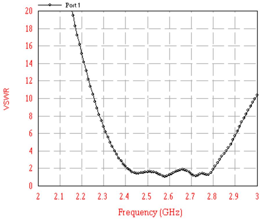
Figure 2.3 Graph between VSWR and frequency for antenna design-1
