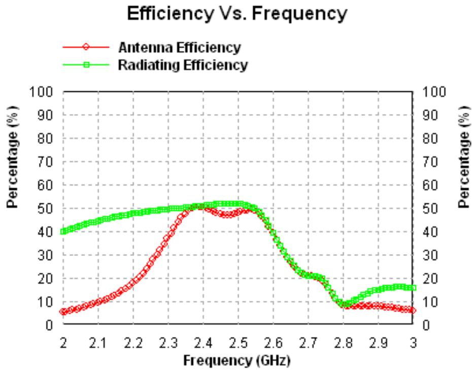
Figure 2.27 Graph between efficiency and frequency for antenna design-4
