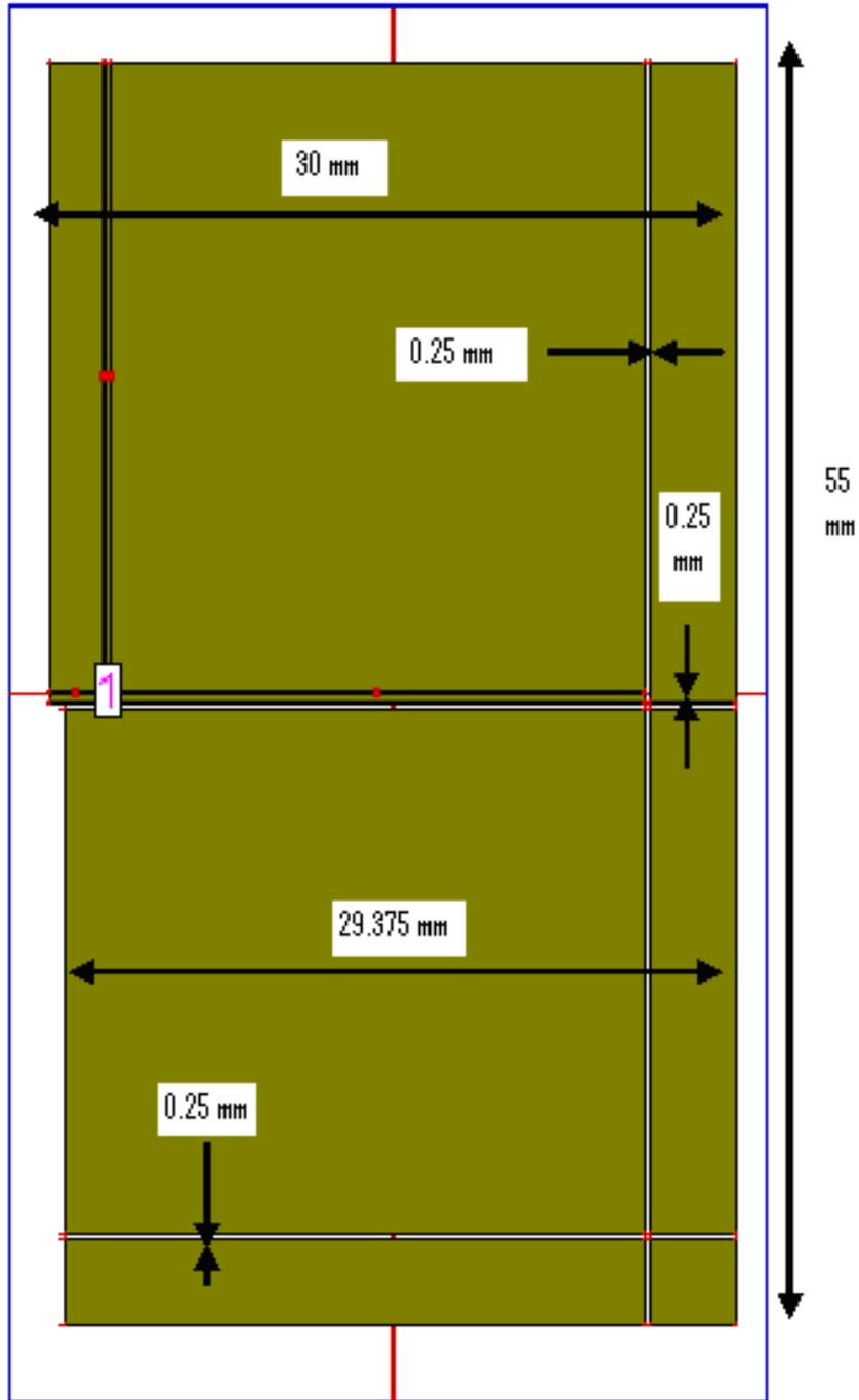
Figure 2.8 Gap-coupled rectangular microstrip antenna design-2
