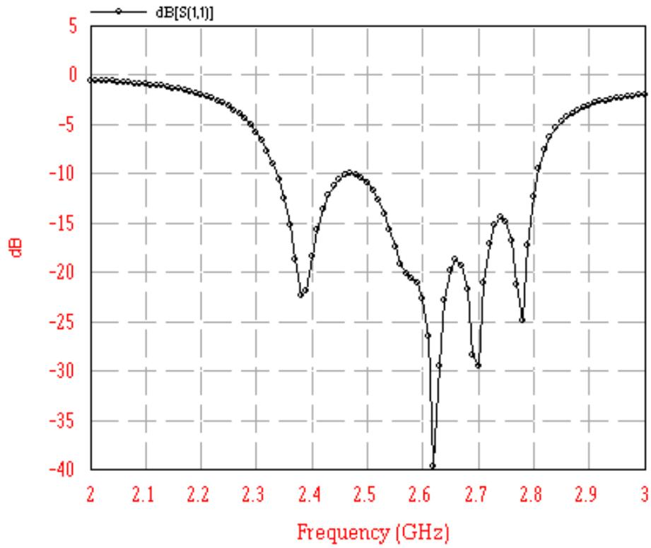
Figure 2.23 Graph between return loss and frequency for antenna design-4
