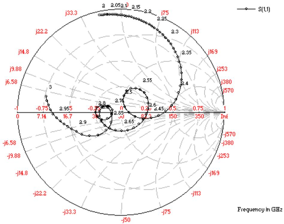
Figure 2.14 Impedance loci for antenna design-2
