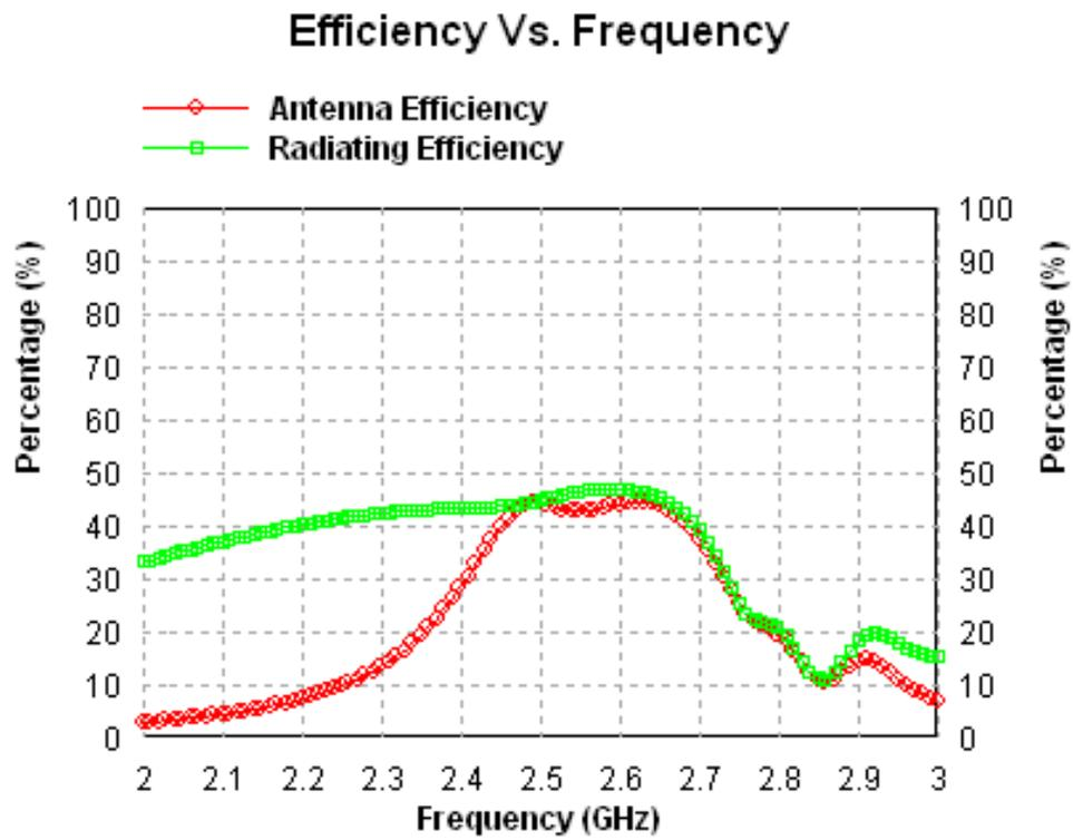
Figure 2.13 Graph between efficiency and frequency for antenna design-2
