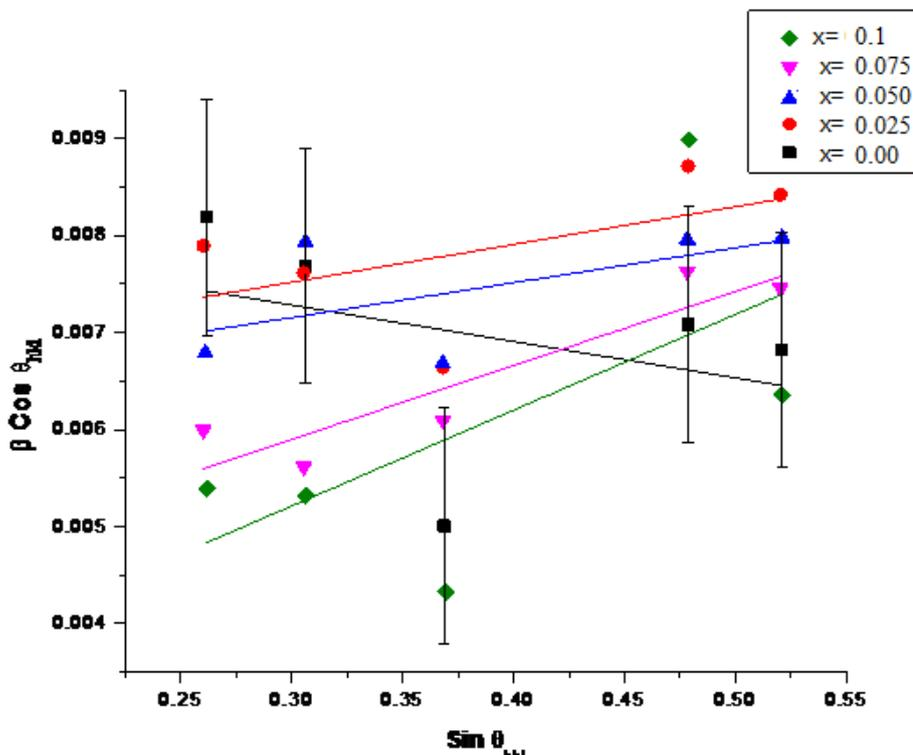
**Fig. 3.3: Williamson-Hall plot of as-prepared and annealed  $\text{CoFe}_2\text{O}_4:\text{SiO}_2$  nanocomposites at different temperatures**
