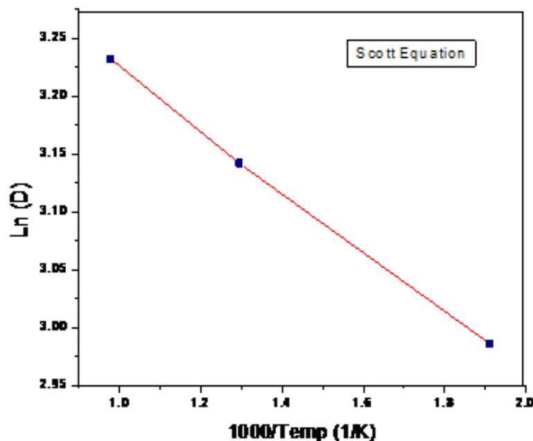
**Fig. 3.4: Crystallite size versus calcinations temperatures (Scott equation)**
