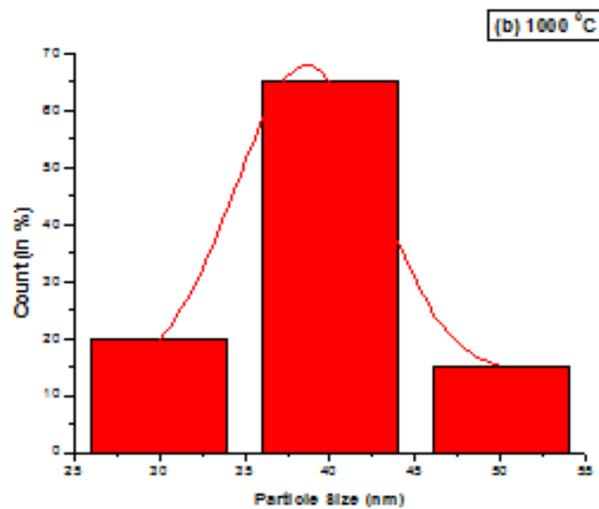
**Fig. 3.8: (b) Histogram of  $\text{CoFe}_2\text{O}_4:\text{SiO}_2$  nanocomposites annealed at  $1000^\circ\text{C}$**
