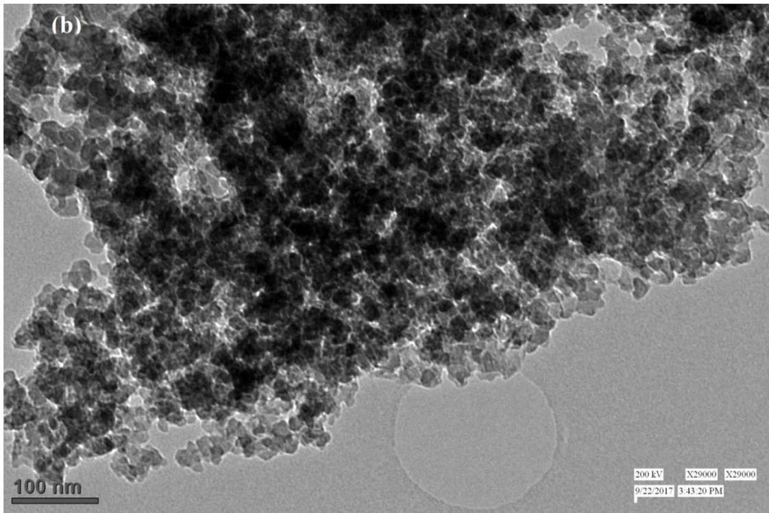
**Fig. 3.7: (b) TEM micrograph of  $\text{CoFe}_2\text{O}_4:\text{SiO}_2$  nanocomposites annealed at  $1000^\circ\text{C}$**
