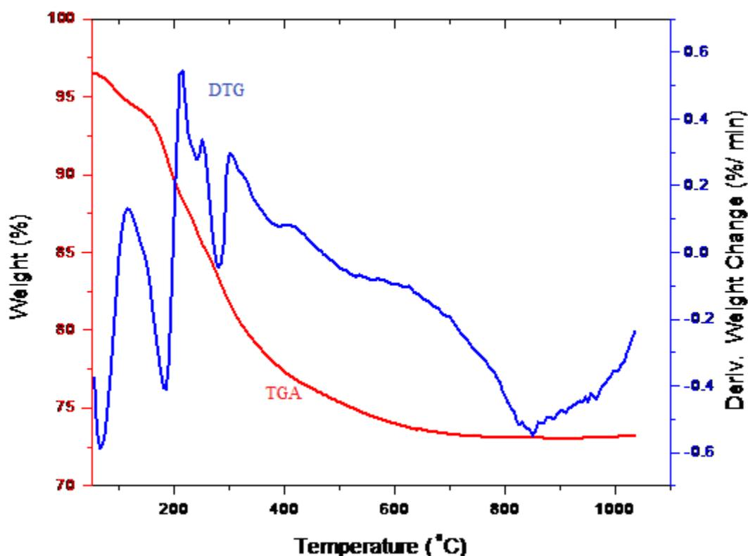
**Fig. 3.9:** TGA-DTG curve of  $\text{CoFe}_2\text{O}_4:\text{SiO}_2$  nanocomposites
