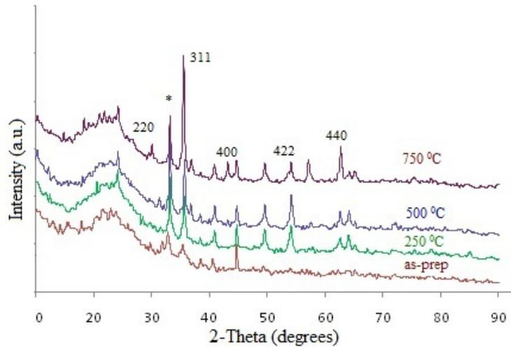
**Fig. 3.1: XRD patterns of as-prepared and thermally treated samples of  $\text{CoFe}_2\text{O}_4:\text{SiO}_2$  nanocomposites**
