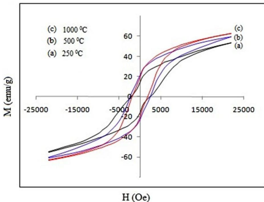
**Fig. 3.10: Hysteresis loop of  $\text{CoFe}_2\text{O}_4:\text{SiO}_2$  nanocomposites annealed at different temperatures**
