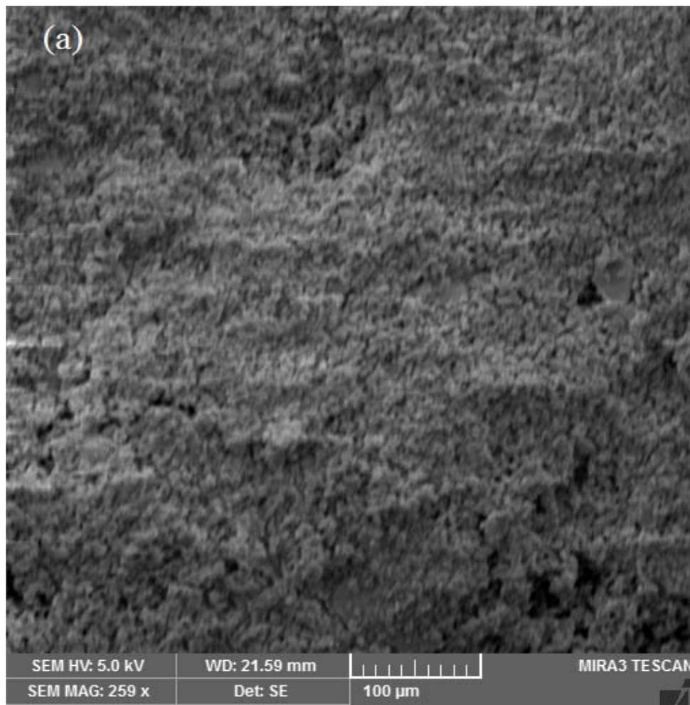
**Fig. 3.6: (a) SEM micrograph of  $\text{CoFe}_2\text{O}_4:\text{SiO}_2$  nanocomposites at  $250^\circ\text{C}$**
