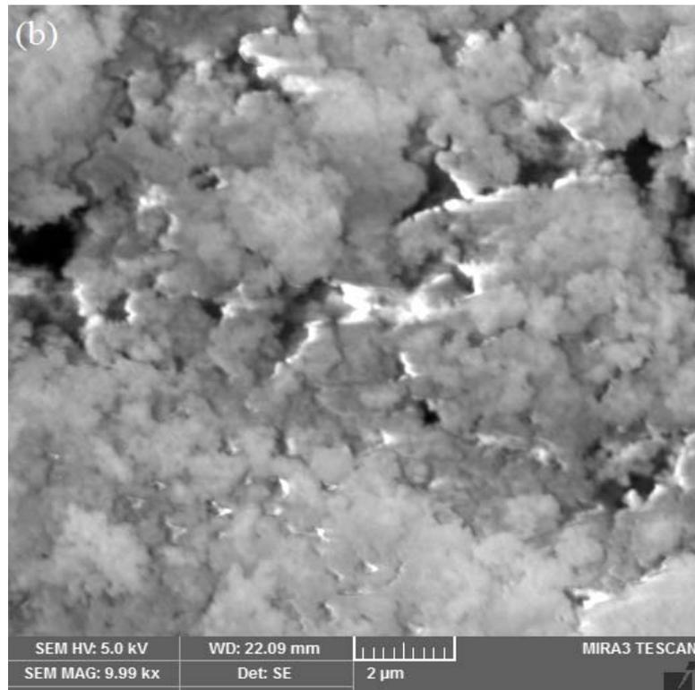
**Fig. 3.6: (b) SEM micrograph of  $\text{CoFe}_2\text{O}_4:\text{SiO}_2$  nanocomposites at 500 °C**
