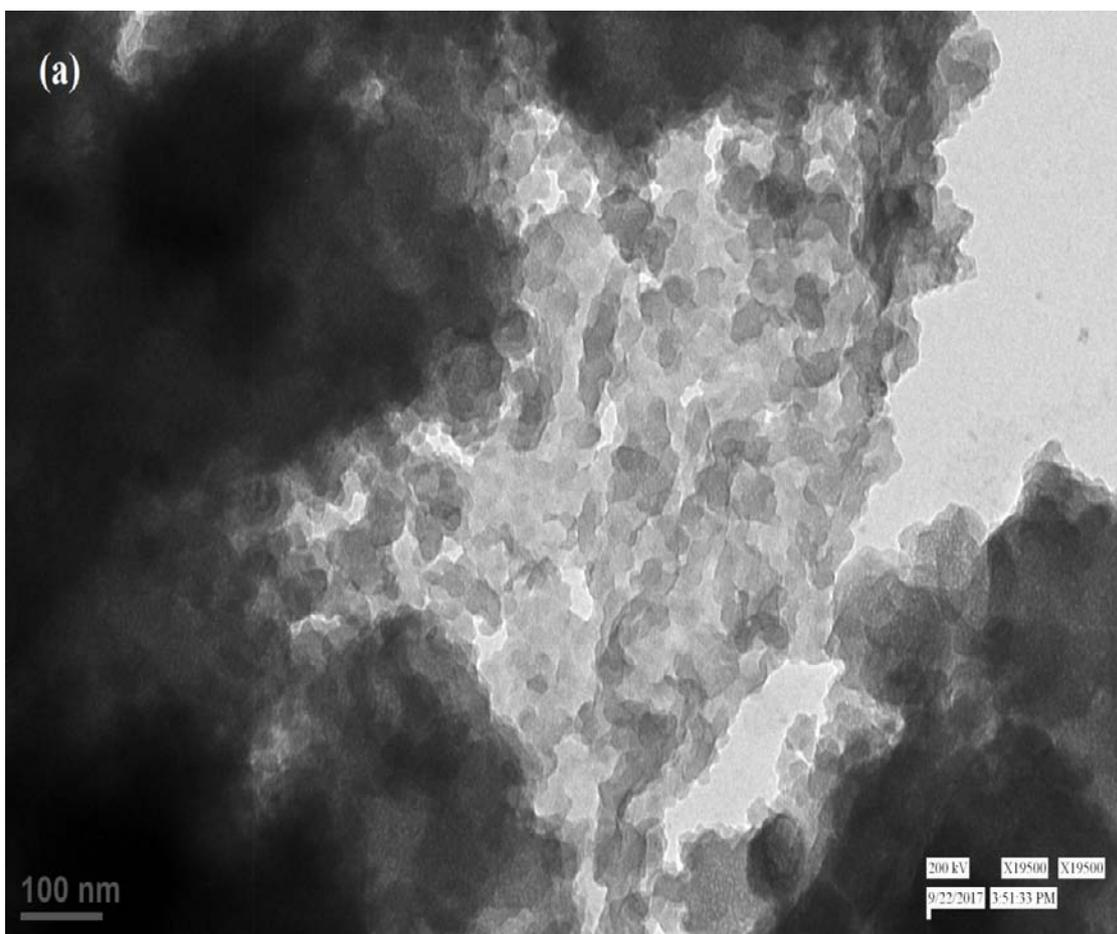
**Fig. 3.7:** (a) TEM micrograph of  $\text{CoFe}_2\text{O}_4:\text{SiO}_2$  nanocomposites annealed at  $750^\circ\text{C}$
