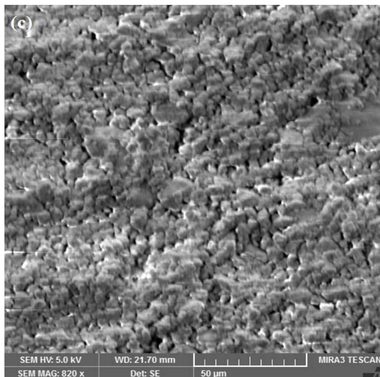
**Fig. 3.6: (c) SEM micrograph of  $\text{CoFe}_2\text{O}_4:\text{SiO}_2$  nanocomposites at 750 °C**
