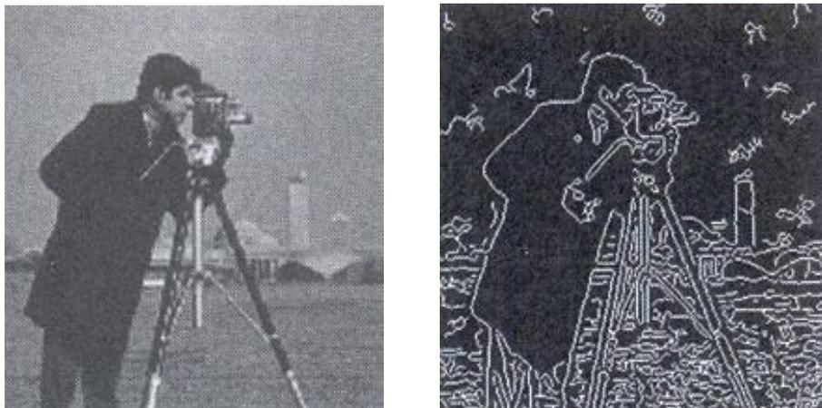
**Figure 5.2** Edge detected image displayed in a GLV display
