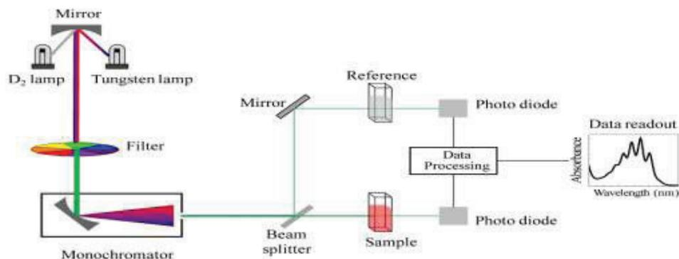
**Figure 1.6 Schematic diagram of UV-visible double beam spectrophotometer**
