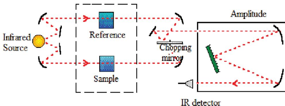
**Figure 1.2 Schematic diagram of dispersive infrared spectrophotometer**
