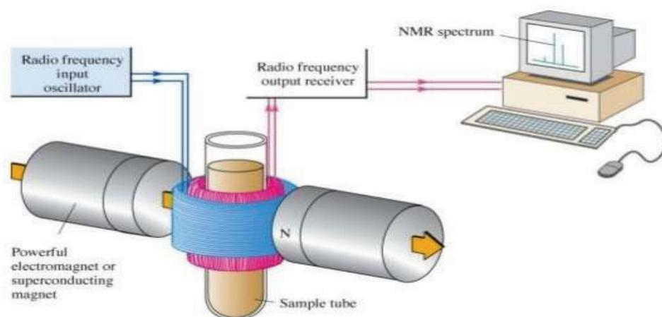
**Figure 1.7 Schematic diagram of nuclear magnetic resonance spectrophotometer**
