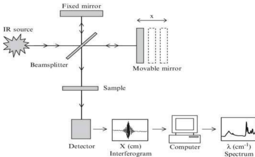
**Figure 1.3 Schematic diagram of Fourier Transform Infrared Spectrophotometer**
