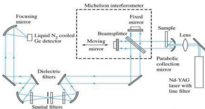
**Figure 1.5 The block diagram of FT -Raman Spectrophotometer**
