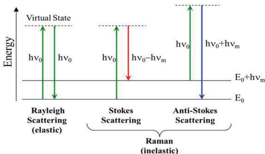
Figure 1.4 Rayleigh, Stoke's and anti stoke's scattering energy levels
