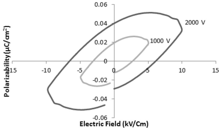
**Fig. 4.2** Ferroelectric hysteresis loop study
