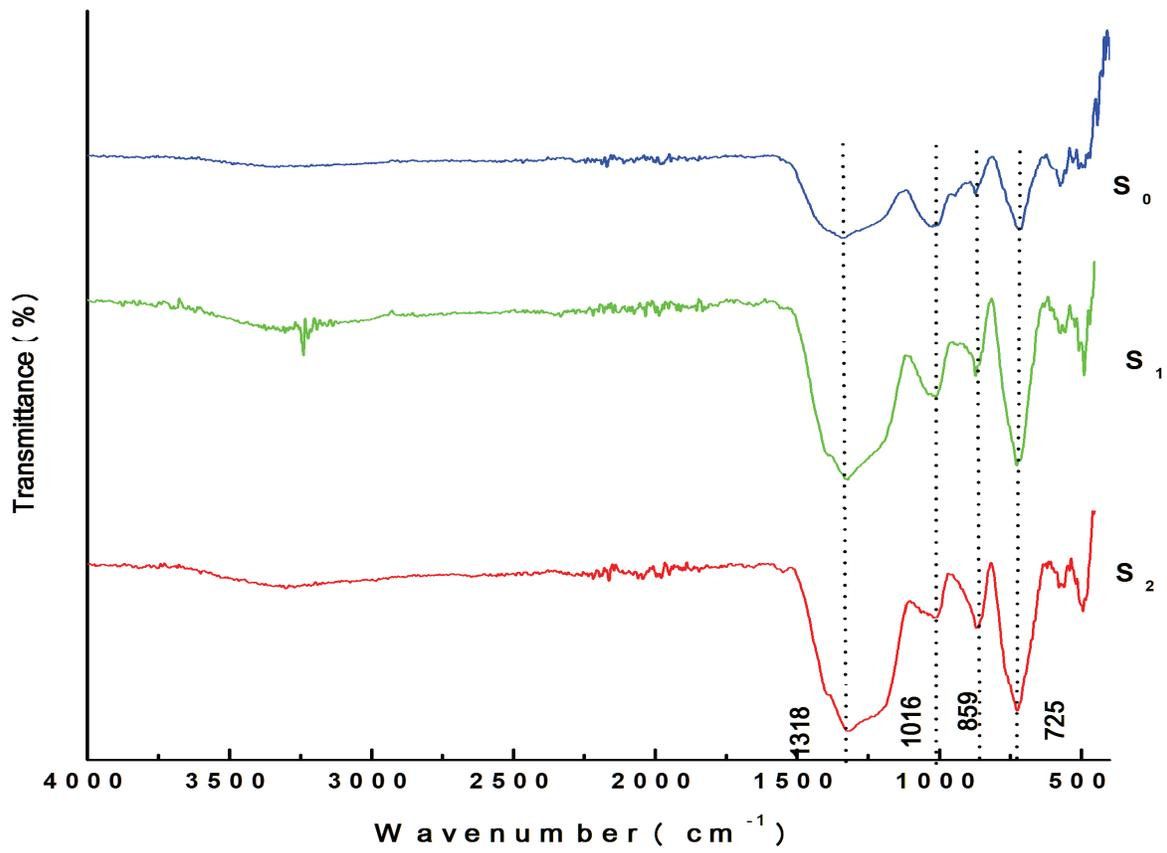
Fig. 5.2.1. FT-IR Spectra of Pure NCPB glass (S<sub>0</sub>) and 0.05 to 0.1 CuO doped NCPBC glasses (S<sub>1</sub> – S<sub>2</sub>)
