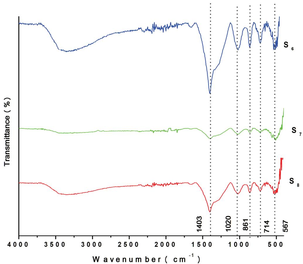
Fig. 5.2.3. FT-IR Spectra of 0.3 to 0.4 CuO doped NCPBC glasses (S<sub>6</sub> – S<sub>8</sub>)
