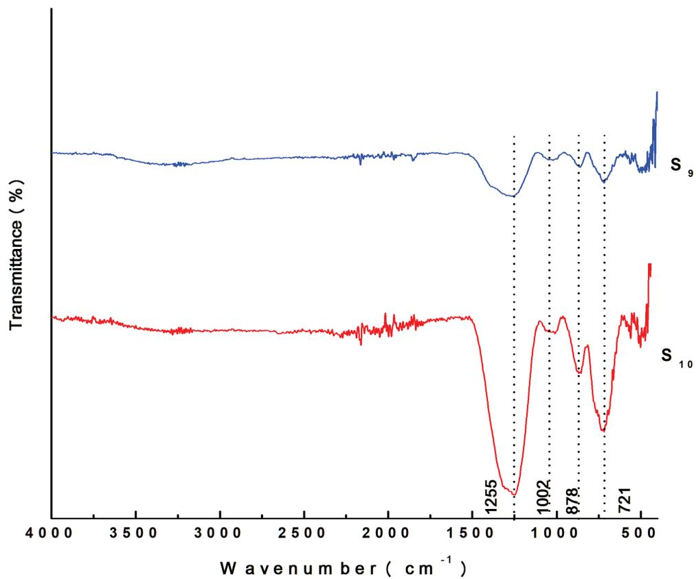
Fig. 5.2.4. FT-IR Spectra of 0.45 to 0.5 CuO doped NCPBC glasses (S<sub>9</sub> – S<sub>10</sub>)
