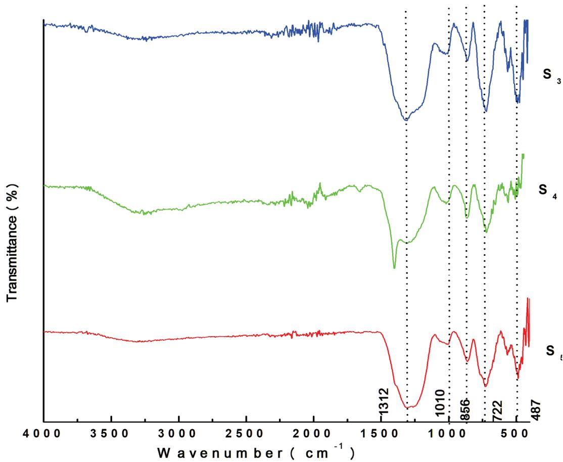
Fig. 5.2.2. FT-IR Spectra of 0.15 to 0.25 CuO doped NCPBC glasses (S<sub>3</sub> – S<sub>5</sub>)
