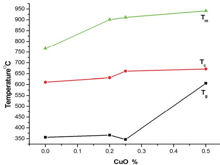
Fig. 5.1.5. Compositional dependency of glass transition, crystallization and melting temperature
