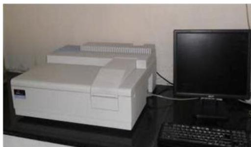
**Figure 2.5 UV-Vis double beam spectrometer**
