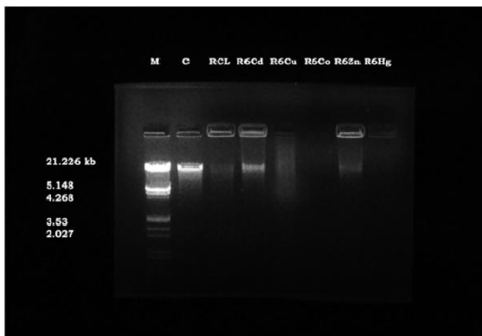
Fig. 6(2) DNA cleavage of Schiff base [BCACP] and their Cu(II), Co(II), Zn(II), Cd(II) and Hg(II) complexes
