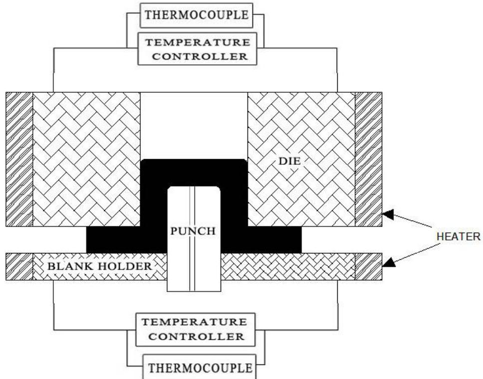
**Figure 4.2 Schematic diagram of the die arrangement**
