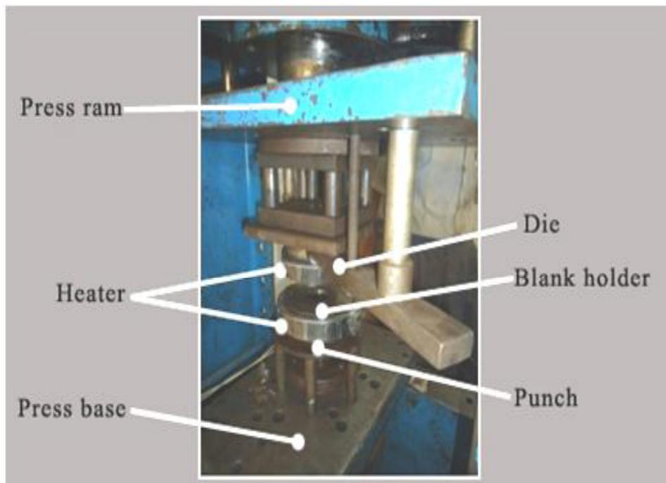
**Figure 4.3 Close up view of the Tooling set-up**
