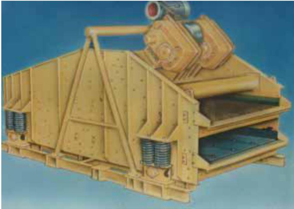
**Figure 1.1 Vibrating Screen Equipment**
