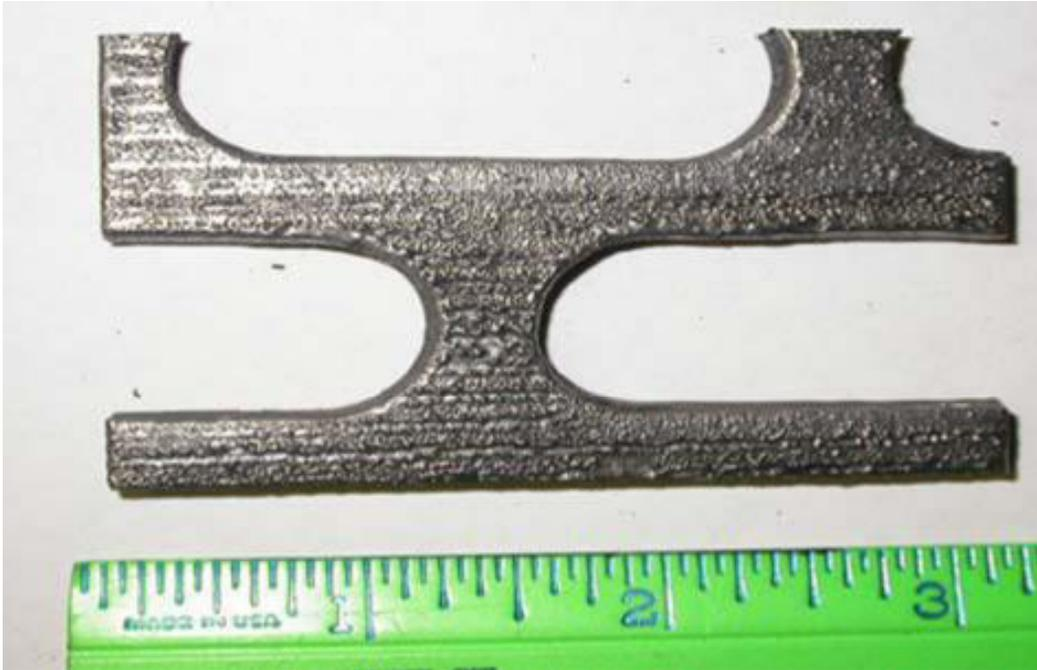
**Figure 1.2 Screen Section Made of En 19 Steel (Tao et al (2007))**
