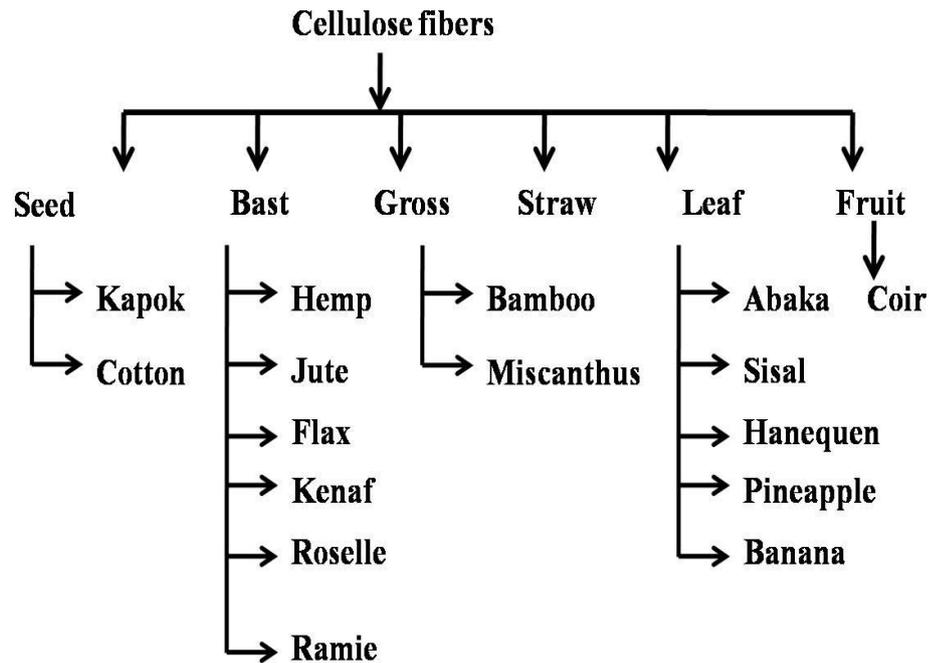
**Figure 1.5 Classifications of cellulose fibers**
