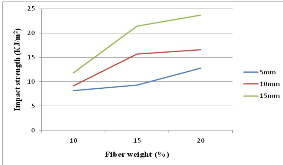
**Figure 4.3 Graphical illustrations of impact strength properties of treated sisal/unsaturated polyester composites**
