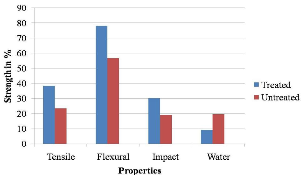
**Figure 4.4 Comparisons of mechanical and moisture absorption properties of treated/untreated hybrid composites**
