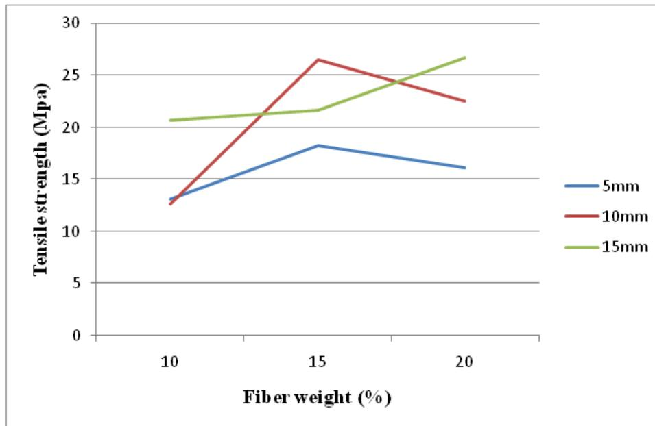
**Figure 4.1 Graphical illustrations of tensile properties of treated sisal/unsaturated polyester composites**
