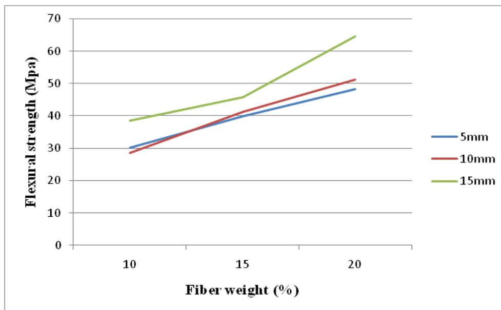
**Figure 4.2 Graphical illustrations of flexural properties of treated sisal/unsaturated polyester composites**
