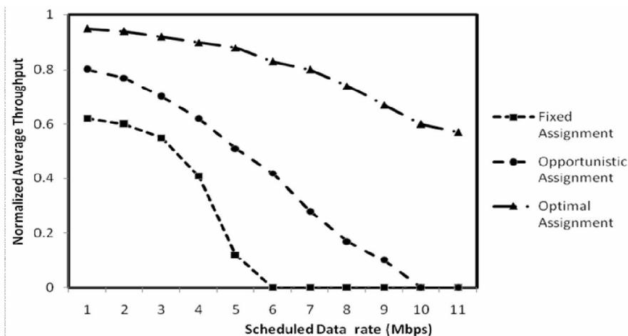
**Figure 4.2 Normalized Average Throughput Versus Scheduled Data Rate with CSIT Error Variance = 0.05**
