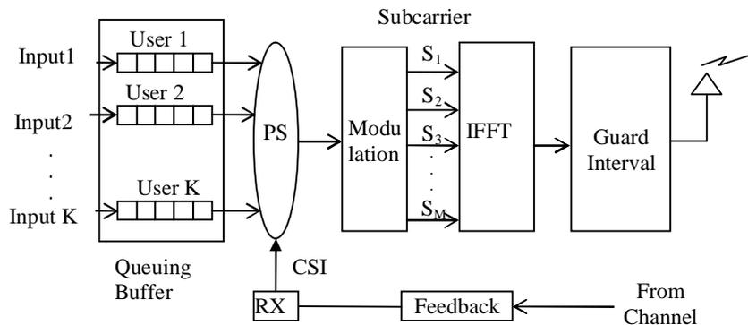
**Figure 4.1 General Cross-Layer Scheduling Model of OFDM Based Multiuser Wireless System**
