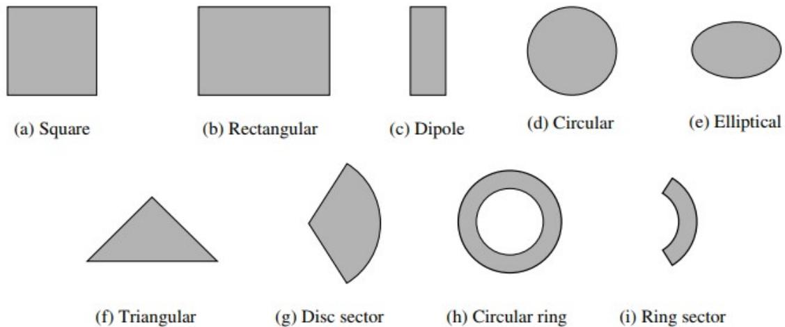
**Figure 3.2** Different shapes of micro-strip patch elements (Balanis C. A. (2005))
