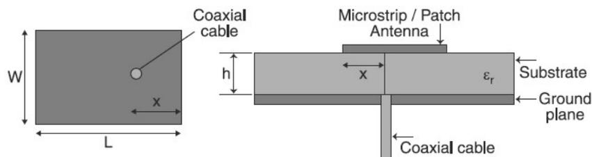
**Figure 3.5** Coaxial feed MSA (John D Kraus et al. (2015))
