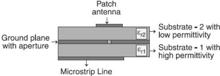
**Figure 3.6** Aperture coupled feed MSA (John D Kraus et al. (2015))
