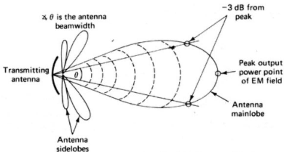
Figure 3.9 Radiation pattern of antenna
