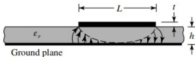
Figure 3.1(b) Micro-strip patch antenna side view (Balanis C. A. (2005))
