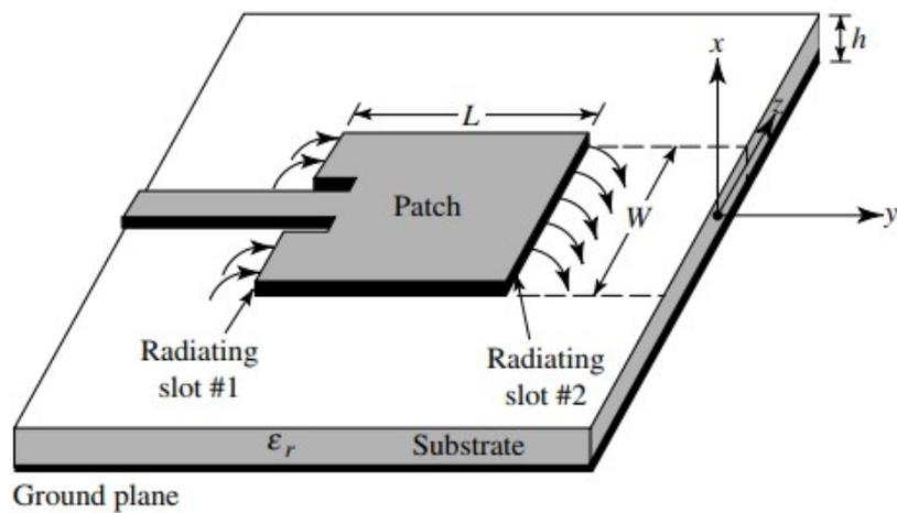
Figure 3.1(a) Micro-strip patch antenna top view (Balanis C. A. (2005))
