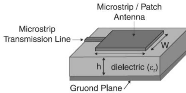
**Figure 3.3** Micro-strip line feed MSA (John D Kraus et al. (2015))
