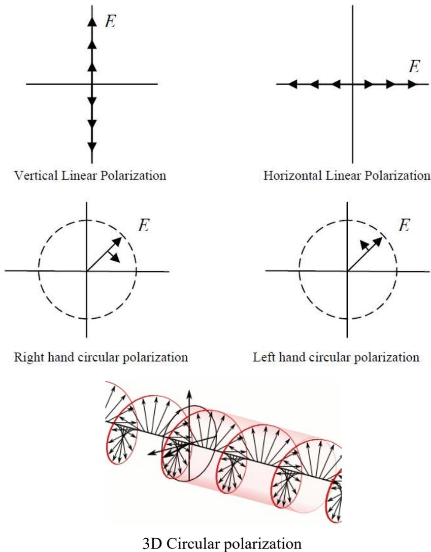
**Figure 3.10** Linear and circular polarizations of an antenna
